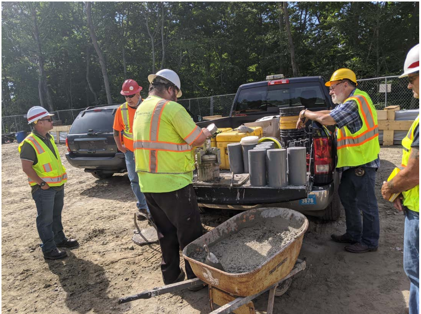
Picture 8: JTC testing the concrete being placed, Shared Access Driveway. View to the east.
