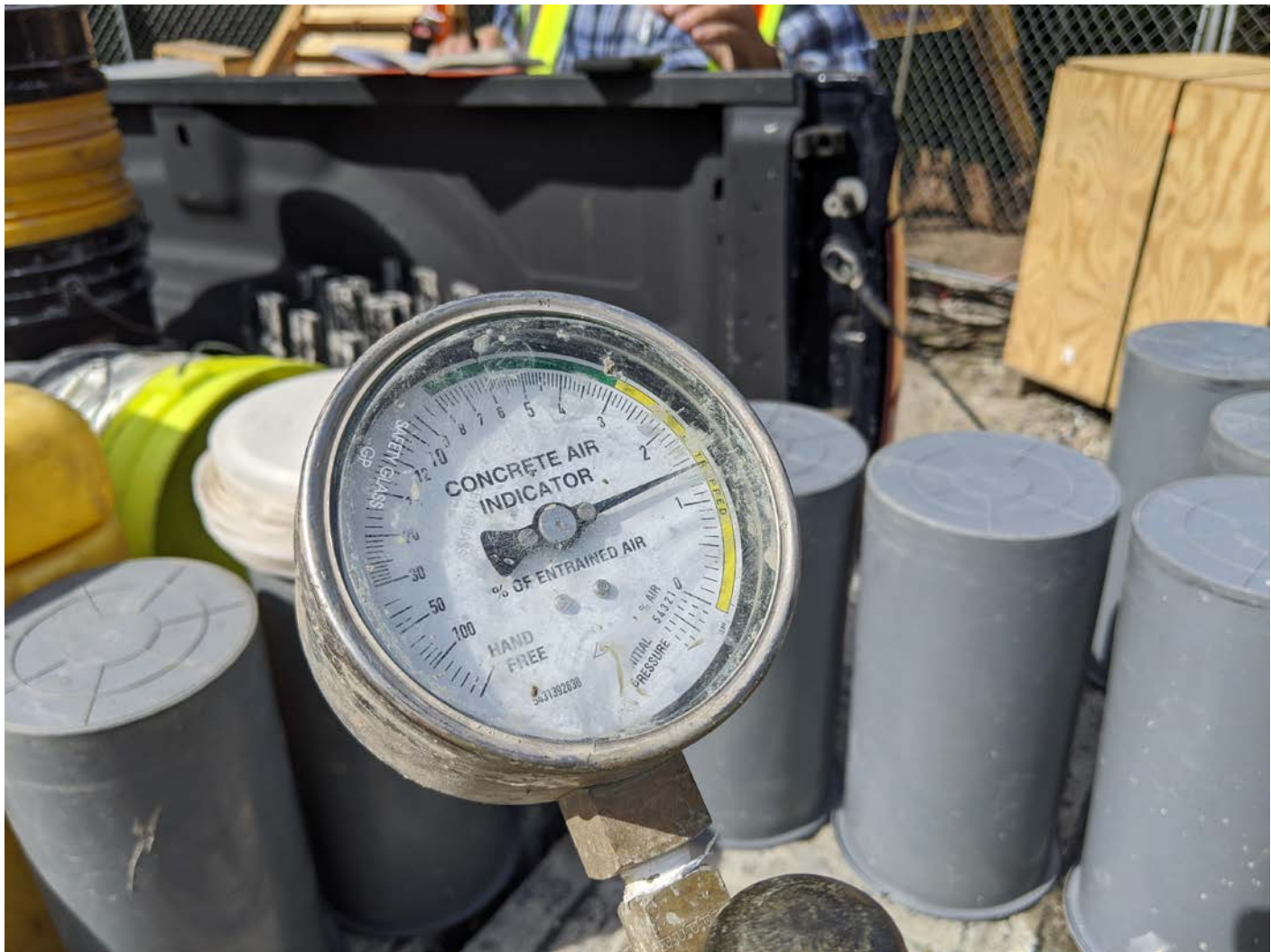
Picture 9: Concrete air entrainment indicator reading 1.4, Water Tank, Shared access driveway.
