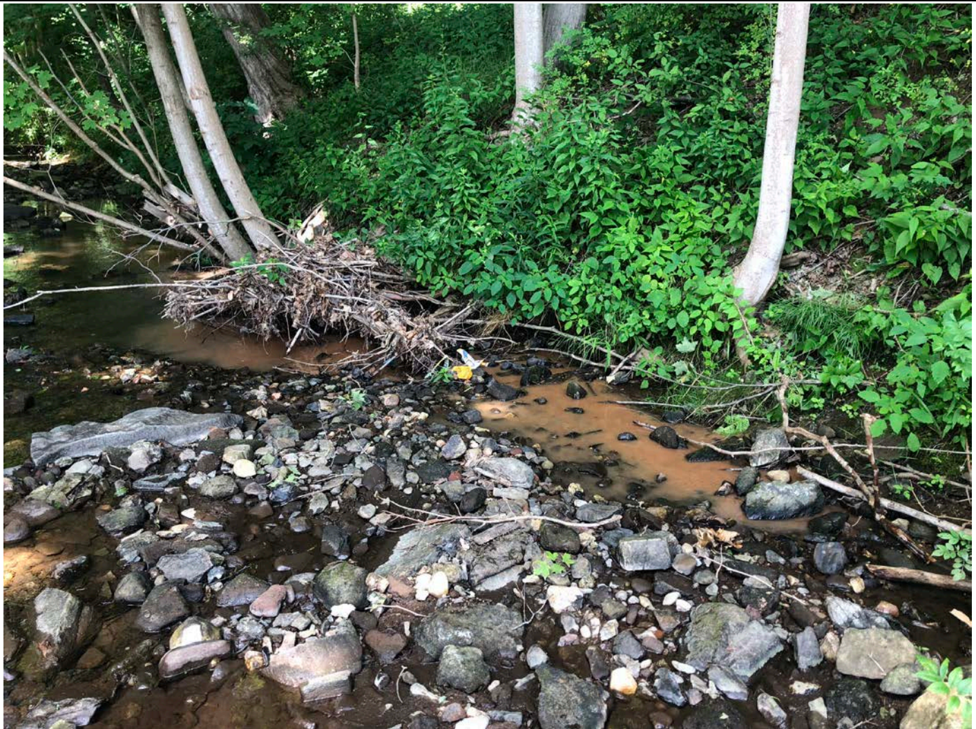
Picture 5: Turbidity from water draining off the filter bed closest to the stream bank on Hersig Brook. View is to the northwest. Pickett Lane, Durham. Station ~532+00.
