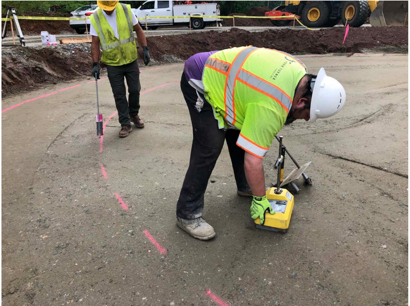
Picture 8: JTC collecting soil compaction data at elevation 437 at the water tank footprint. Shared Access Driveway, Middletown. View to the southeast.
