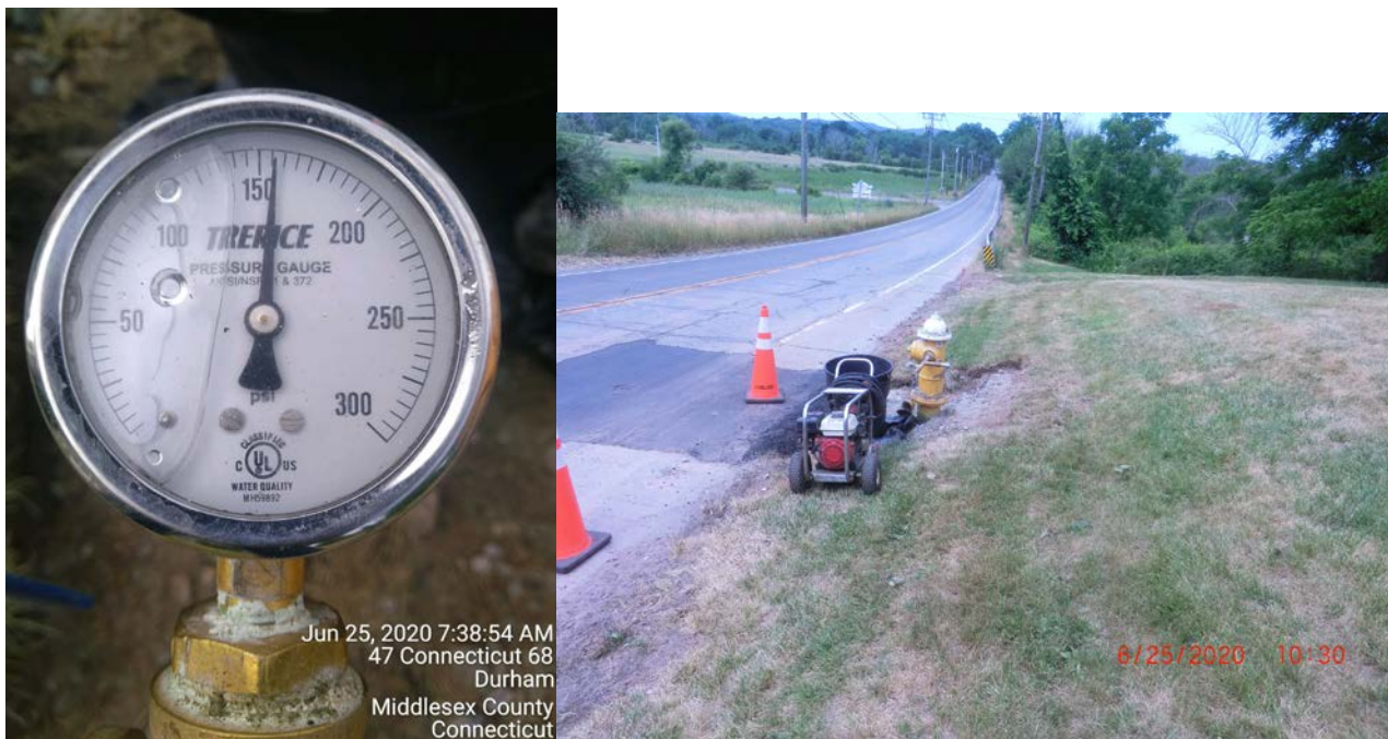
Picture 1: Ludlow begins pressure test. This is a shot taken by Ludlow on left and hydrant on right.
