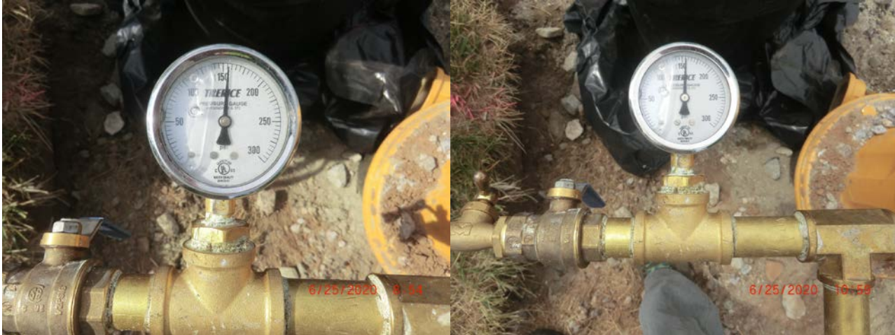
Picture 2: Two additional shots of pressure gage for test on Route 68, Wallingford Road. System held pressure for over three hours.
