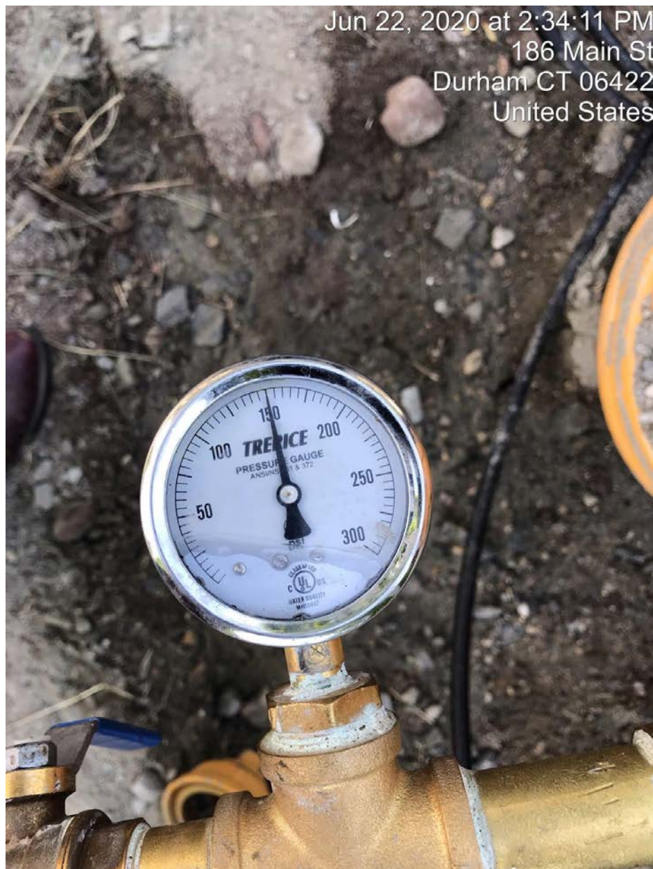
Picture 7: Pressure reading taken several minutes before pressure test was concluded today on Main Street. The meter used to monitor the pressure was placed on the hydrant located at Station 203+83 on Main Street.
