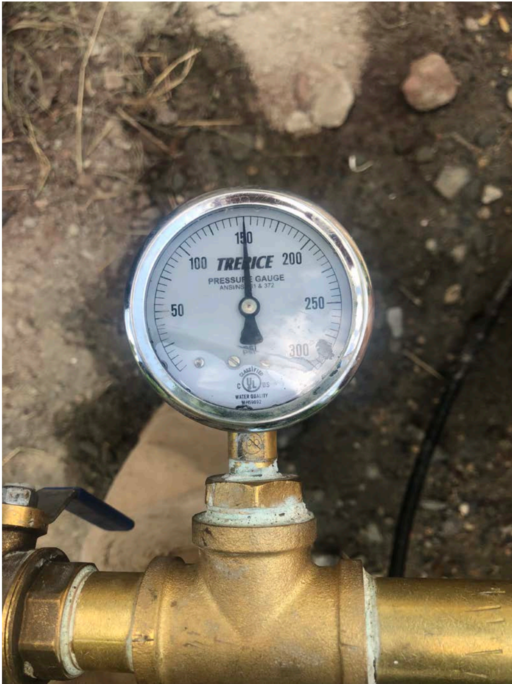
Picture 6: Starting pressure for pressure test run today. The meter used to monitor the pressure was placed on the hydrant located at Station 203+83 on Main Street.
