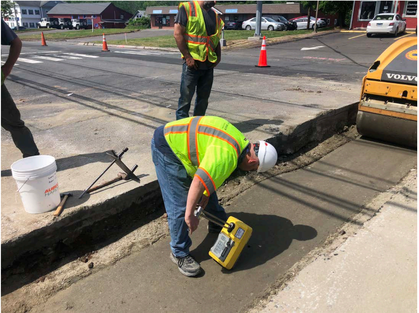
Picture 4: JTC performing soil compaction testing at Haddam Quarter Road, Durham, CT.
