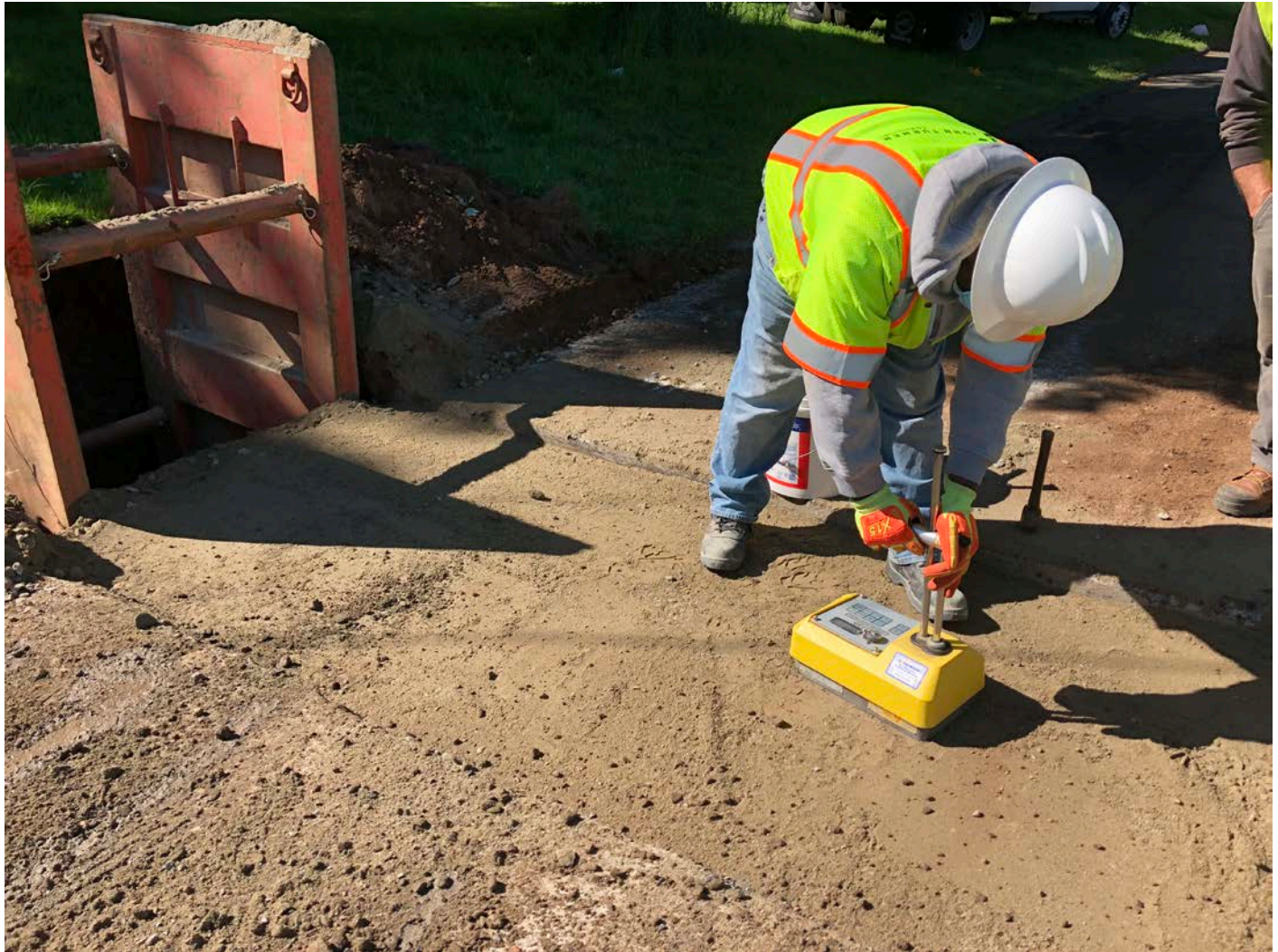
Picture 3: JTC performing soil compaction testing at Station 117+64. South Main Street, Middletown. View to the southeast.
