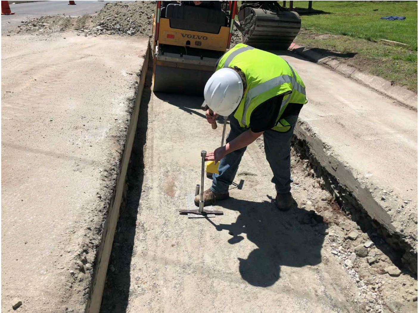
Picture 6: JTC prepares to collect soil compaction data at ~Station 196+25. View to the south. Main Street, Durham CT.
