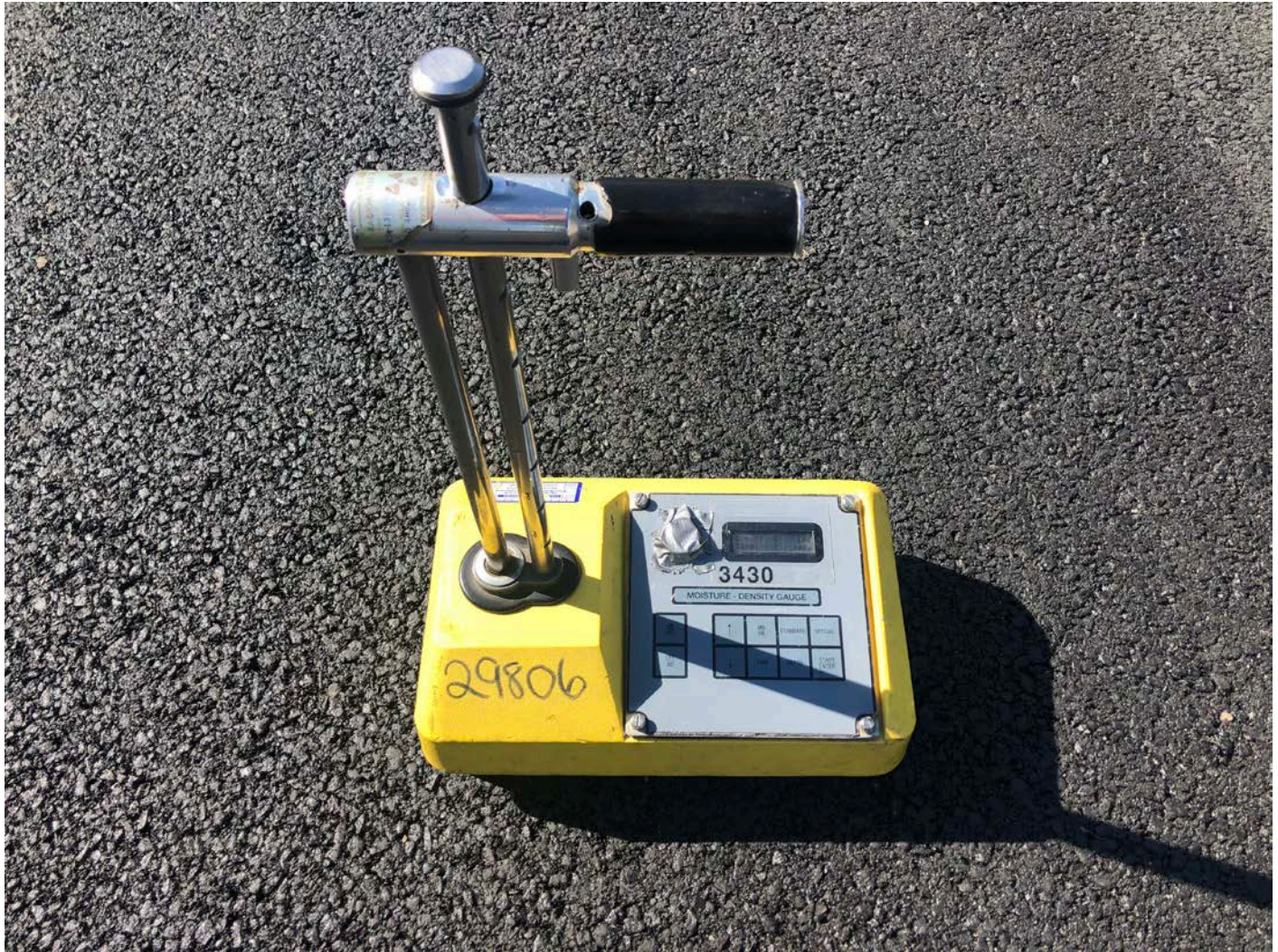
Picture 4: JTC collecting compaction test data on the asphalt placed on May 18, 2020 on Talcott Ridge Drive.
