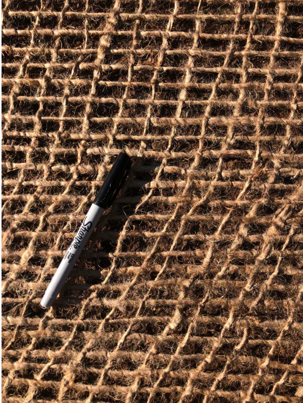
Picture 2: Close-up of jute erosion control cloth that Ludlow is placing north of the shared access road. Middletown, CT.
