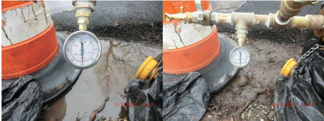
Picture 3: Little Lane (141+27) Durham water line test station at 0900 and 1100 hours. 150 PSI maintained for two hours. Other end of test was at 132+32
