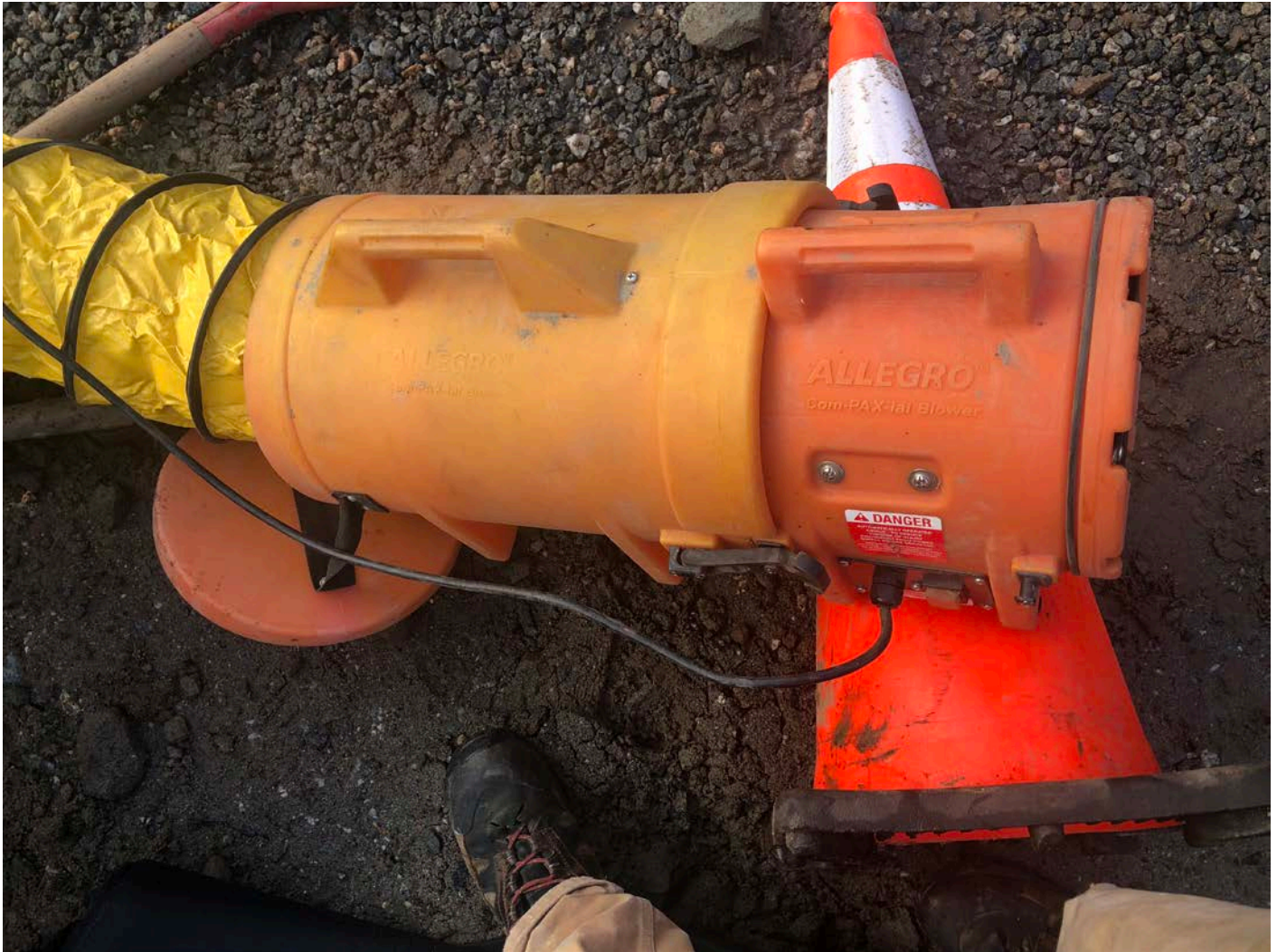
Picture 2: The blower Ludlow used to evacuate air from the catch basin while performing the confined space entry. North side of the shared access road at Station 14+40. Middletown, CT.
