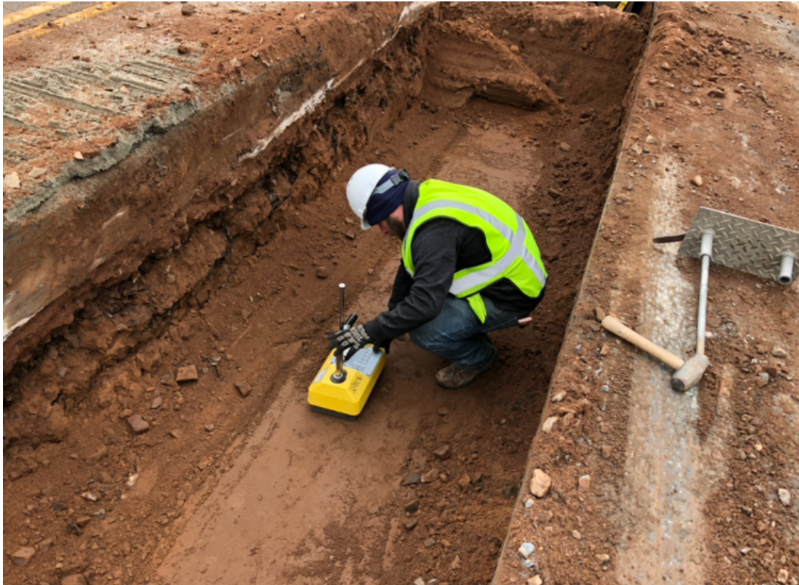
Picture 4: JTC performing soil compaction test at ~Station 168+00. View to the south. Durham, CT.
