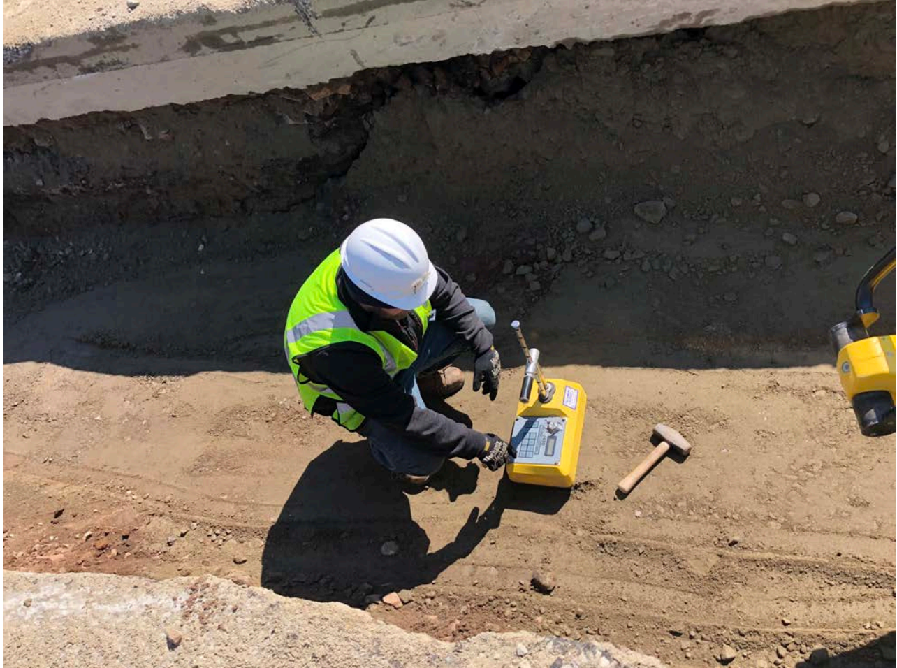
Picture 5: JTC personnel performing soil compaction test at ~Station 160+10.
