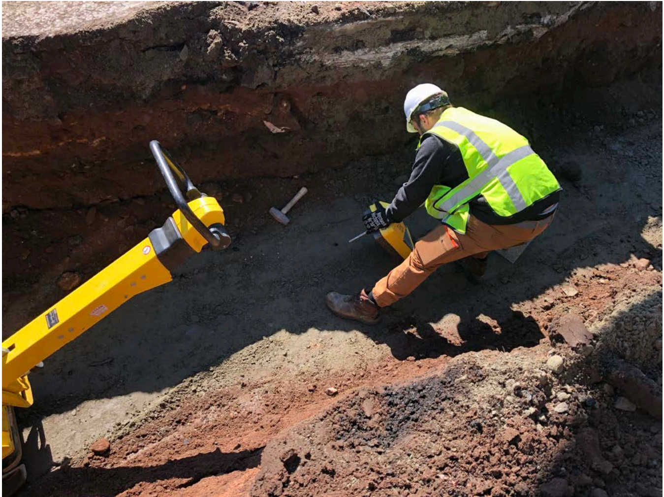
Picture 5: Compaction testing being performed at Station 751+55.
