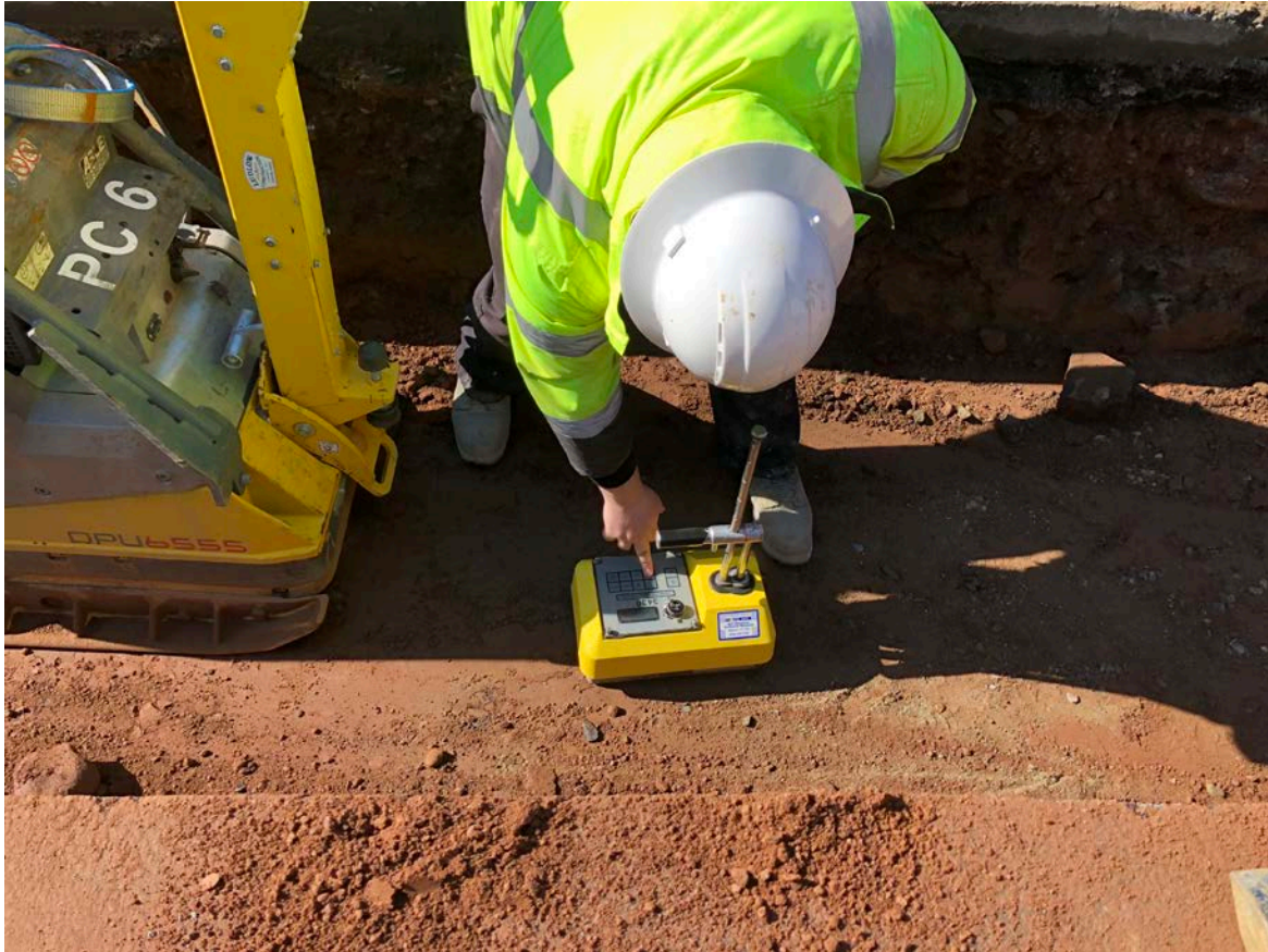
Picture 2: Soil compaction testing being performed by JTC personnel.
