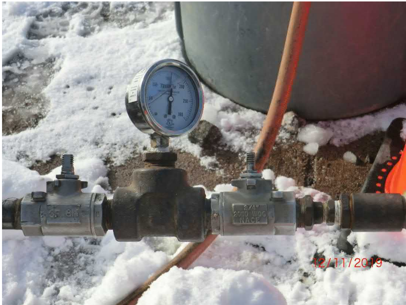
Figure 6 – New hydrant on Talcott Ridge by intersection with upper Watch Hill Dr. Pressure reading about 155 PSI. Note that angle of picture makes it appear higher.
