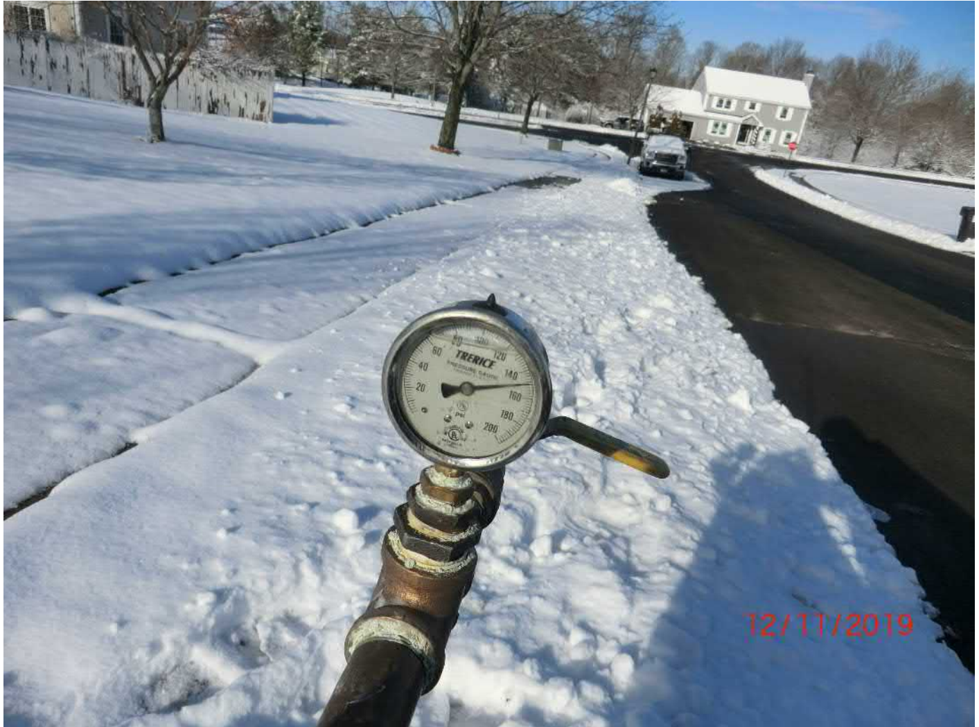
Figure 10 –Lower Watch Hill hydrant gauge reading a hair under 150 PSI.
