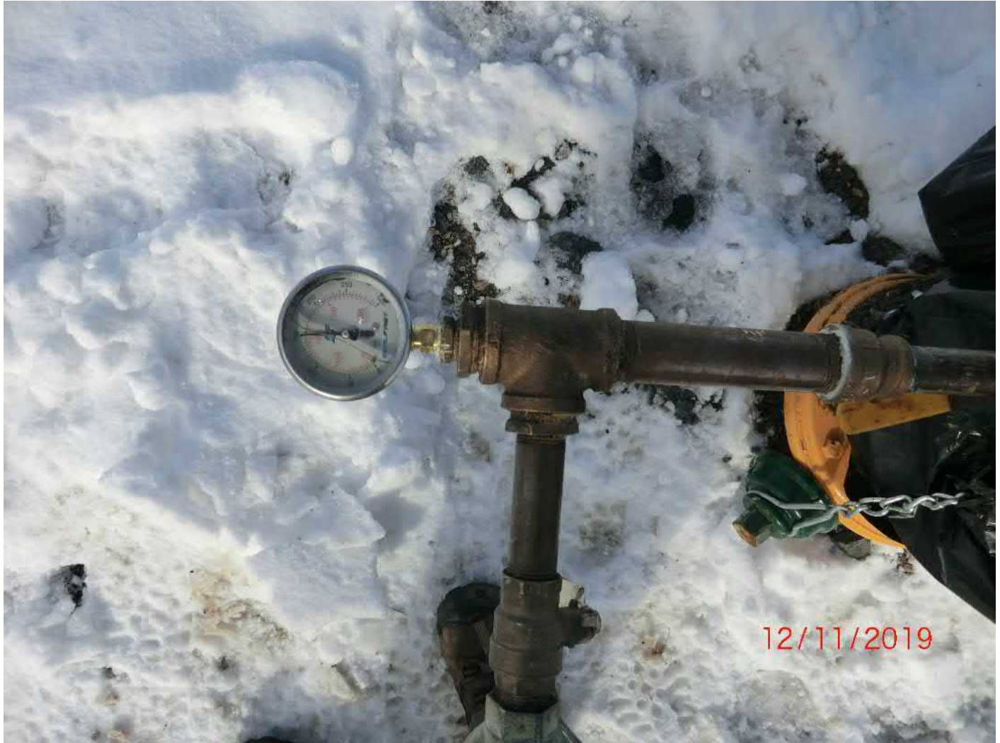
Figure 2 – Upper Watch Hill hydrant under pressure at 150 PSI.
