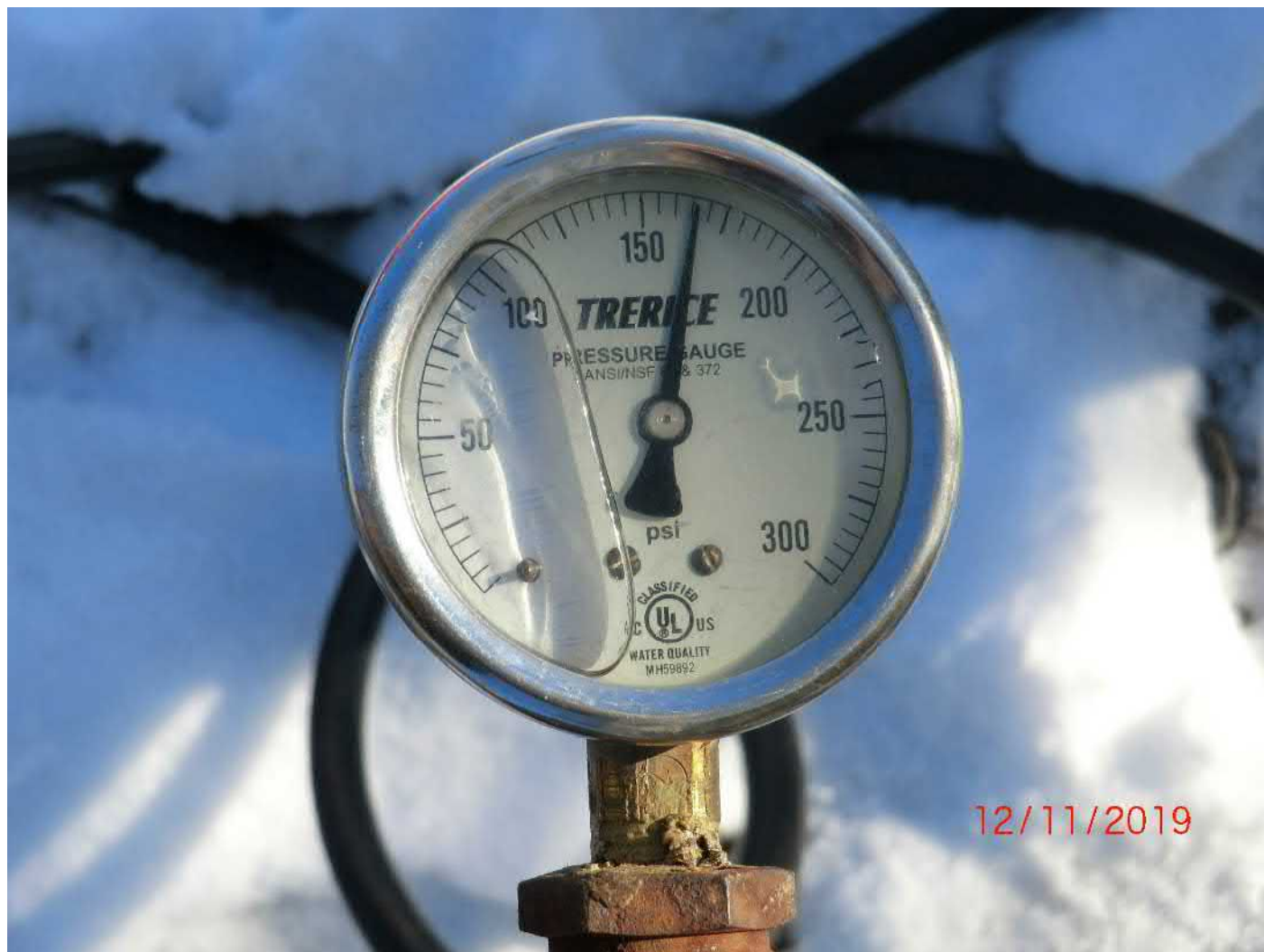
Figure 12 – Gauge on hydrant located at intersection of Talcott Ridge and S. Main Street. Reading 167 PSI.
