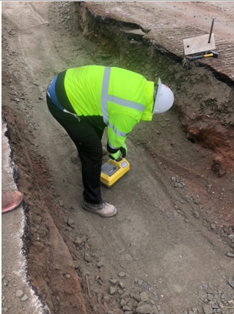
Figure 14– John Turner Consulting performing a compaction test on the top-most lift of 3”minus gravel.
