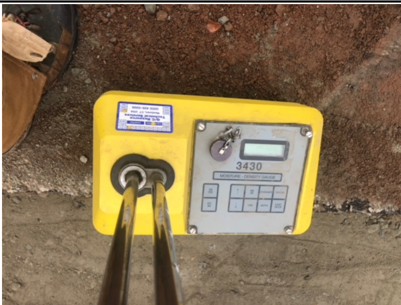
Figure 15– Density and moisture meter used by John Turner Consulting.
