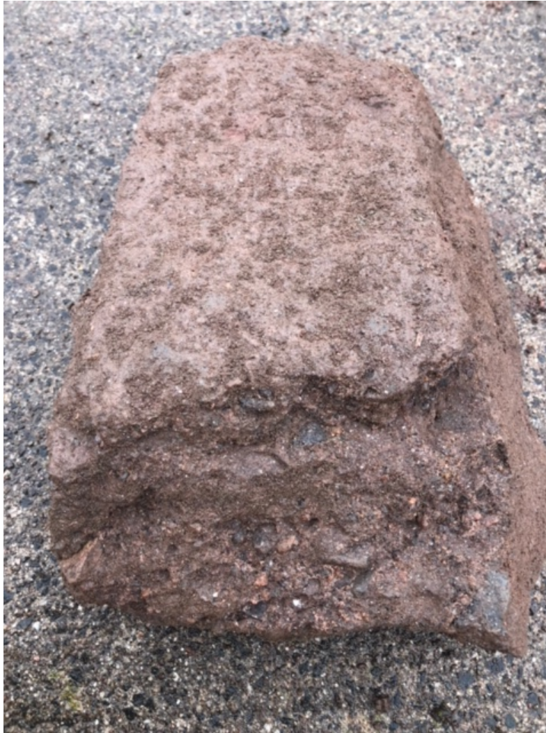
Figure 8 – Typical bedrock that Ludlow encountered during trench excavation activities while placing the third and fourth stick of 8" DIP.
