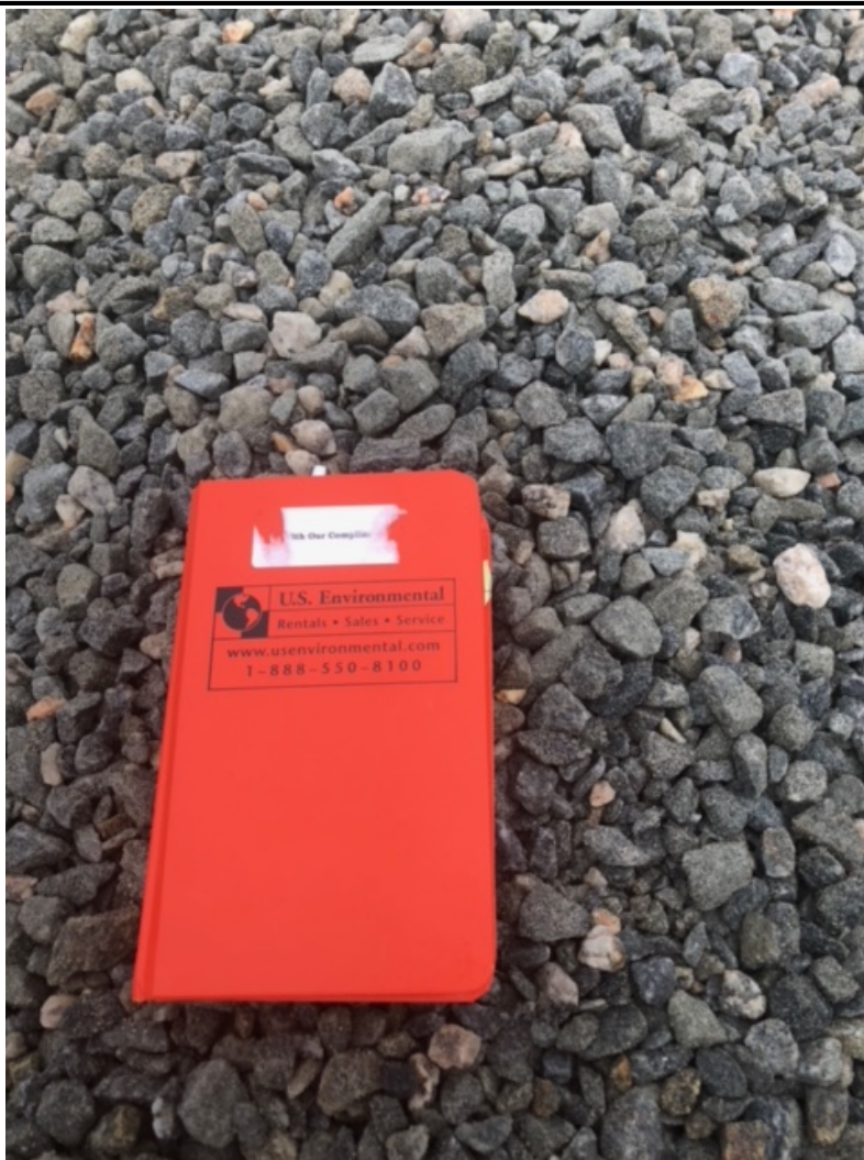
Figure 11– Typical ¾” gravel used during pipe placement and backfilling.
