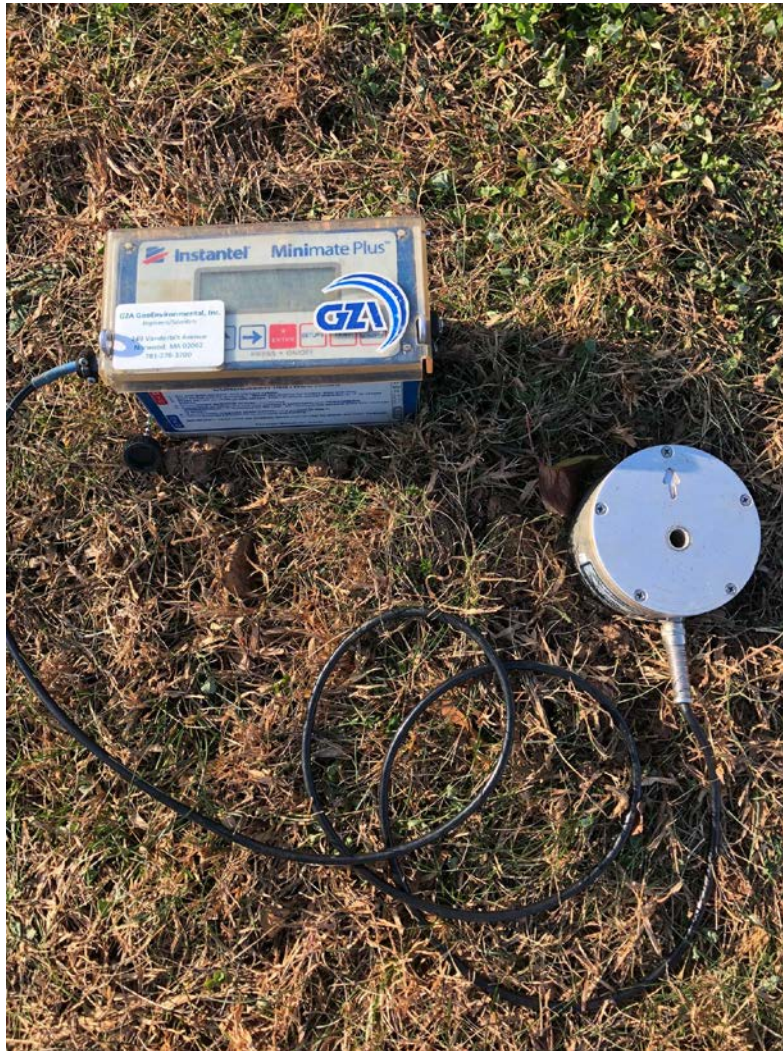
Figure 4 – One of the vibration meters used by GZA today.
