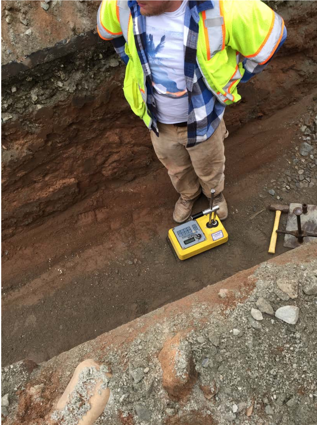
Figure 10 – Compaction testing at 42+54. Deepest level tested. Additional levels tested at 43+49.
