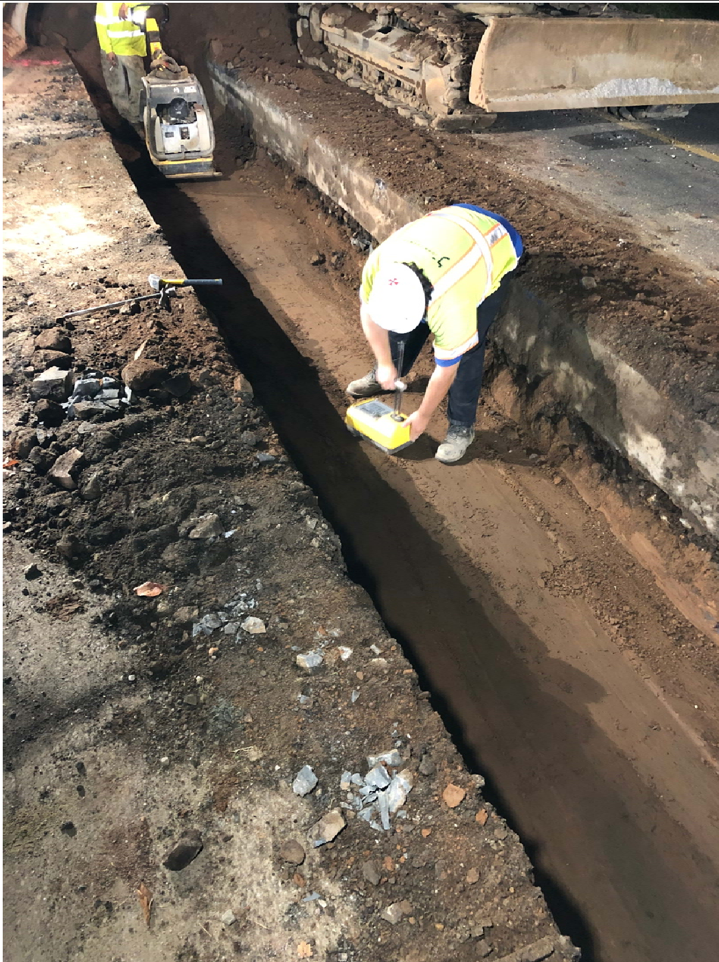
Figure 3 – Compaction testing over sections 1, 2
