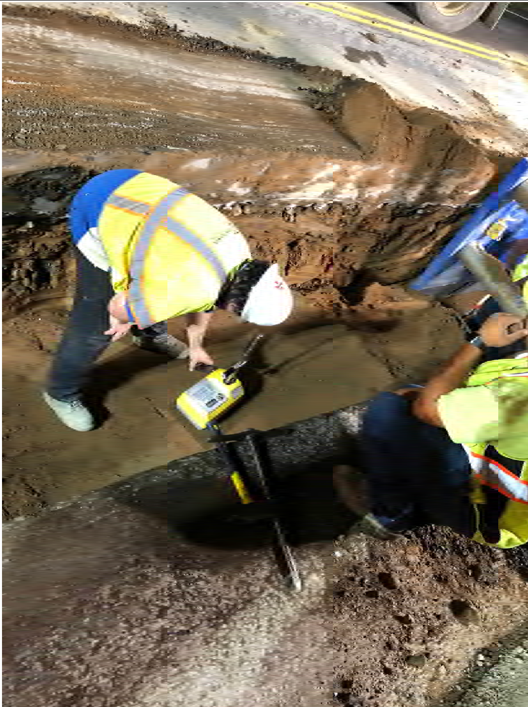
Figure 4 – Compaction testing underway
