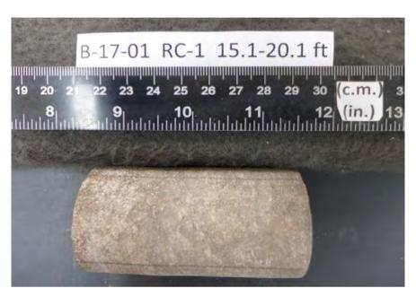
After cutting and grinding
