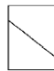
Type 4 Diagonal fracture with no cracking through ends; tap with hammer to distinguish from Type 1
