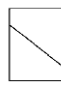
Type 4 Diagonal fracture with no cracking through ends; tap with hammer to distinguish from Type 1
