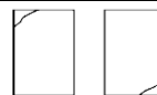
Type 5 Side fractures at top or bottom (occur commonly with unbonded caps)
