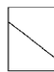
Type 4 Diagonal fracture with no cracking through ends; tap with hammer to distinguish from Type 1
