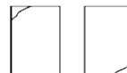
Type 5 Side fractures at top or bottom (occur commonly with unbonded caps)
