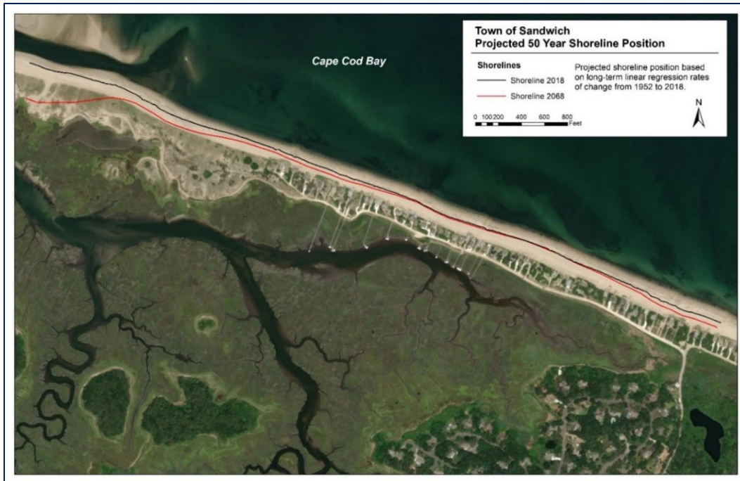
Figure 2-16: Existing (2018) and projected (2068) MHW shoreline positions, Springhill Beach (WHG, 2020)
