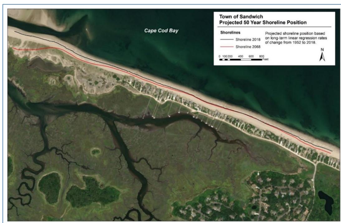
Figure 4-3: Existing (2018) and projected (2068) MHW shoreline positions, Springhill Beach (WHG, 2020)
