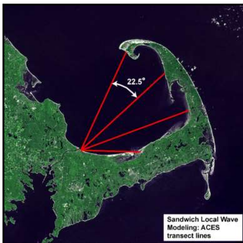
Figure 23. Angle bands describing the semi-restricted geometry of Cape Cod Bay affecting locally generated waves near the Cape Cod Canal.
