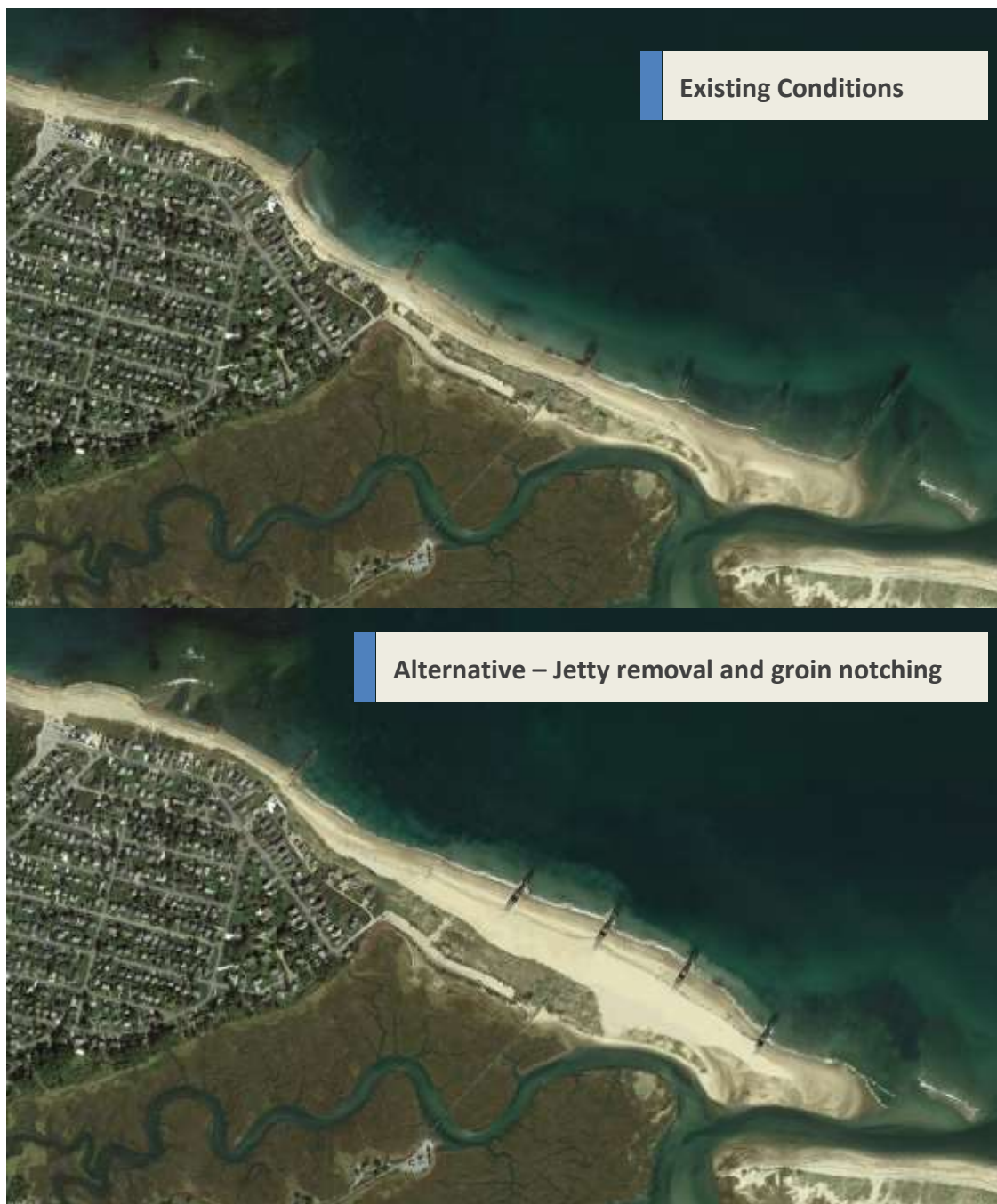
Figure 52. Old Sandwich Harbor jetty removal and groin notching alternative.
