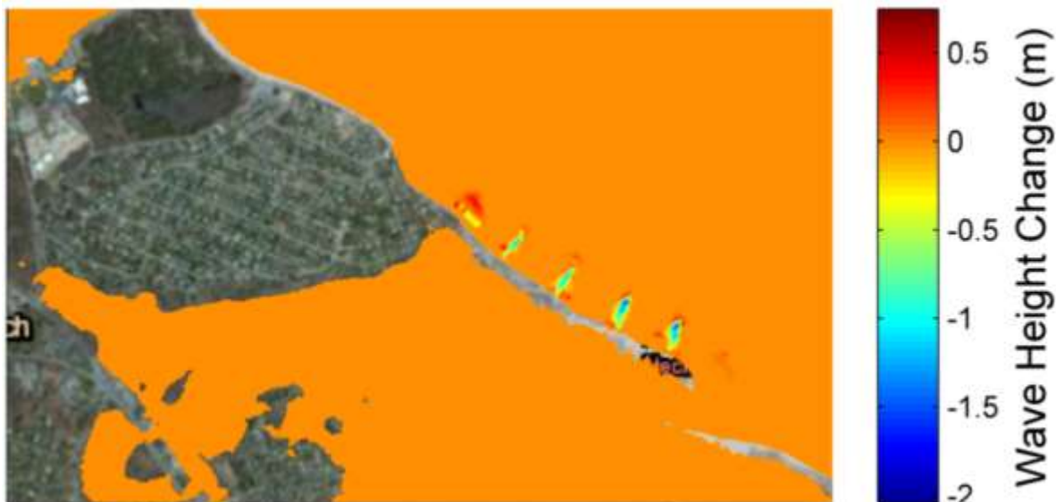
Figure 53. Wave simulation wave height results comparison for. Positive wave height change means higher waves with the alternative in place.
