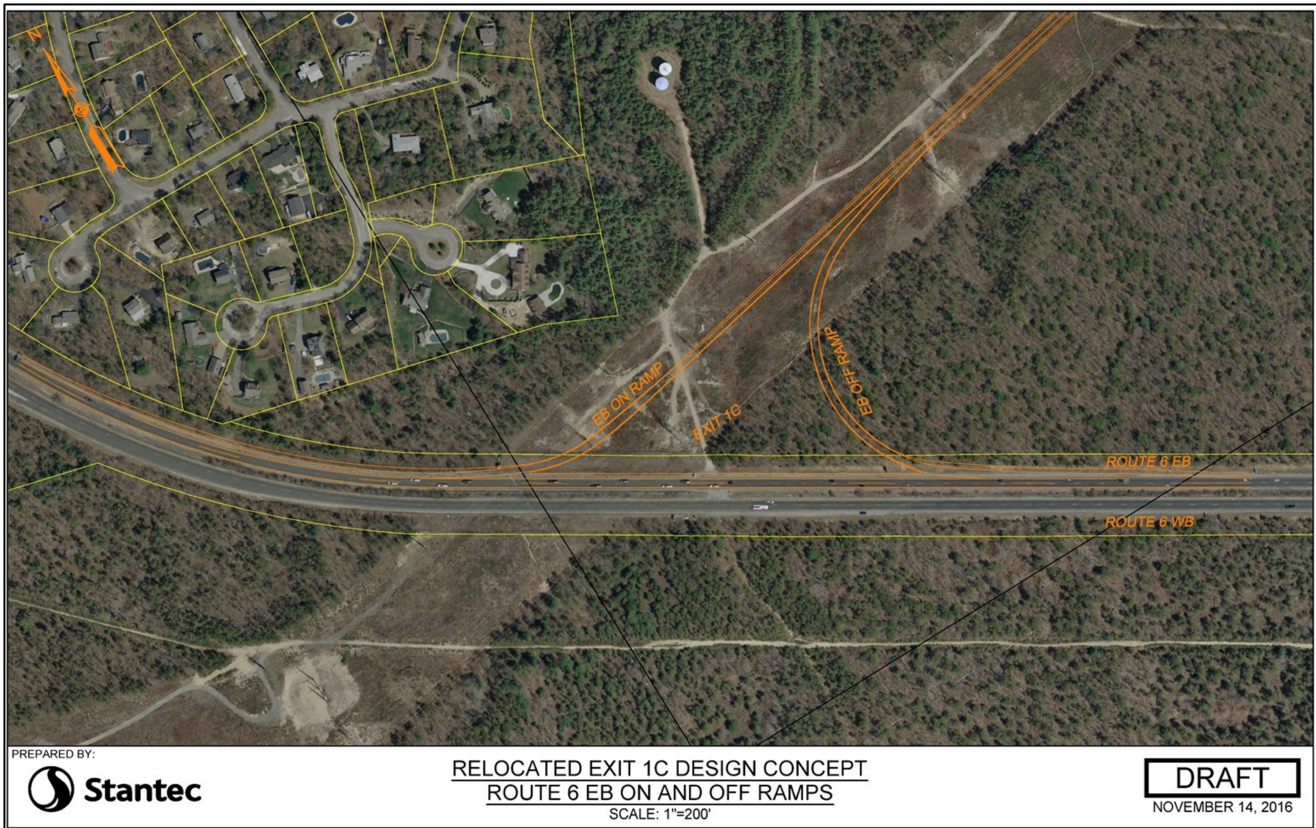
Figure 8. Relocated Exit 1C Design Concept Route 6 EB On and Off Ramps.
