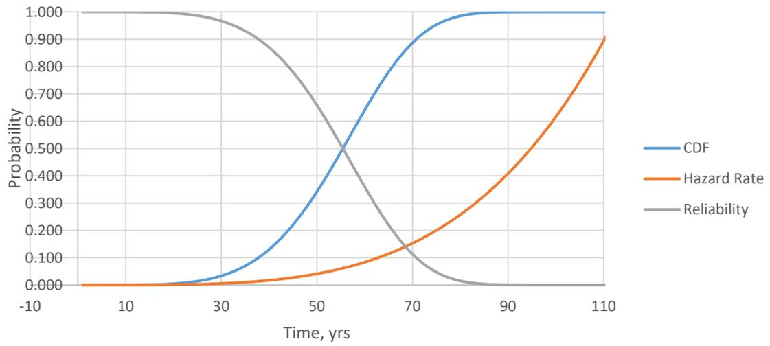
Figure 8-3 - Substructure - Weibull CDF and Hazard Rate
