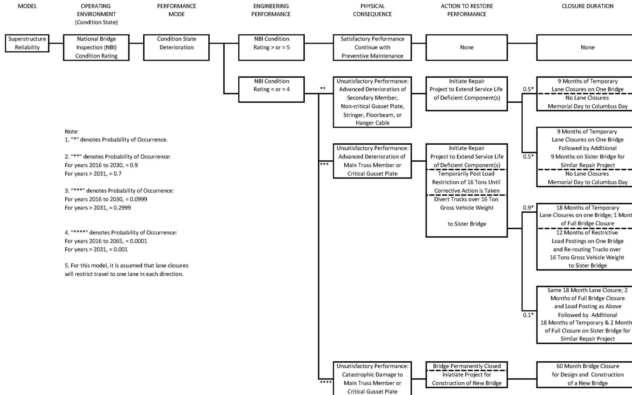
**FIGURE 8-4: SUPERSTRUCTURE DETERIORATION MODEL-EVENT TREE**
