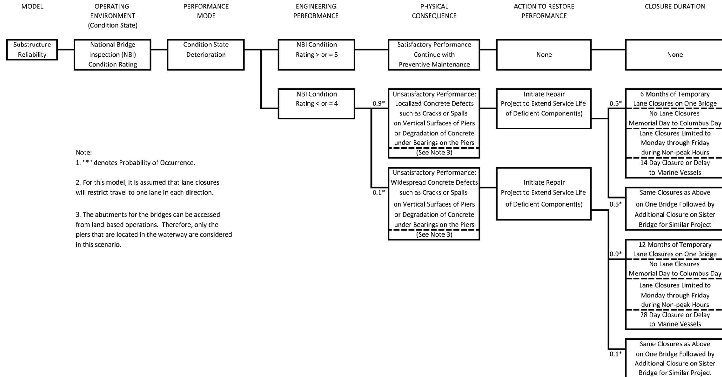
**FIGURE 8-6: SUBSTRUCTURE DETERIORATION MODEL-EVENT TREE**
