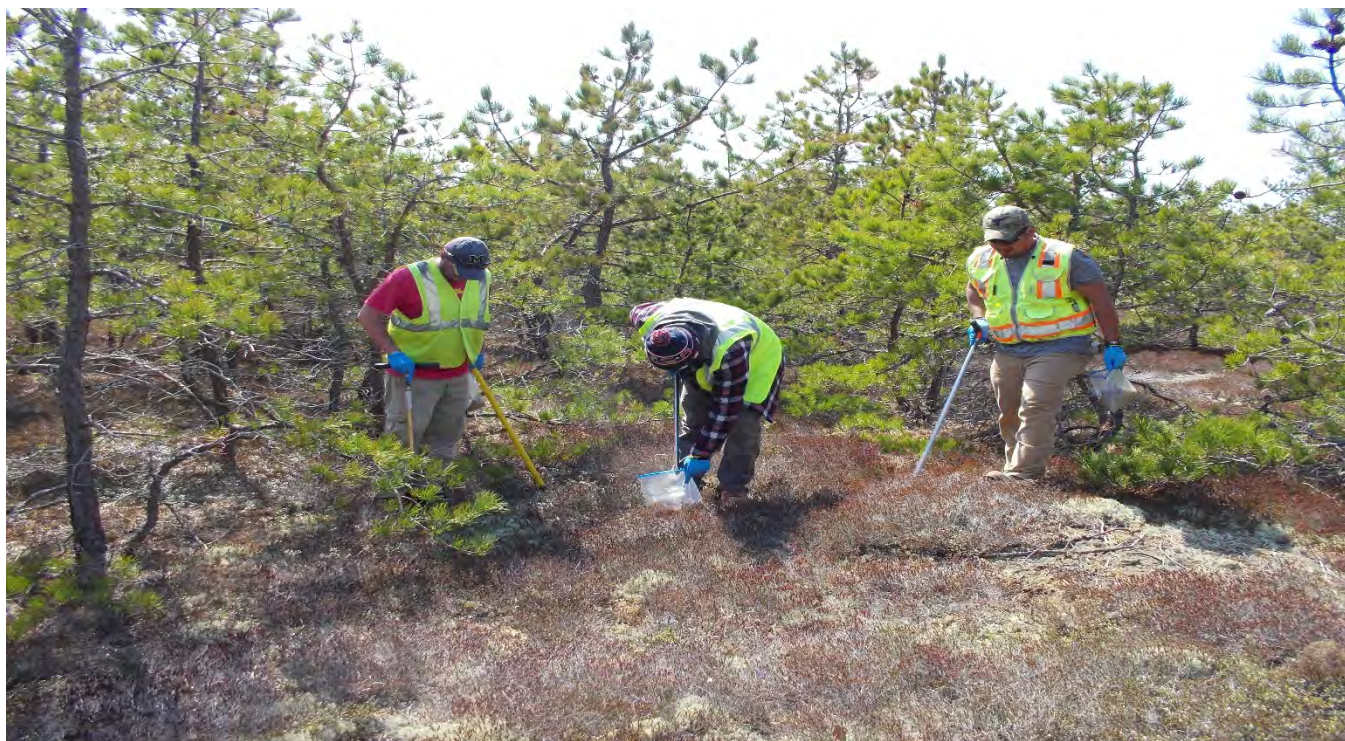
Photo 02 – UXO team and field personnel using step probes to collect soil samples. Date: 13 April 2018
