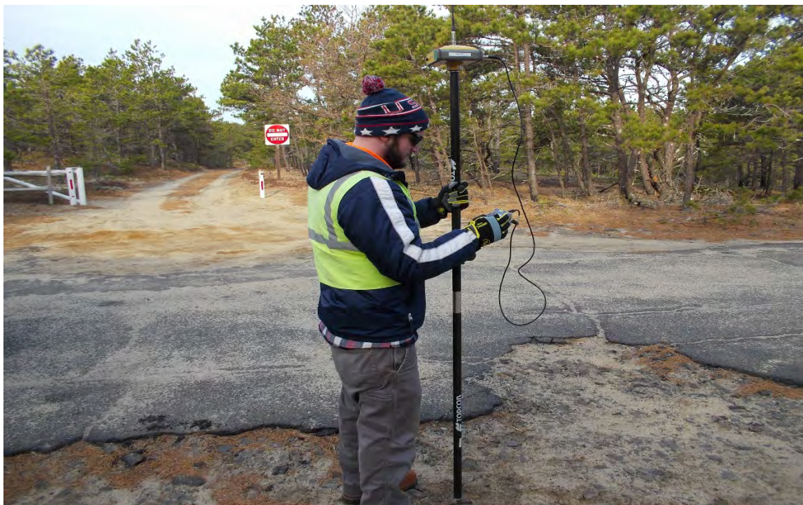
Photo 04 – Field personnel performing RTK base station check to ensure accuracy. Date: 12 April 2018
