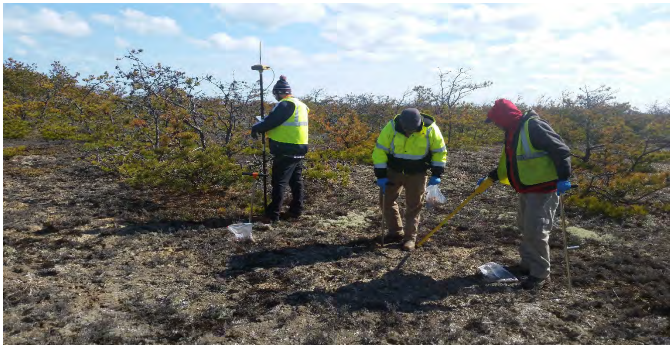
Photo 03 – UXO team performing sweep of surface soils with a Schonstedt before sampling. Field personnel using RTK rover to validate location. Date: 12 April 2018
