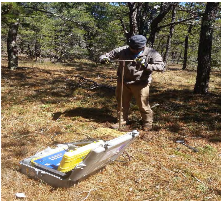
Photo 06 – UXO field personnel using hand auger in AOI-01 to collect discrete samples. Date: 14 April 2018
