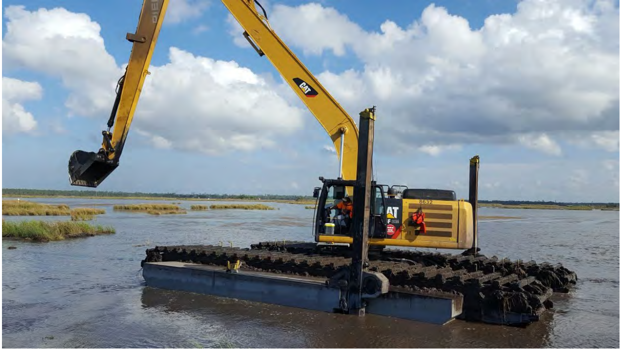
Figure 7. Alternative 4 – Amphibious Dredge - Mechanical. Source: BIG Dredging
