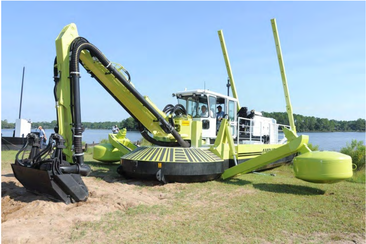
Figure 8. Alternative 4 – Amphibious Dredge - Mechanical. Source: Amphibex
