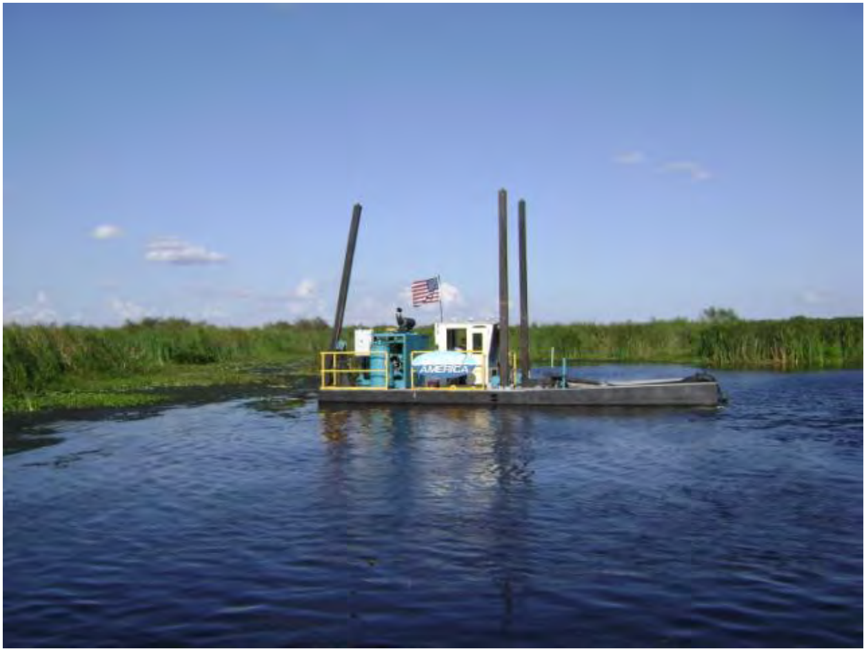
Figure 1. Alternative 1 - Swinging Ladder Dredge. Source: Dredge Supply Company
