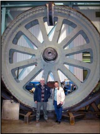
Housed in the top of each tower are four sheaves (as seen in photo above). Each one is 16 feet in diameter and weighs 34 tons! With the help of four 150-horsepower electric motors the sheaves turn, moving the cables that lower the span and raise the counterweights.
