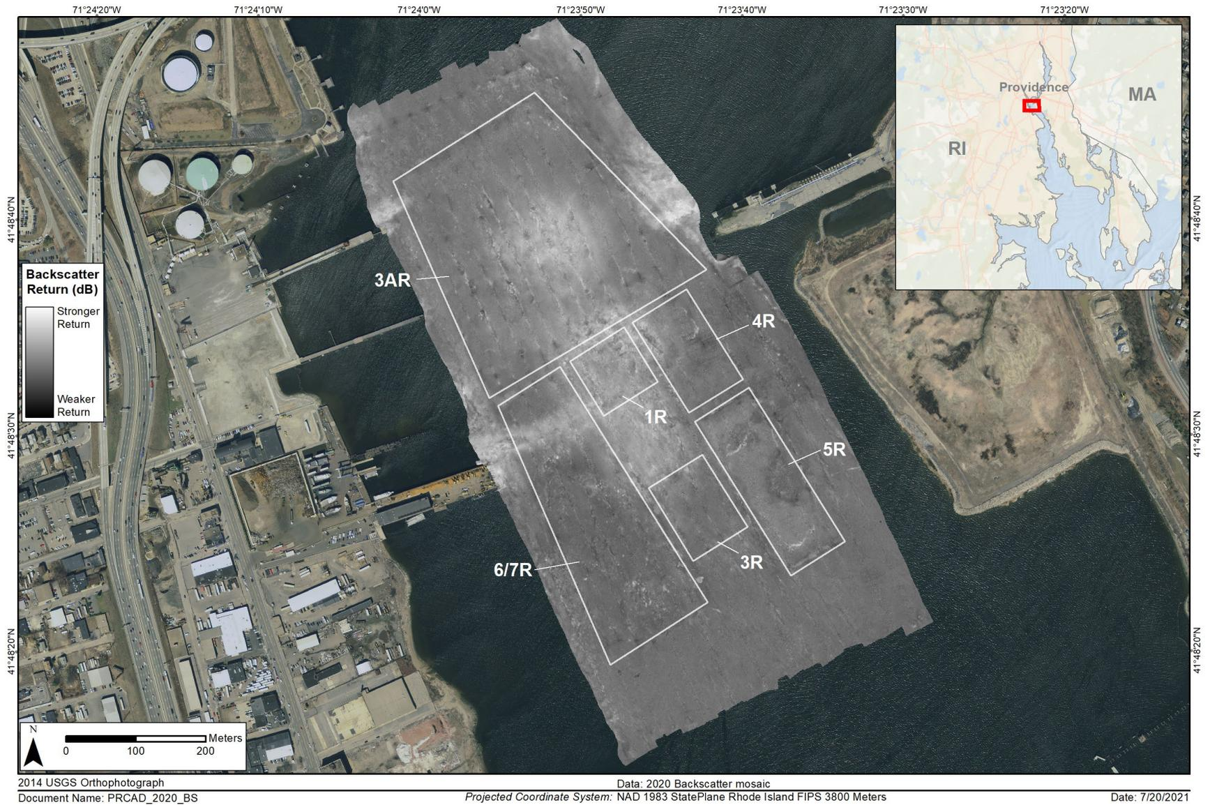
Figure 3-2. Mosaic of unfiltered backscatter data of PRCAD – September and October 2020
