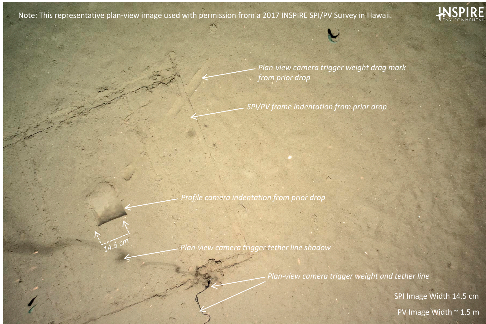
Figure 2-7. This representative plan view image shows the sampling relationship between plan view and sediment profile images. Note: plan view images differ between surveys and stations and the area covered by each plan view image may vary slightly between images and stations.
