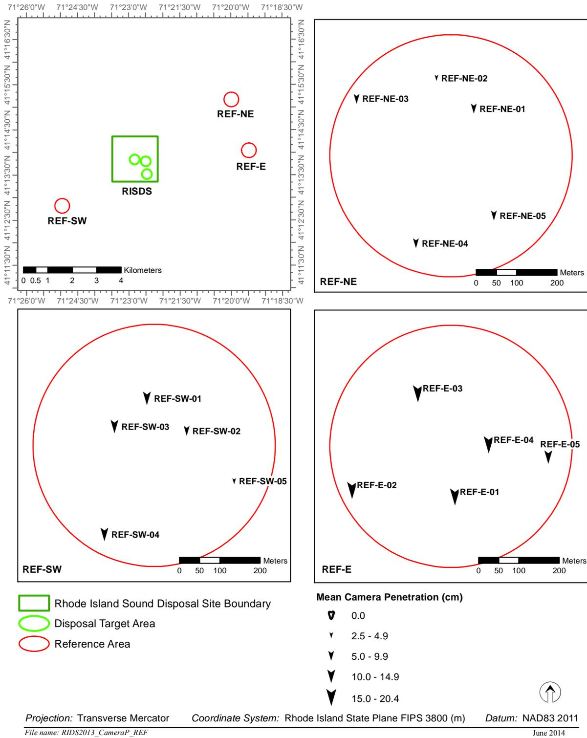
**Figure 3-10.** Mean station camera prism penetration depths (cm) at the RISDS reference areas
