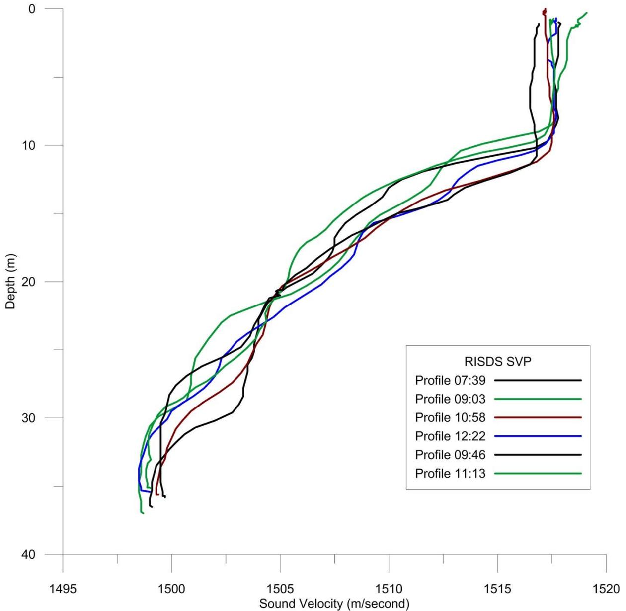
**Figure 2-2.** Sound-velocity profiles from 27 August 2013 at RISDS
