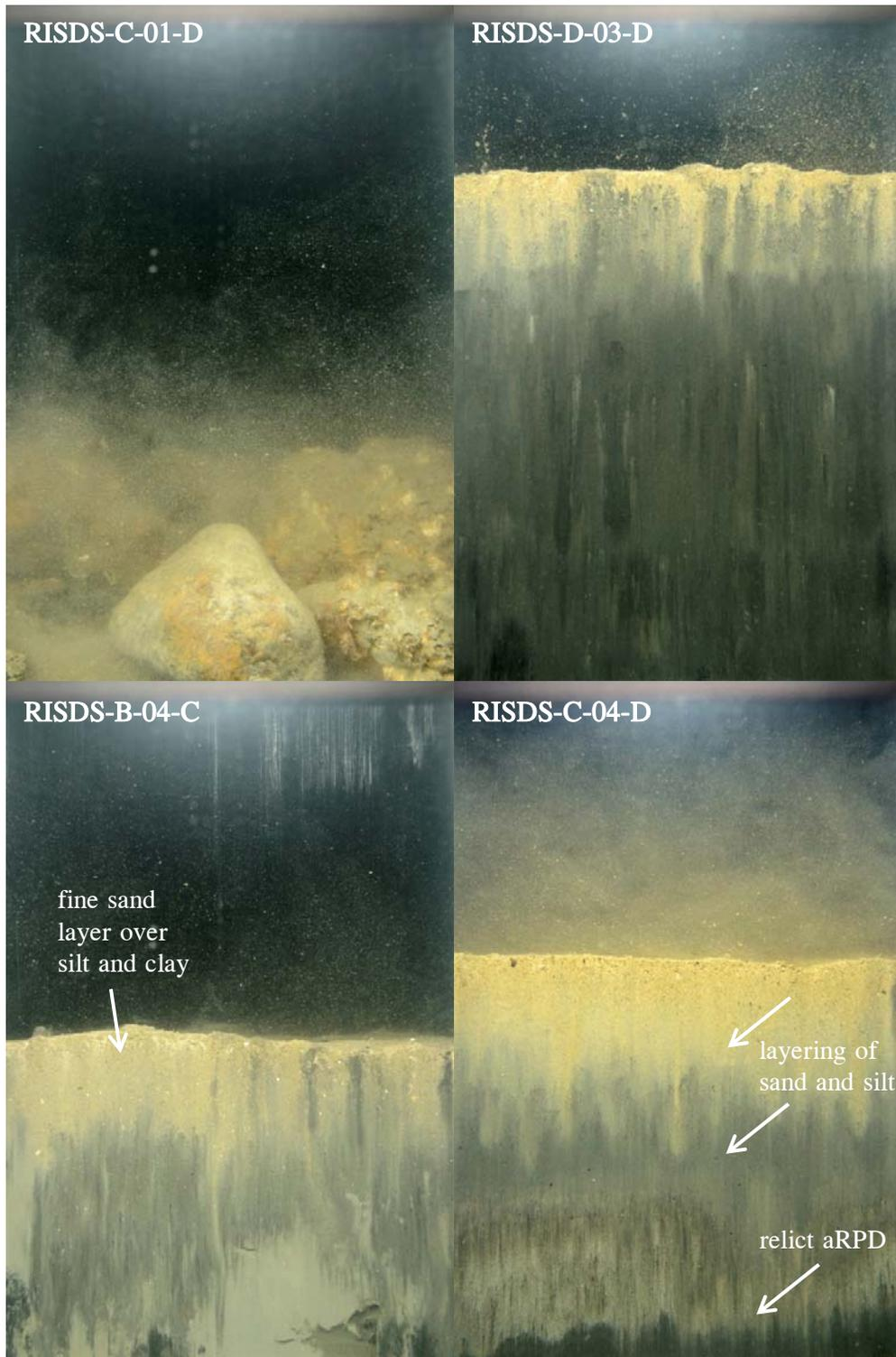
**Figure 3-18.** Sediment grain size and penetration variation at stations sampled within RISDS disposal target areas
