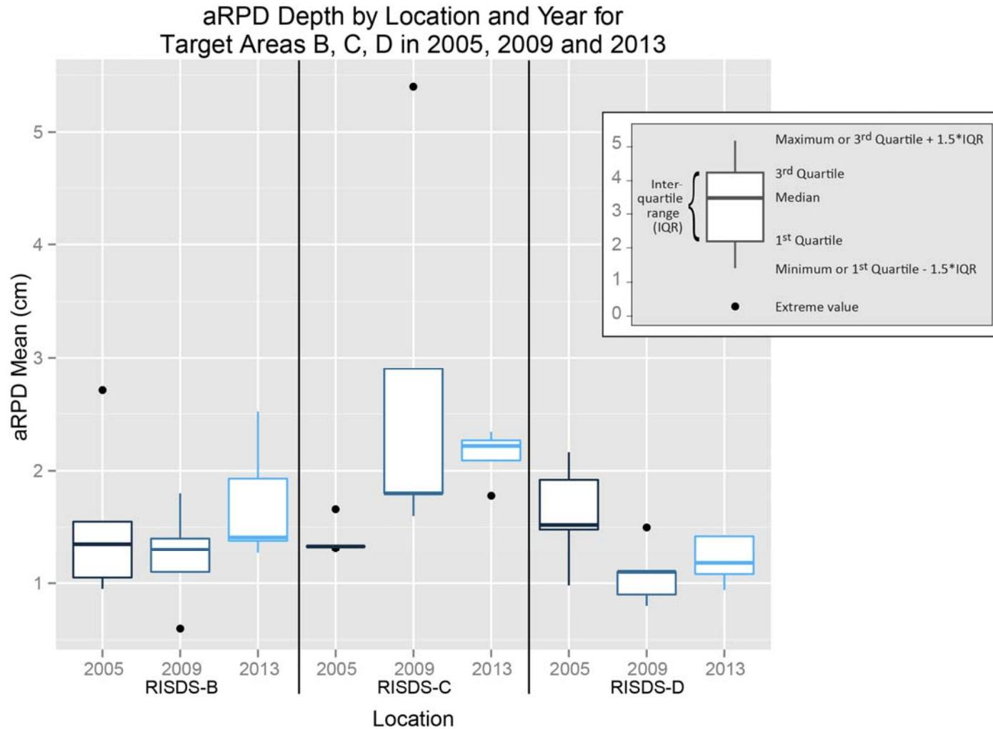
**Figure 3-25.** Boxplots showing the distribution of mean aRPD depths measured at disposal site target areas RISDS-B, RISDS-C, and RISDS-D in 2005, 2009 and 2013.
