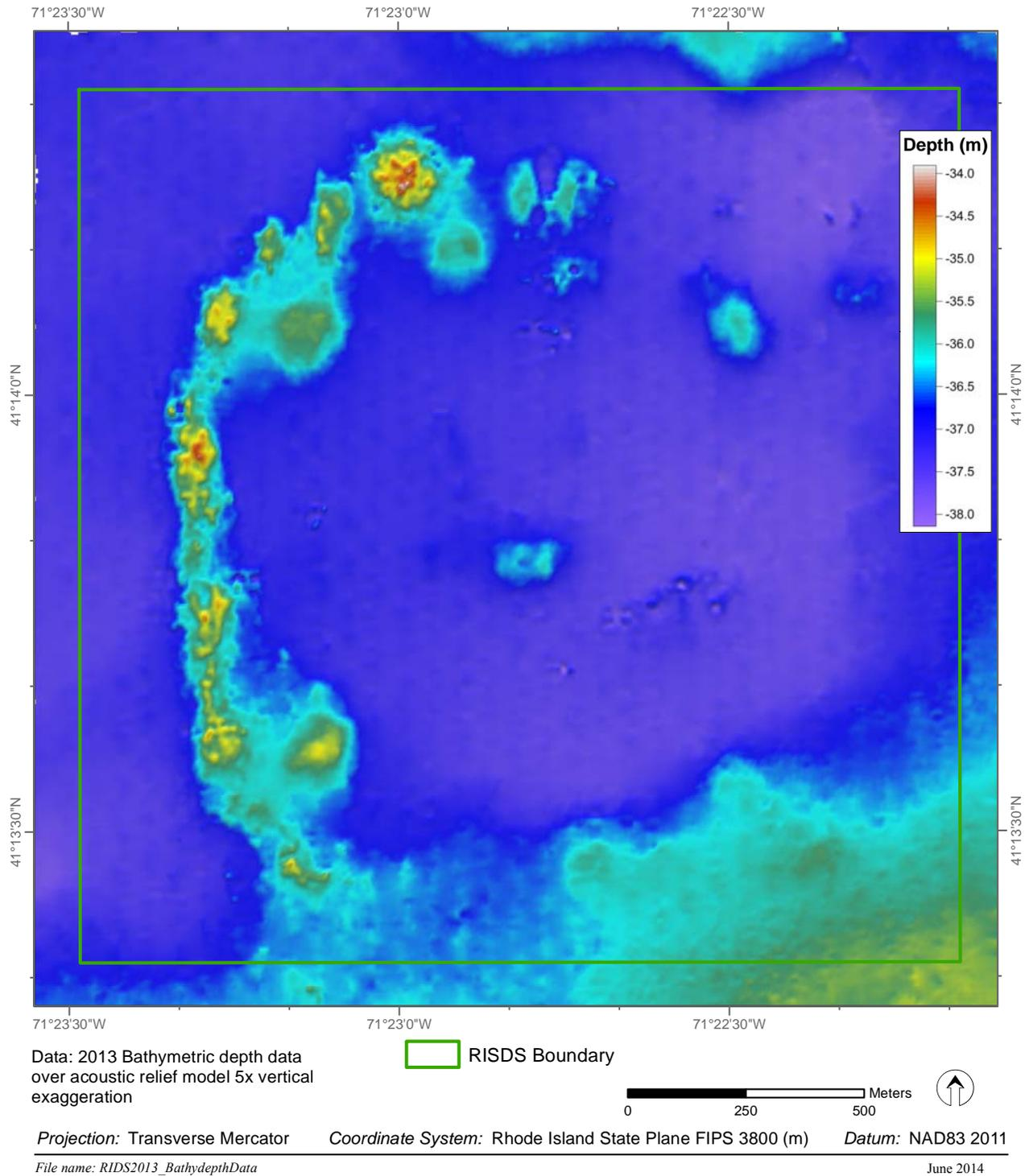
**Figure 3-2.** Bathymetric depth data over acoustic relief model of RISDS – August 2013
