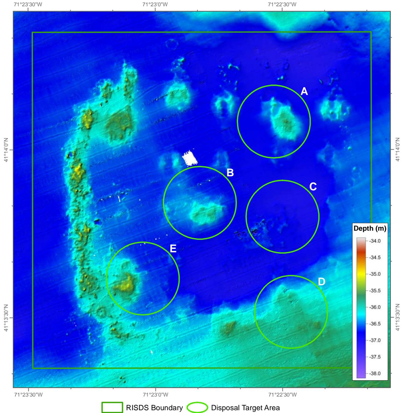
Data: 2008/2009 NOS Bathymetric depth data over acoustic relief model 5x vertical exaggeration.
