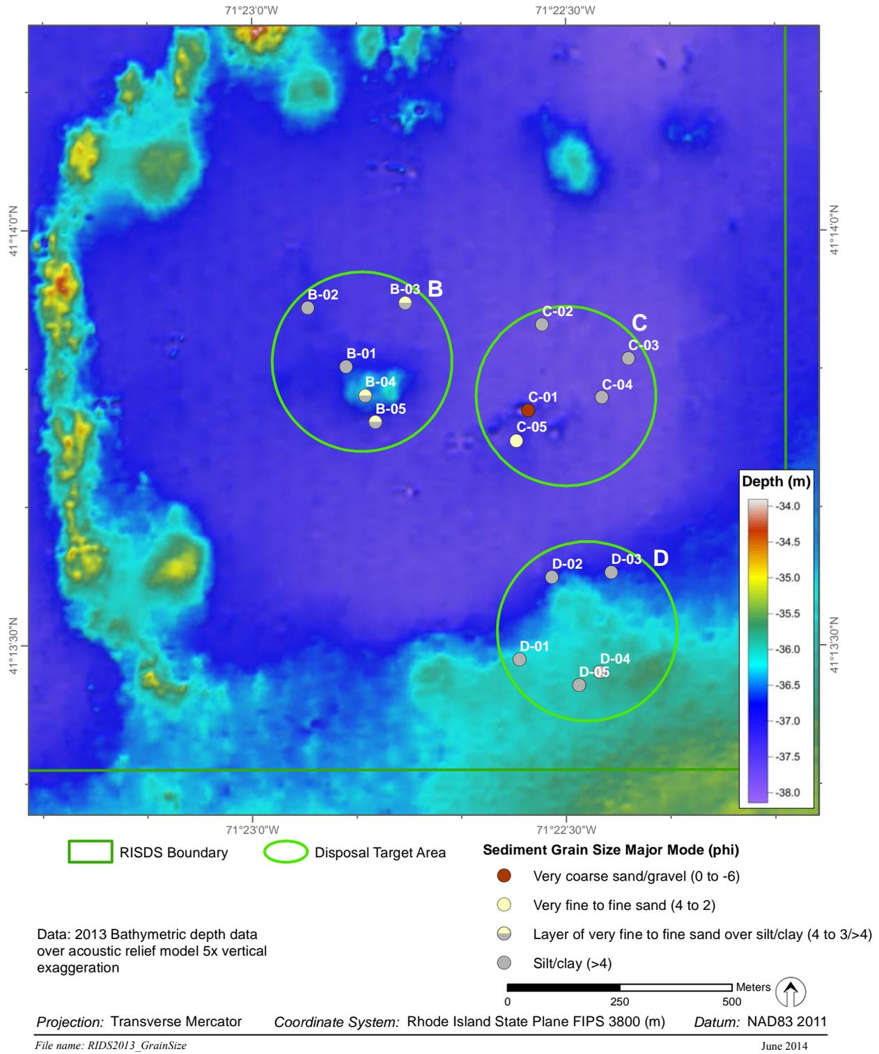
**Figure 3-17.** Sediment grain size major mode (phi units) at stations sampled within RISDS disposal target areas
