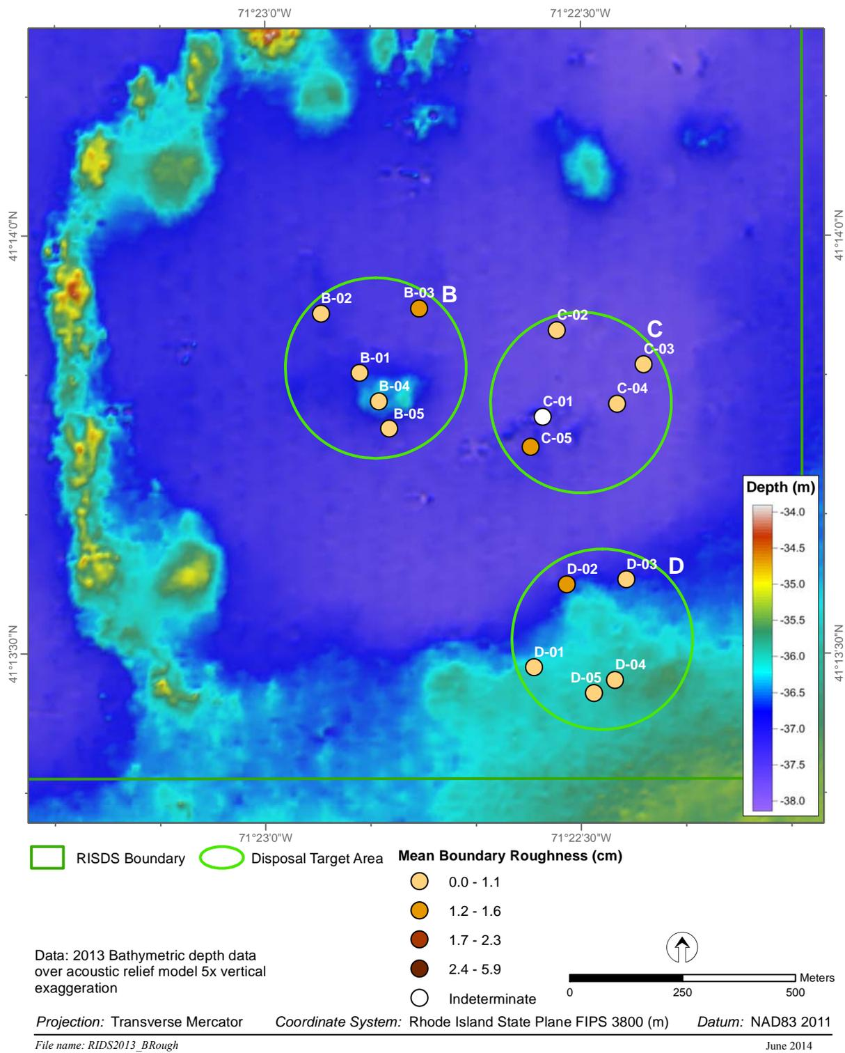
**Figure 3-20.** Mean station small-scale boundary roughness values (cm) at stations sampled within RISDS disposal target areas
