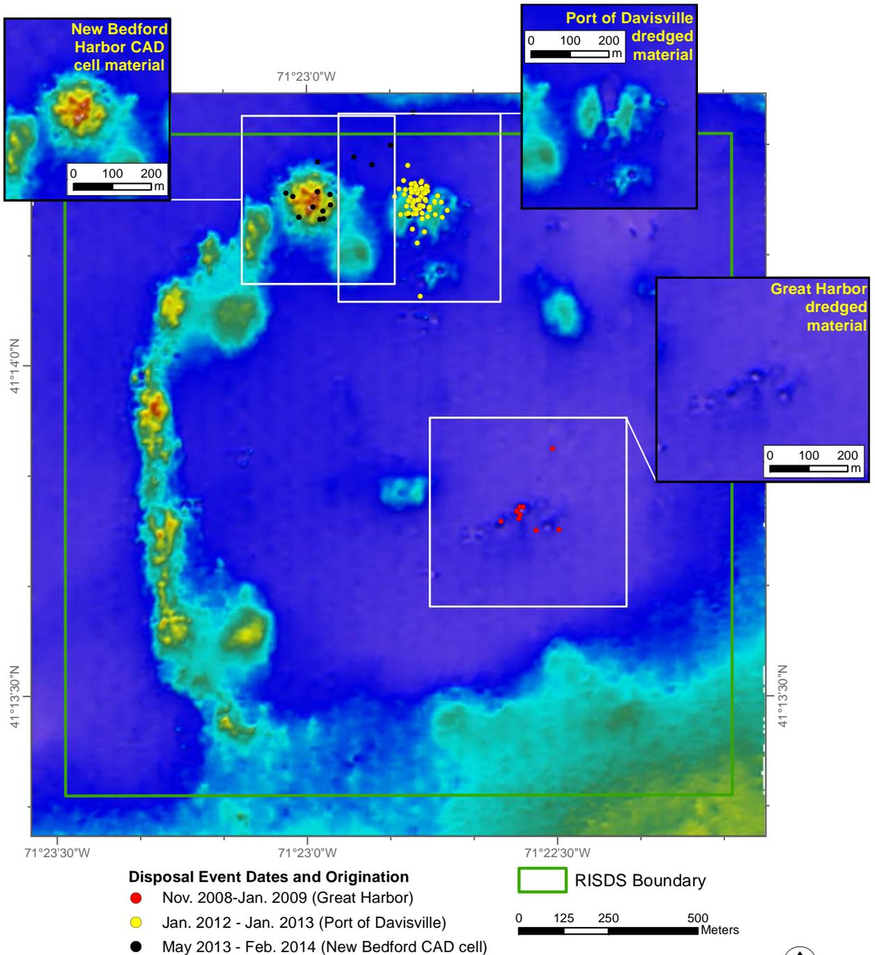
Data: 2013 Bathymetric depth data over acoustic relief model 5x vertical exaggeration
