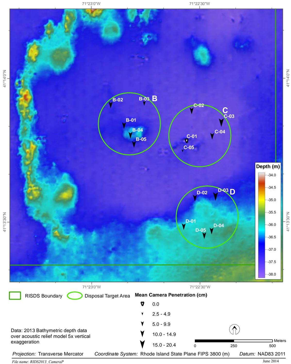
**Figure 3-19.** Mean station camera prism penetration depths (cm) at stations sampled within RISDS disposal target areas
