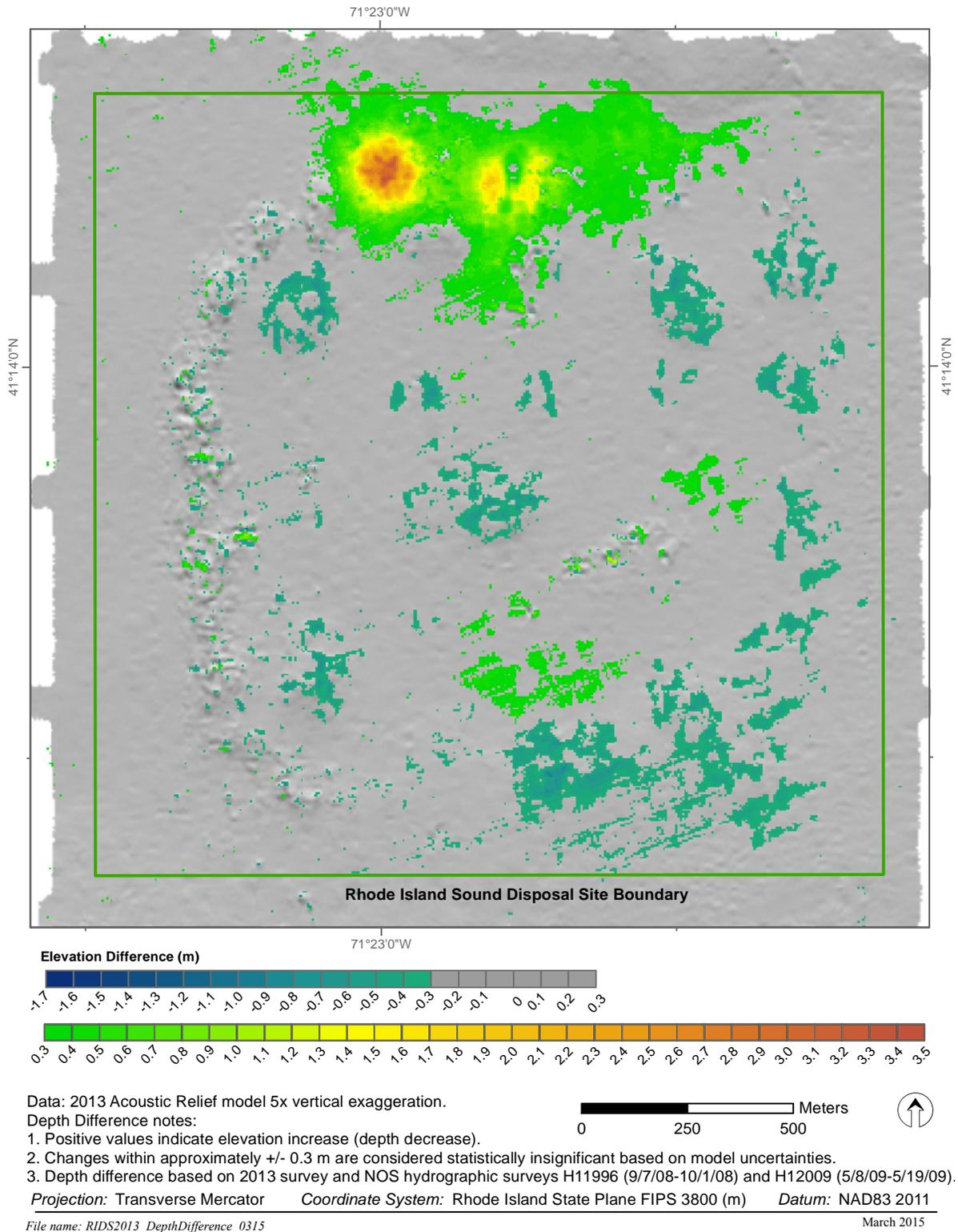
**Figure 3-6.** RISDS depth difference: 2013 vs. 2008 and 2009
