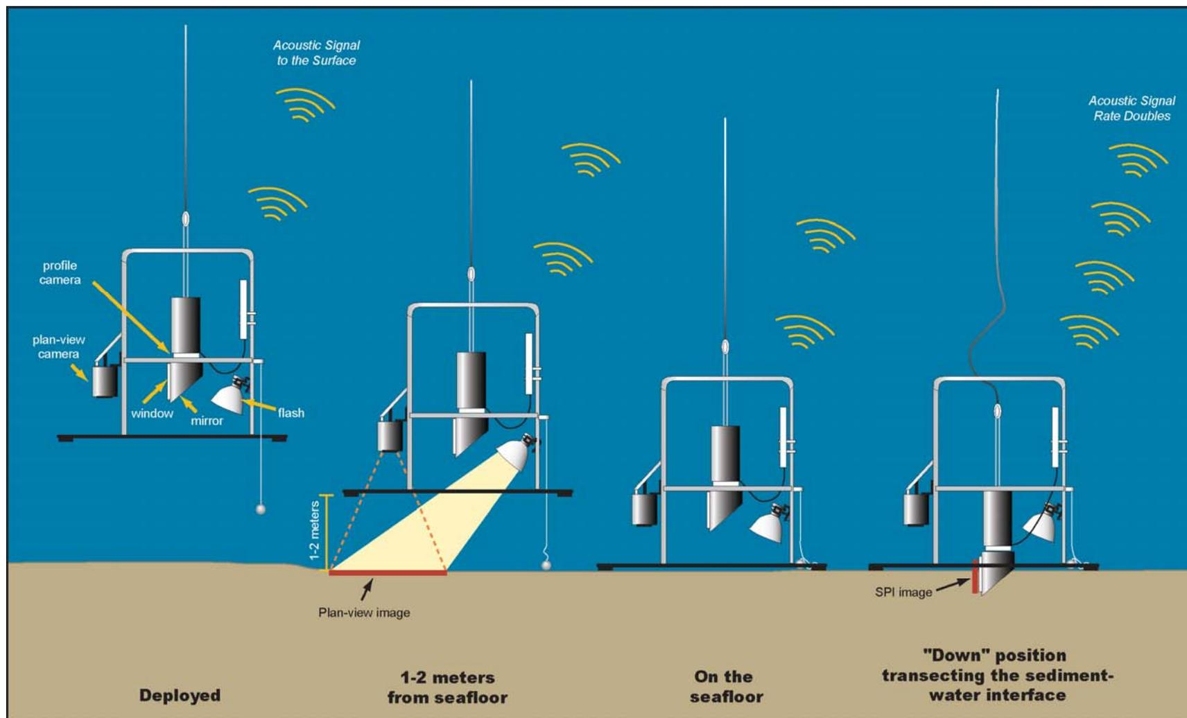
**Figure 2-5.** Schematic diagram of the SPI/PV camera deployment
