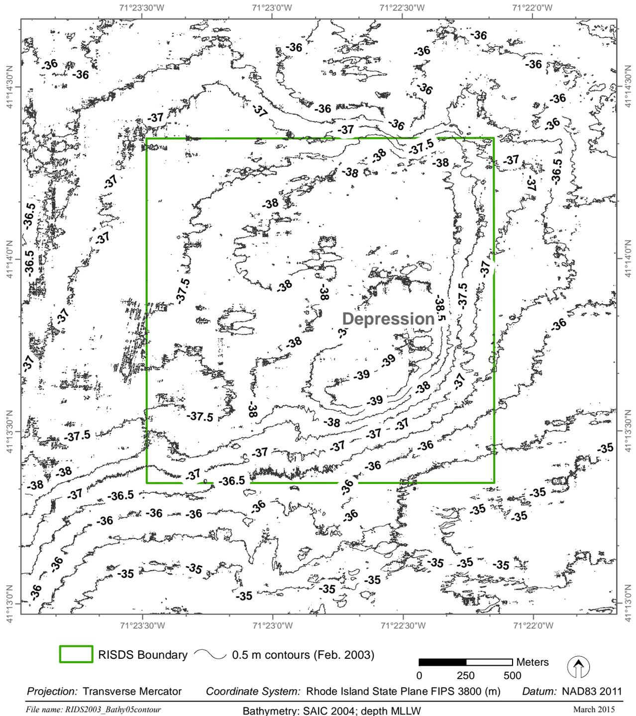
**Figure 1-2.** Bathymetric contour map of RISDS in February 2003, prior to any dredged material placement
