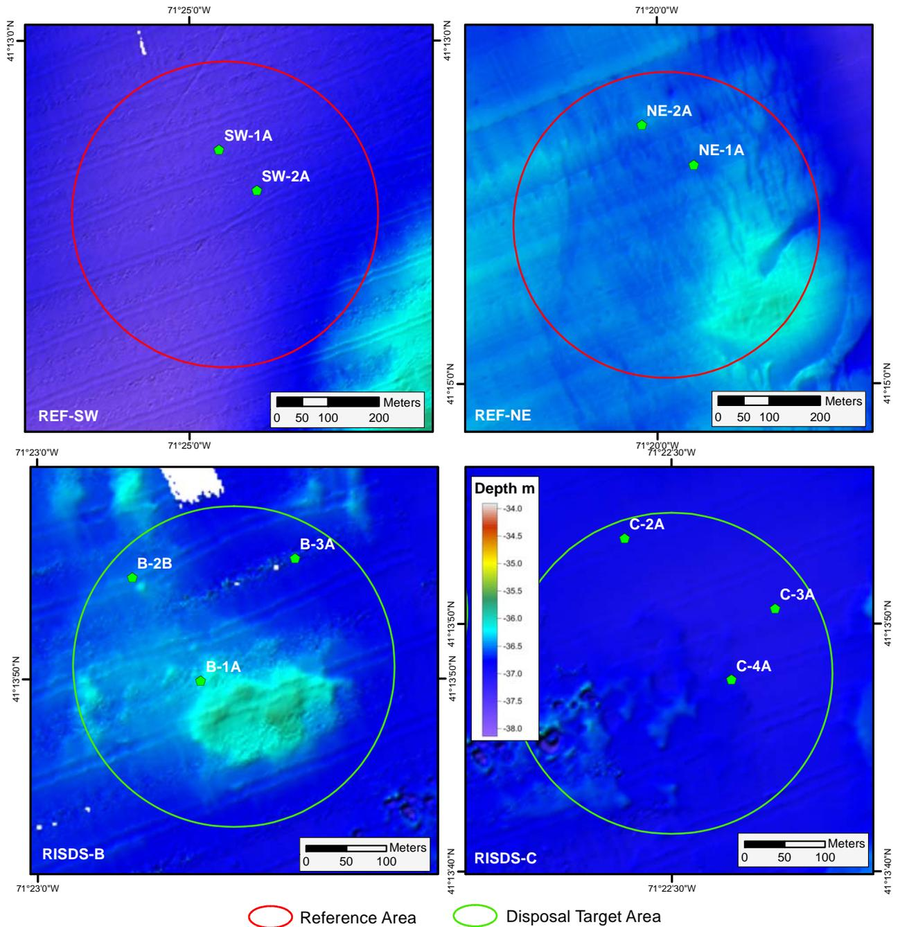
Data: 2008/2009 NOS Bathymetric depth data over acoustic relief model 5x vertical exaggeration.
