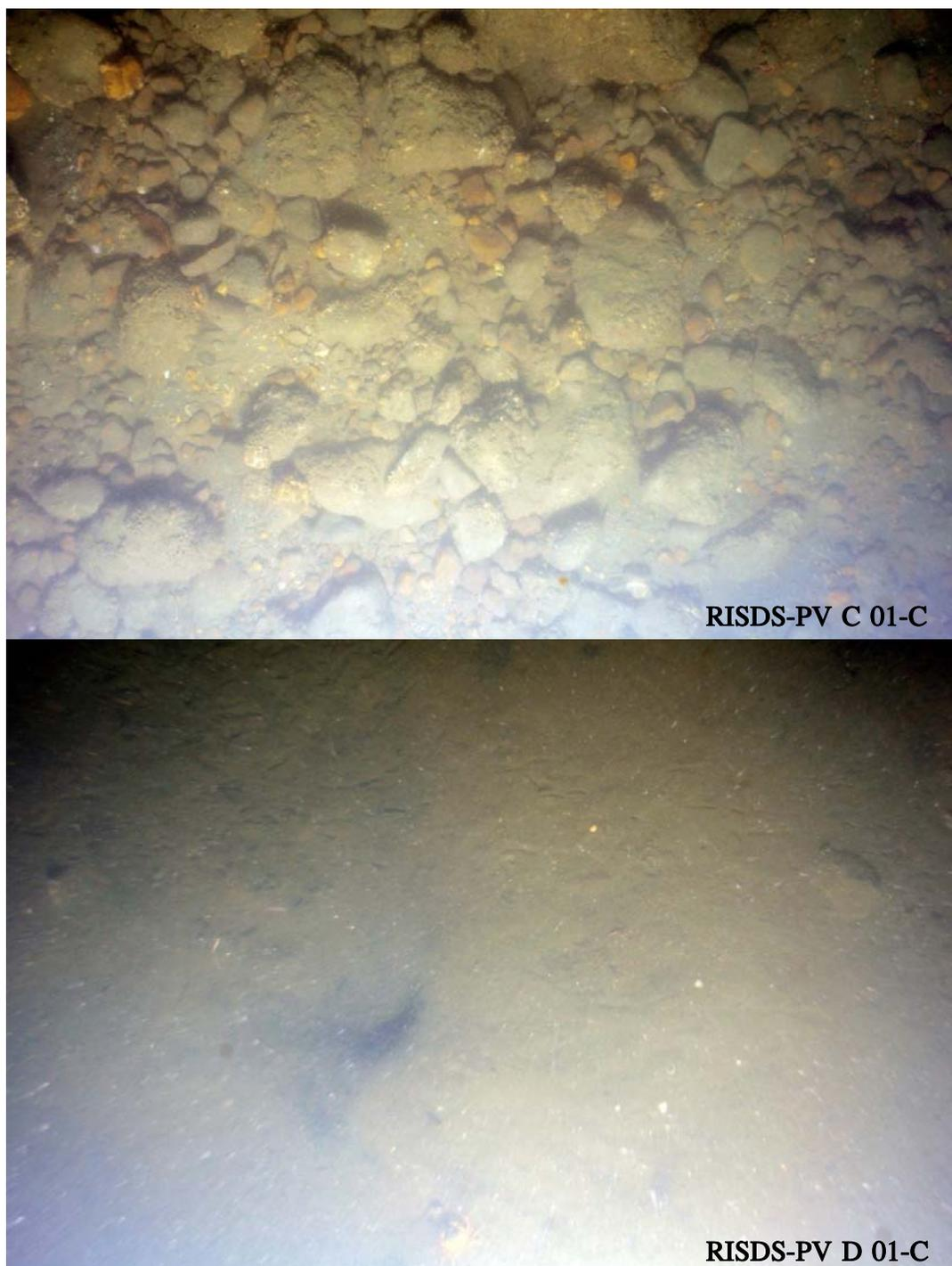
**Figure 3-23.** Plan-view images of sediment surface within the RISDS boundary. Top image is 110 cm across. Bottom image is indeterminate size as laser dots are not clear.
