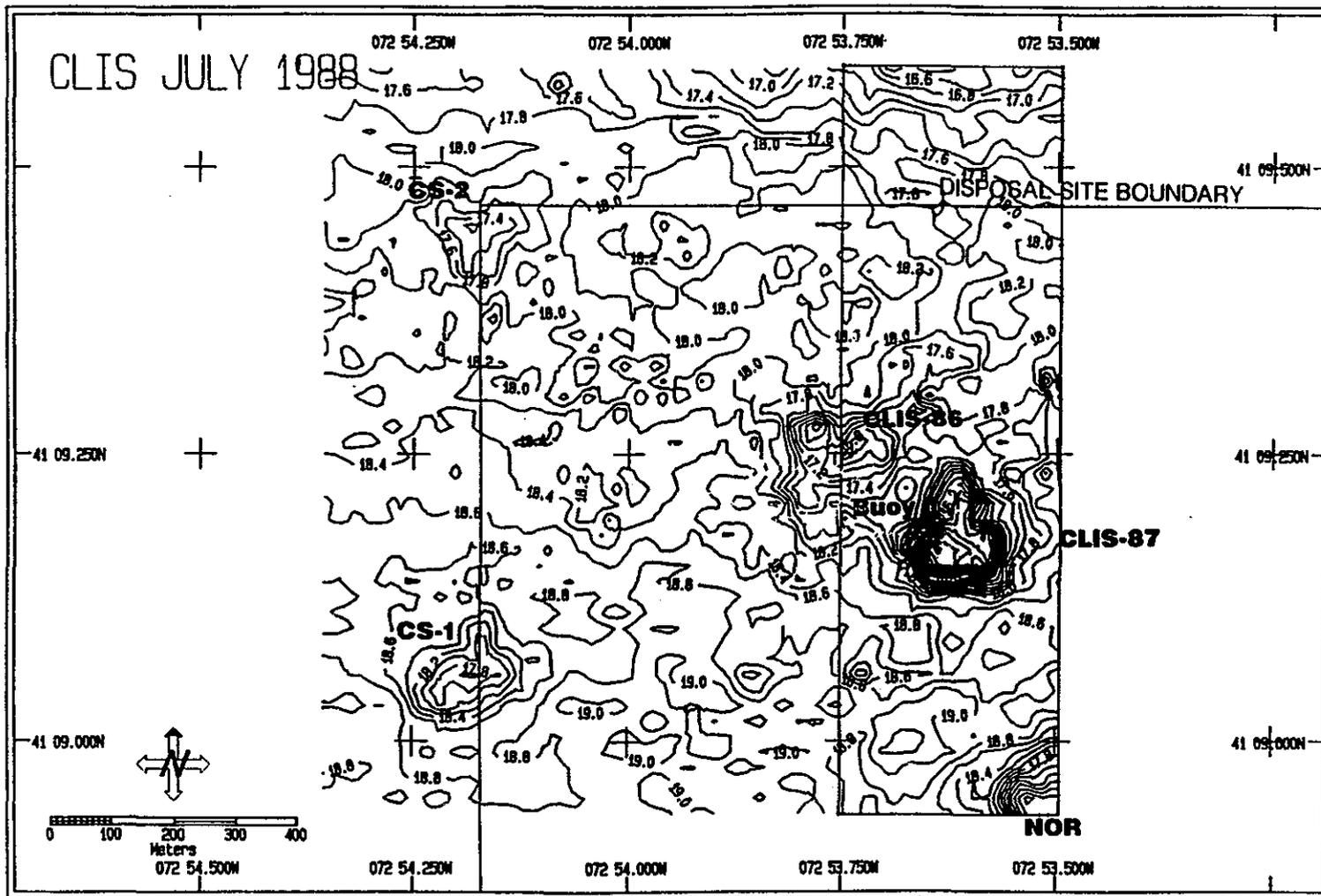
Figure 3-1. Contoured bathymetric chart (depth in meters) of CLIS, 1988. The contour interval is 0.2 m. The area outlined is shown in Figure 3-4.
