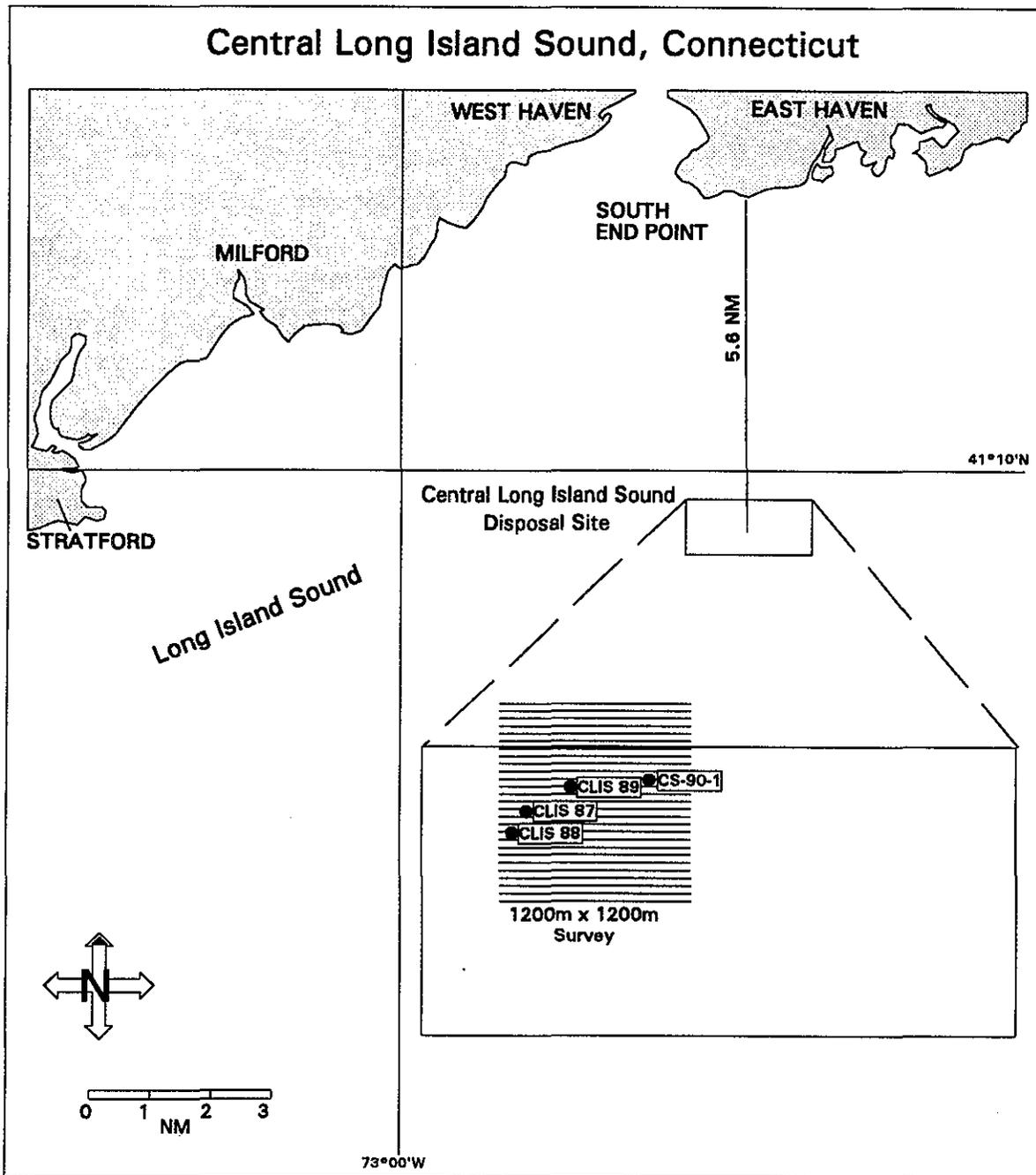
Figure 1-1. Map of bathymetric survey lanes used for the CLIS 1990 survey with the approximate locations of active and inactive disposal mounds
