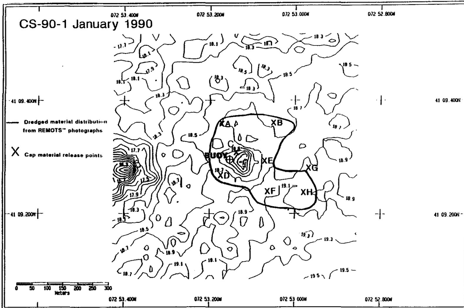
Figure 4-1. Contoured bathymetric chart (depth in meters) of the CS-90-1 disposal mound, January 1990
