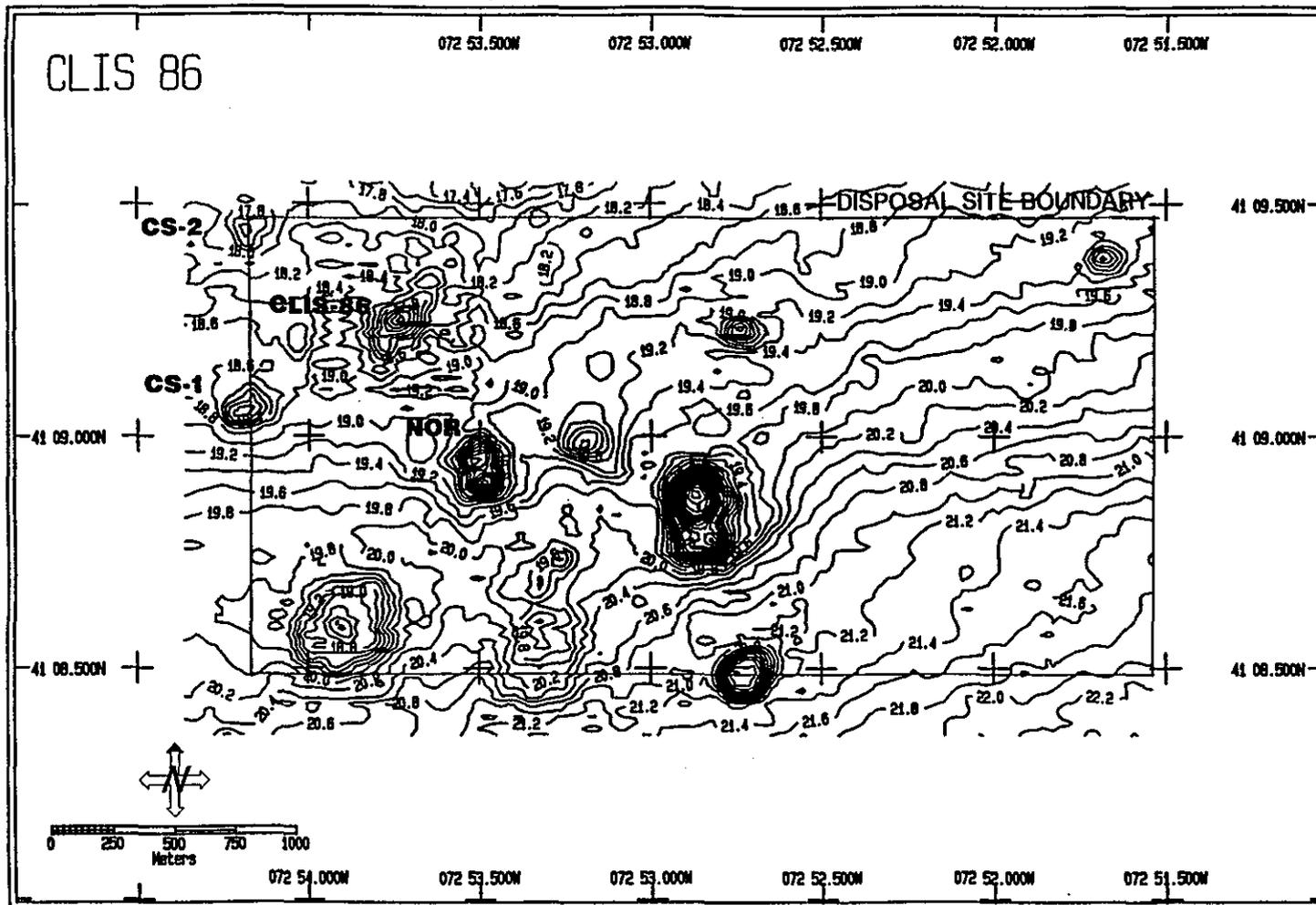
Figure 3-2. Contoured bathymetric chart (depth in meters) of CLIS, 1986. The contour interval is 0.2 m.
