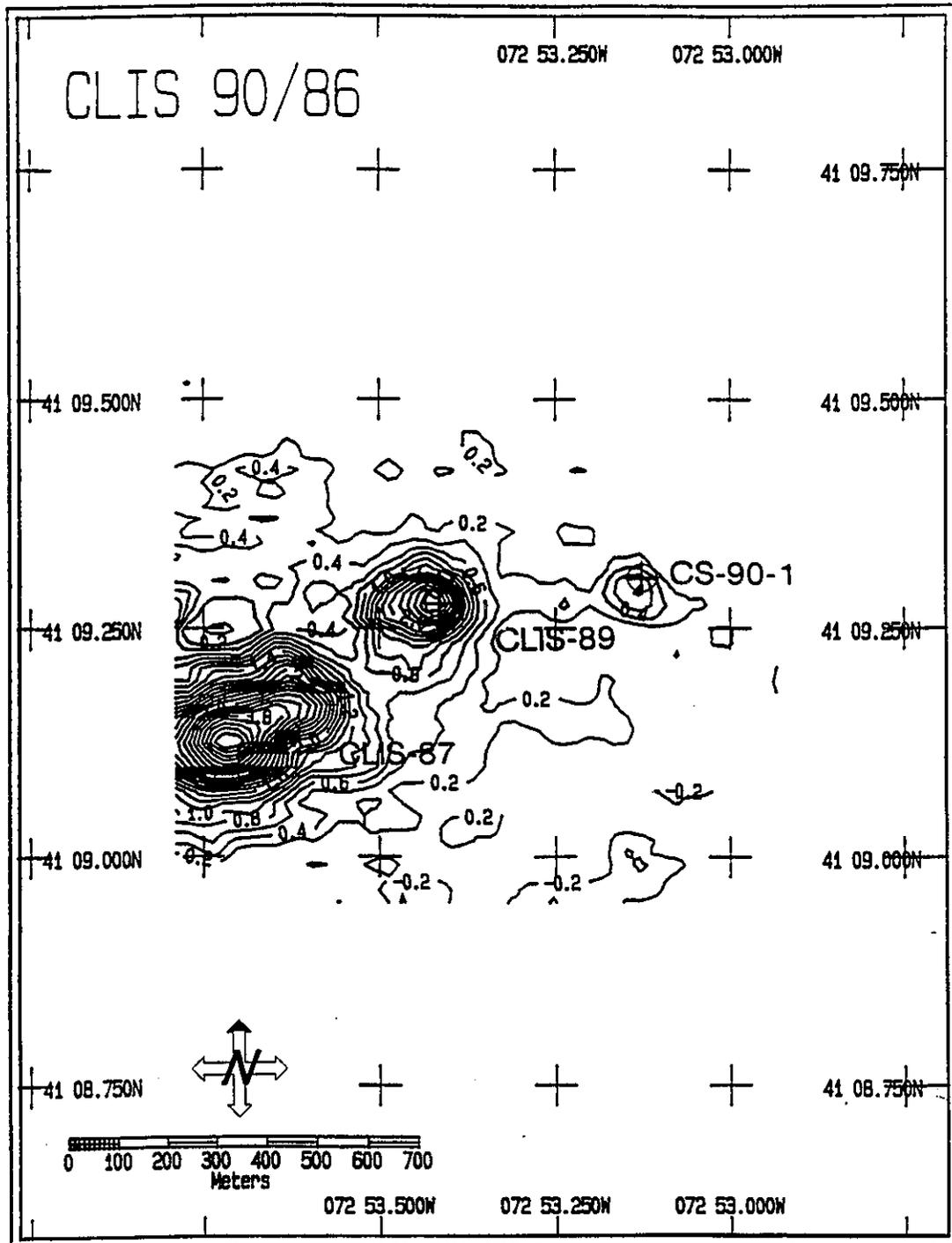
Figure 3-6. Contoured depth difference chart (meters) from 1986 to 1990 surrounding the CLIS-89 and CS-90-1 disposal mounds.
