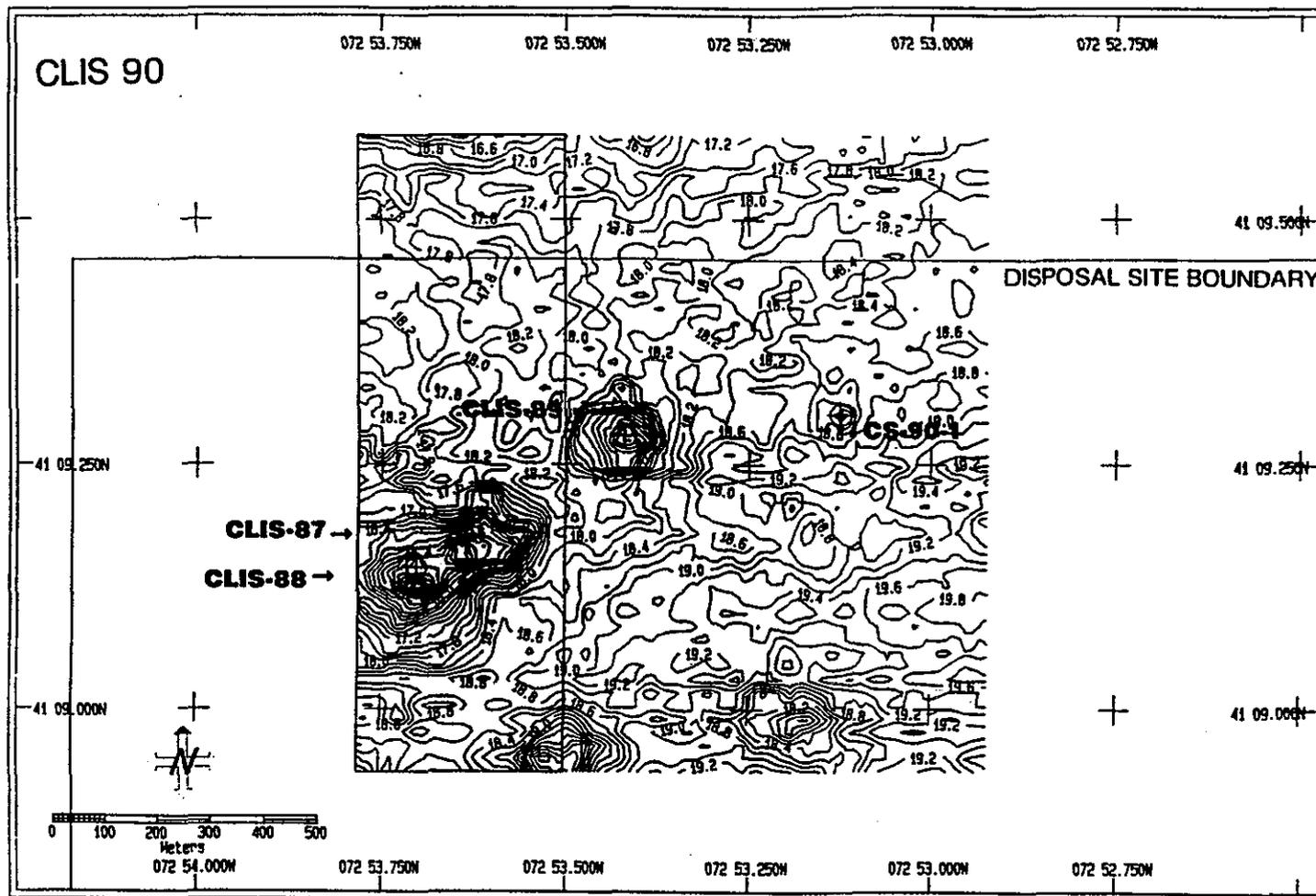
Figure 3-3. Contoured bathymetric chart (depth in meters) of CLIS, 17 and 18 July 1990. The contour interval is 0.2 m. The area outlined is shown in Figure 3-4.
