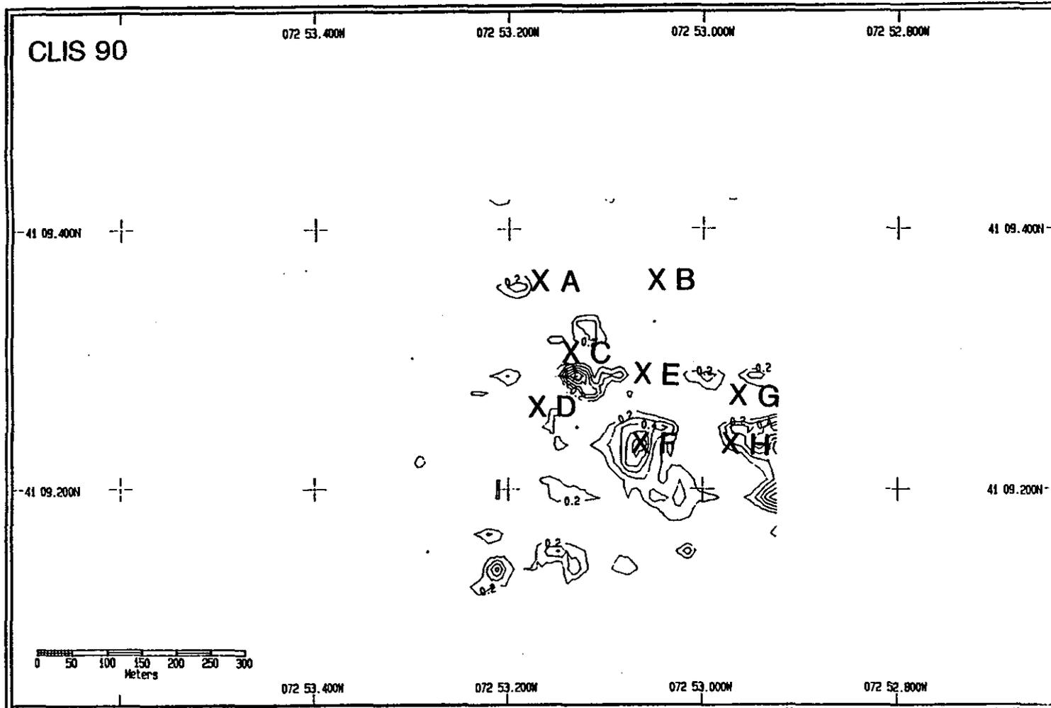
Figure 4-2. Contoured depth difference chart (meters) from January 1990 to July 1990 surrounding the CS-90-1 disposal mound.
