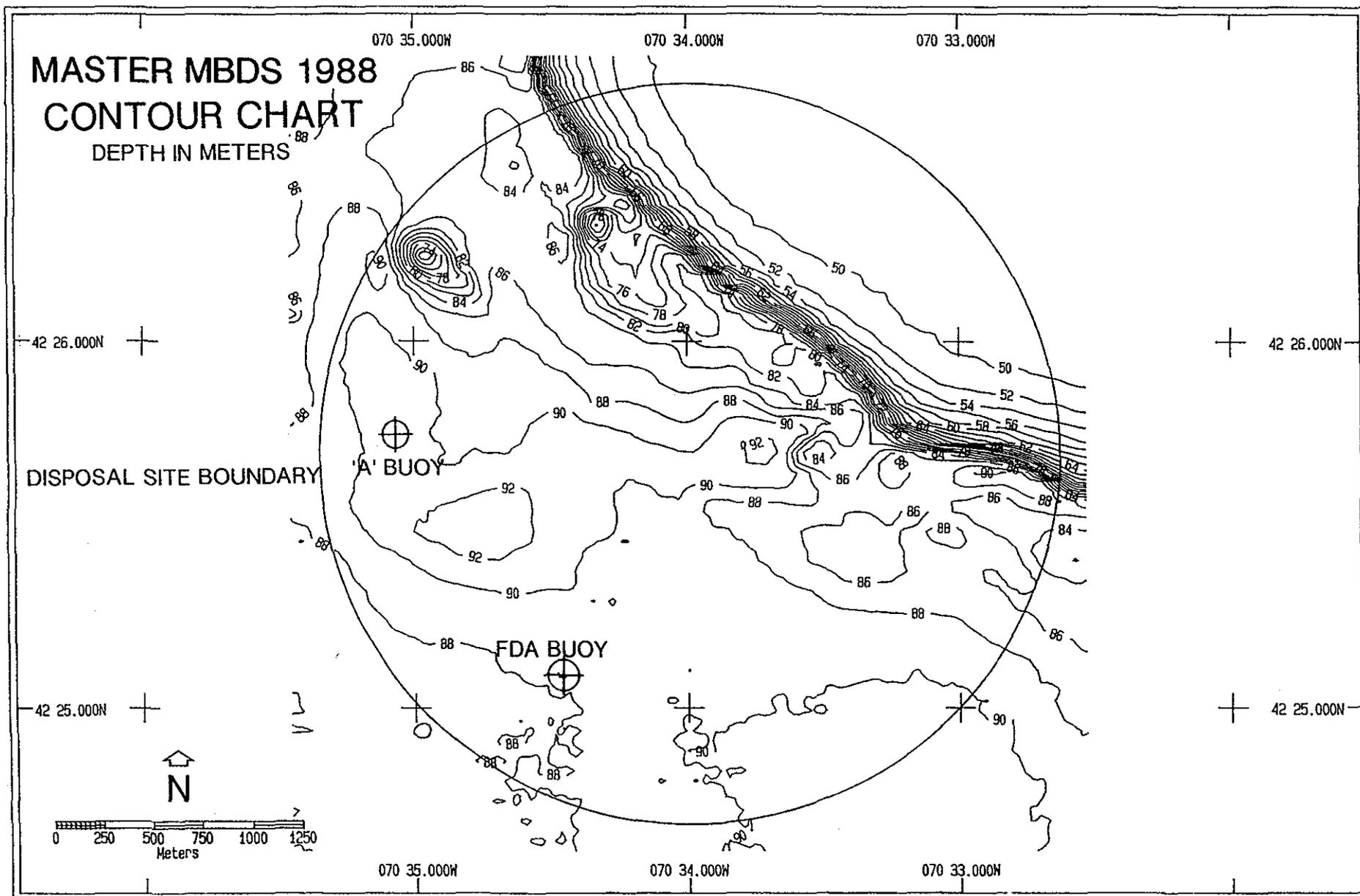
**Figure 3-4.** Bathymetric contour chart of the entire MBDS area, November 1988. Contour interval is 2.0 meters.
