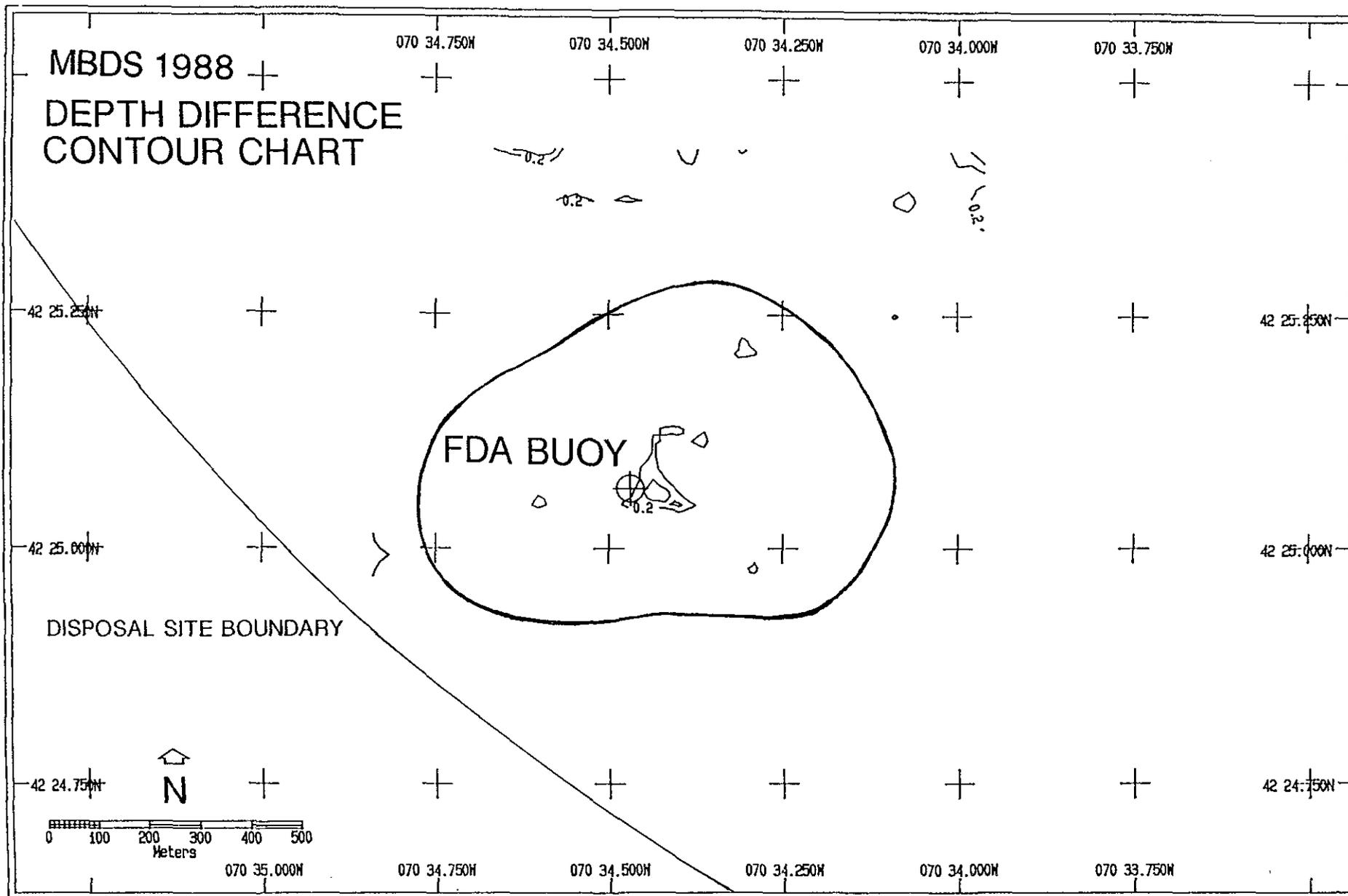
Figure 4-1. Depth difference contour chart with the thick contour line indicating the extent of recently-deposited dredged material around the "FDA" buoy as determined by REMOTS® photography (see Figure 3-6).
