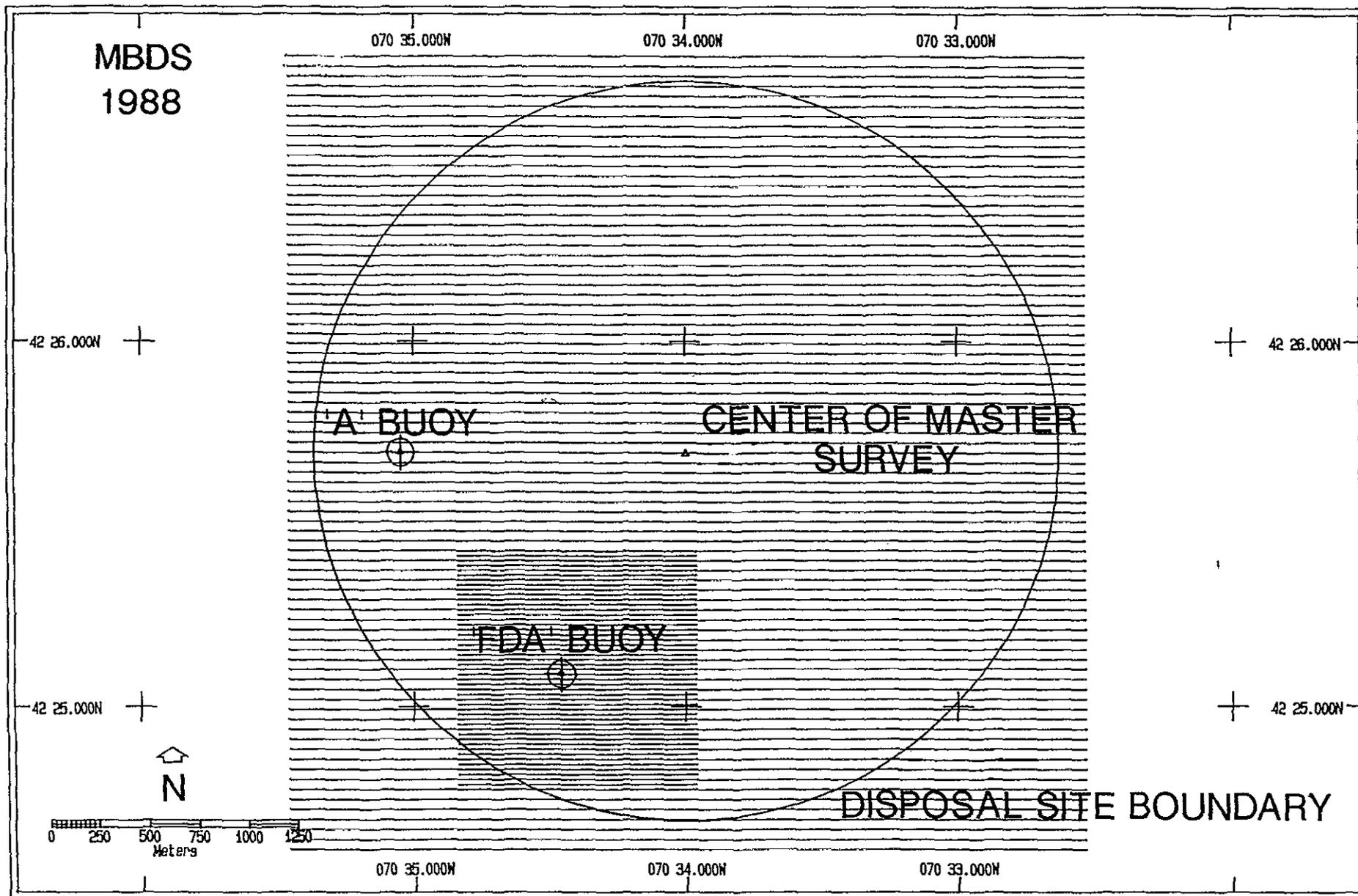
Figure 1-1. Map of bathymetric survey lanes used at MBDS, indicating the location of the "FDA" and "A" buoys, as well as the MASTER MBDS survey encompassing the entire area.
