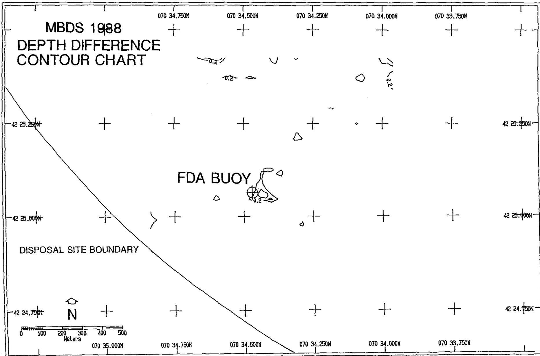
**Figure 3-3.** Depth difference (in meters) contour map based on comparison of the January 1987 and November 1988 precision bathymetric surveys at the "FDA" buoy.
