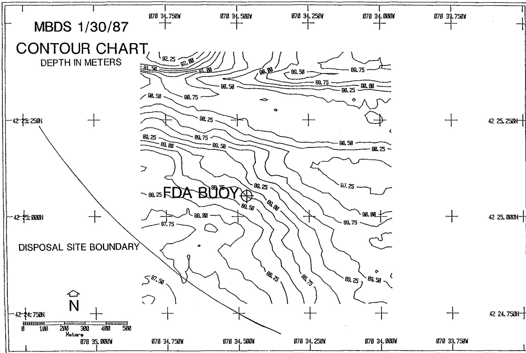
**Figure 3-2.** Bathymetric contour chart of the area surrounding the "FDA" buoy at MBDS, January 1987. The contour interval is 0.25 meters.
