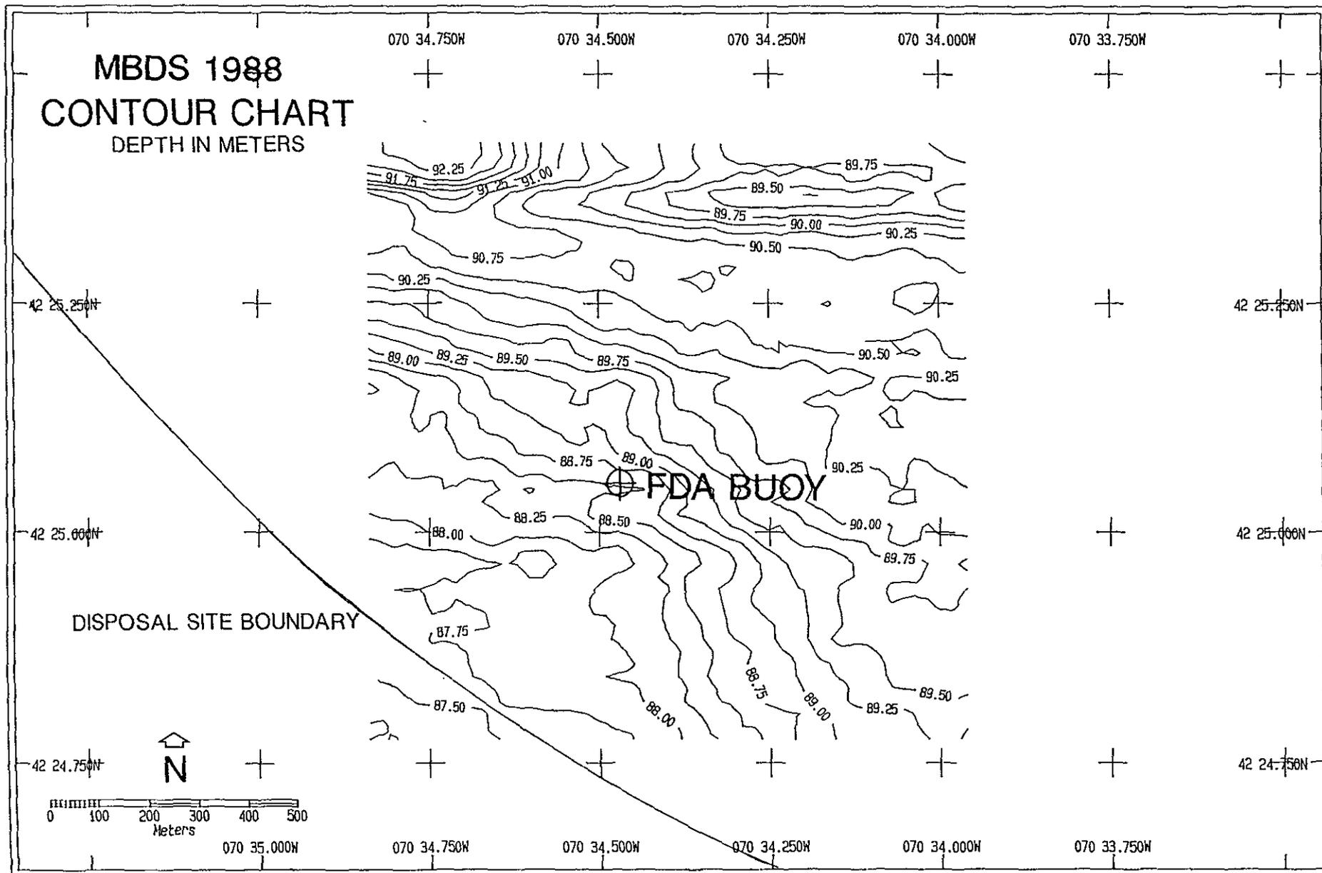
**Figure 3-1.** Bathymetric contour chart of the area surrounding the "FDA" buoy at MBDS, November 1988. The contour interval is 0.25 meters.
