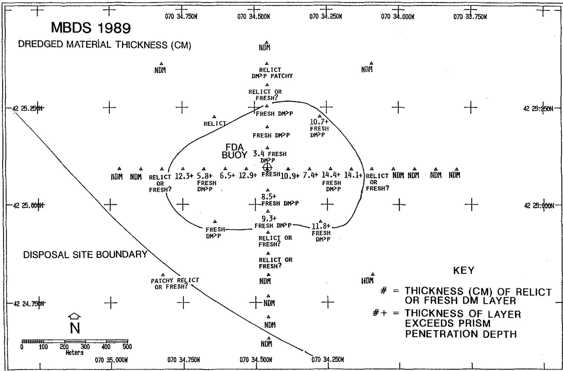
**Figure 3-6.** Map showing the distribution of dredged material based on REMOTS® photography at the "FDA" buoy, January 1989. The contour delimits the extent of dredged material deposited since the January 1987 survey (i.e., "fresh" dredged material).
