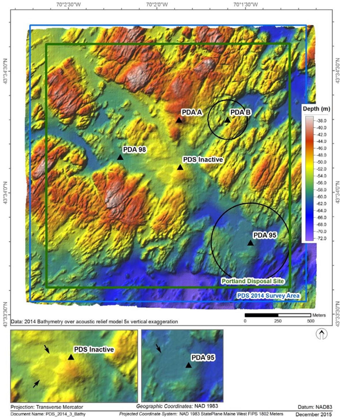
**Figure 3-2.** Bathymetric depth data over acoustic relief model of PDS – August 2014. In insets below figure, arrows indicate patterns consistent with placement of dredged material.
