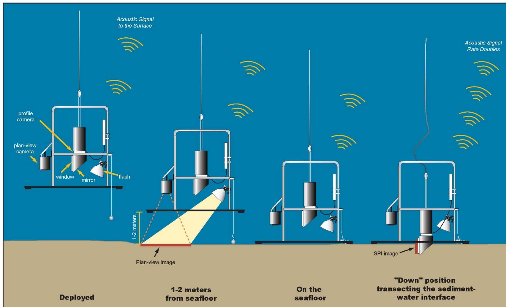
**Figure 2-4.** Schematic diagram of the SPI/PV camera deployment
