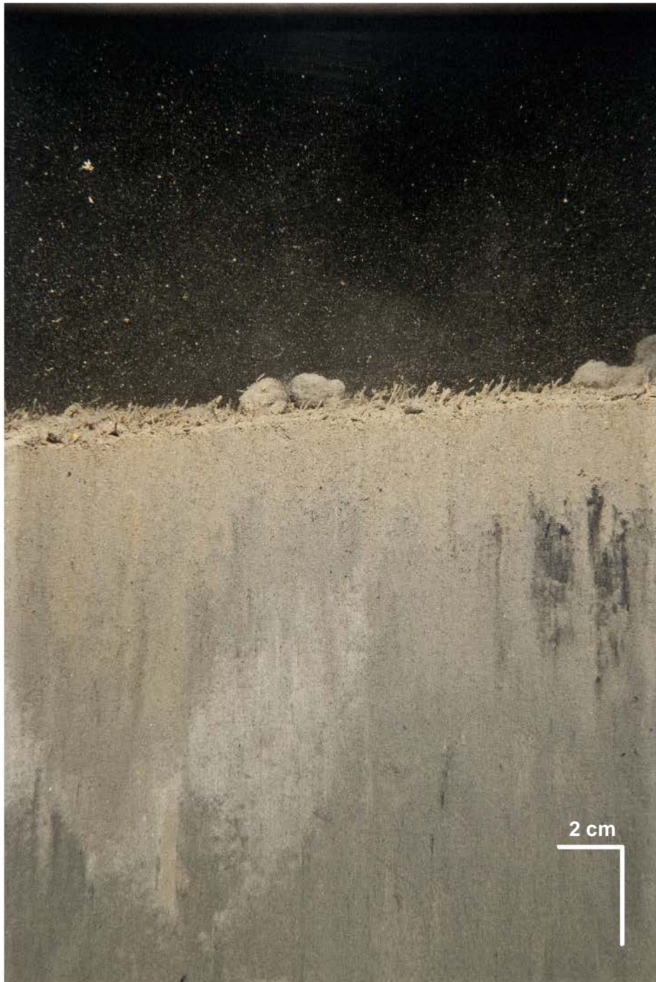
Figure 3-18. Profile image from Mound C Station 2 showing silt/clay dredged material with an oxidized surface layer (i.e., redox layer) overlying relatively light-colored, mottled grey sediment at depth. Clasts on surface are camera artifacts.
