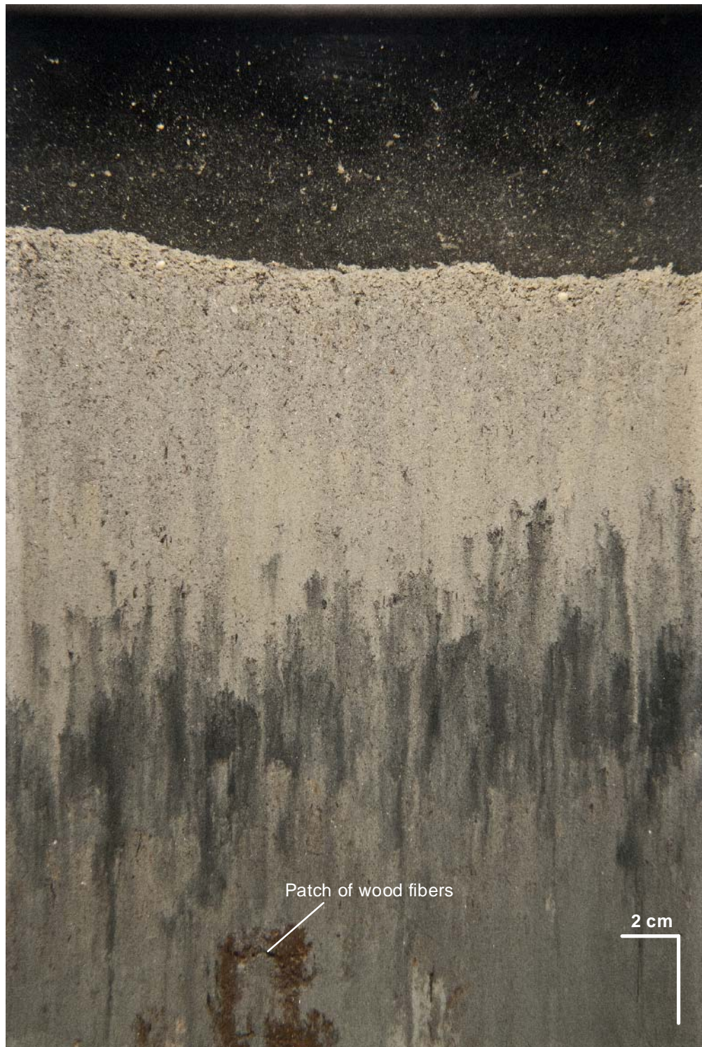
Figure 3-20. Profile image from Mound C Station 4 showing distinct sediment layering and reddish-brown patches of wood fibers at depth.
