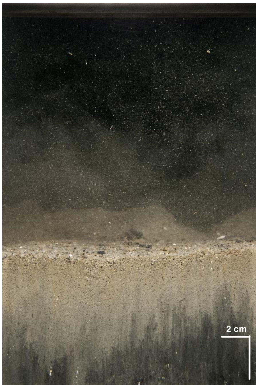
Figure 3-22. Profile image from Station 5 at the apex of Mound C showing a lag deposit of fine sand at the sediment surface overlying reduced, finer-grained sediment at depth.
