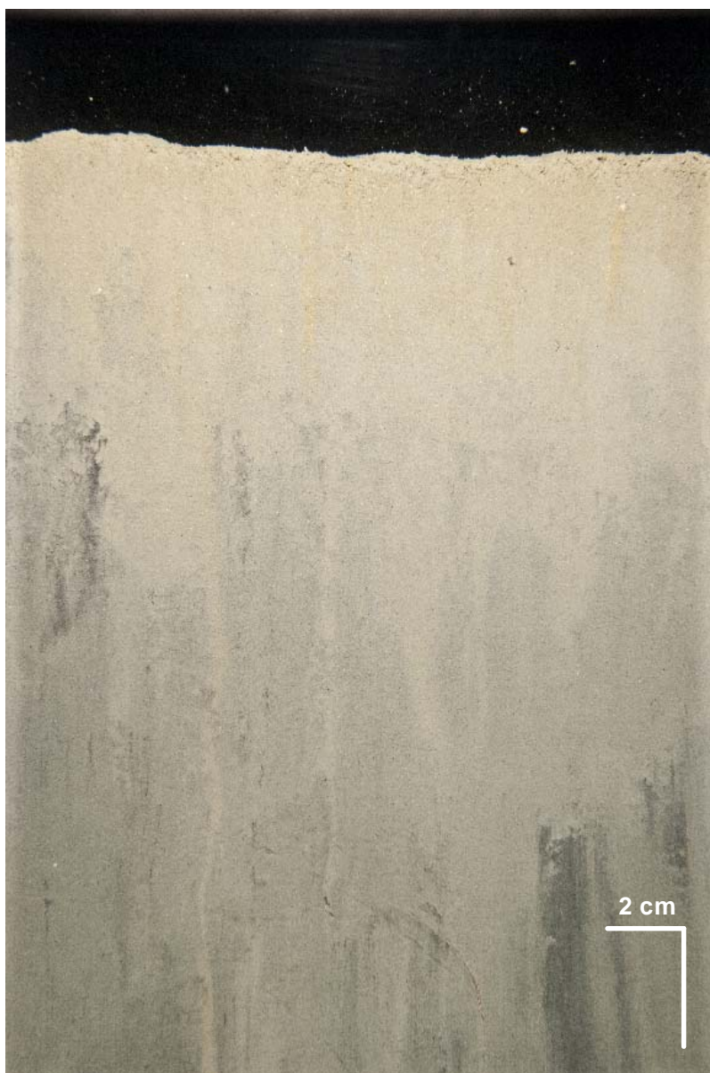
Figure 3-7. Profile image from CCBRS Station 4 showing relatively deep prism penetration in the soft, homogenous silt-clay that typified all three of the reference areas.
