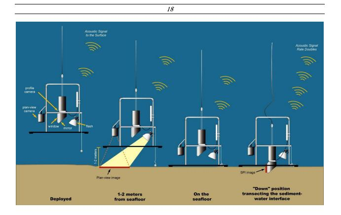
**Figure 2-2.** Operation of the combined Ocean Imaging Model 3731 sediment-profile and Model DSC-6000 plan view cameras
