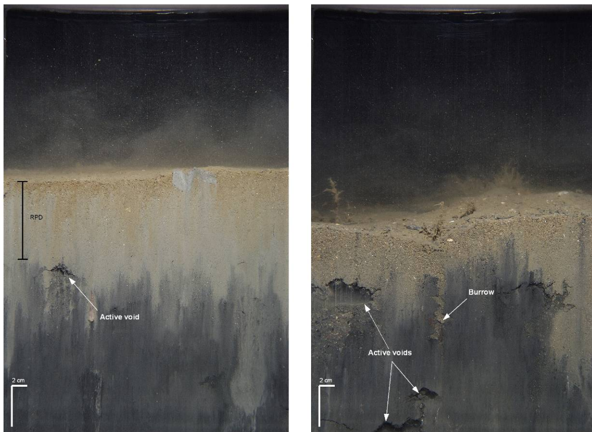
Figure 3-10. SPI images from Stations CLDS04 13 A (left) and CLDS04 07 A (right) at the CLIS 95/96 Mound showing dredged material extending from the sediment surface to below the imaging depth of the SPI camera (i.e., DM thickness > penetration). The dredged material in both images is distinguished by its darker reflectance at depth, indicating higher inventories of organic matter and the presence of reduced sulfides, compared to ambient sediments. Both images also show evidence of extensive surface and sub-surface biological activity, including well-developed RPDs, Stage I tubes, and numerous active Stage III feeding voids and burrows.
