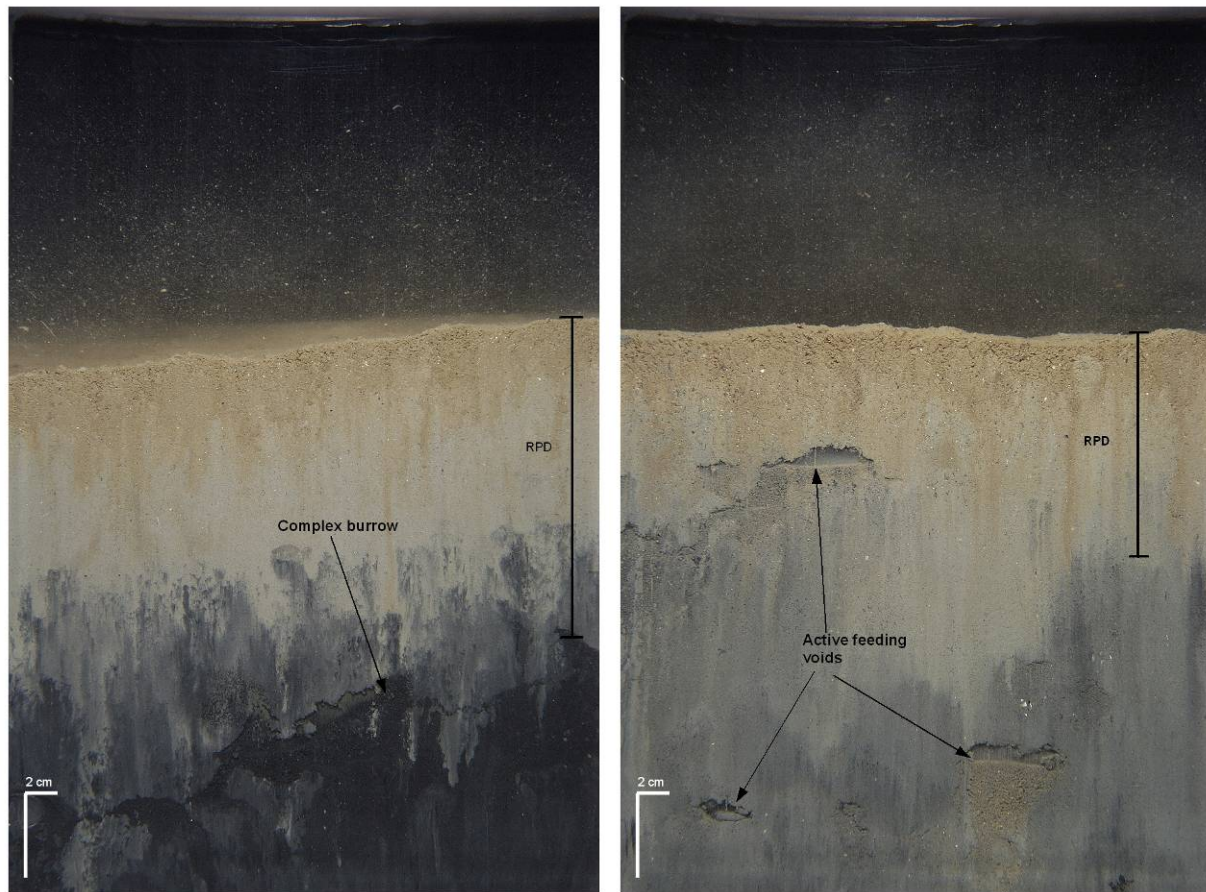
Figure 3-12. SPI images from Stations CLDS04 06 A (left) and CLDS04 03 C (right) illustrating the transition in sediment color from tan/rust at and just below the SWI, to light grey above the apparent RPD, to dark grey or black at depth below the apparent RPD. In both images, the RPD is well-developed (5.3 cm (left) and 3.8 cm (right)), and the sediment surface appears to have a grainier texture due to intensive biological reworking (e.g., tunneling and fecal pellet production). An extensive feeding void complex/burrow is visible in the black subsurface sediment in the left image. Several active, subsurface feeding voids are visible in the right image. Note the oxidized sediment that has been subducted and comprises the floor of the feeding void at right.
