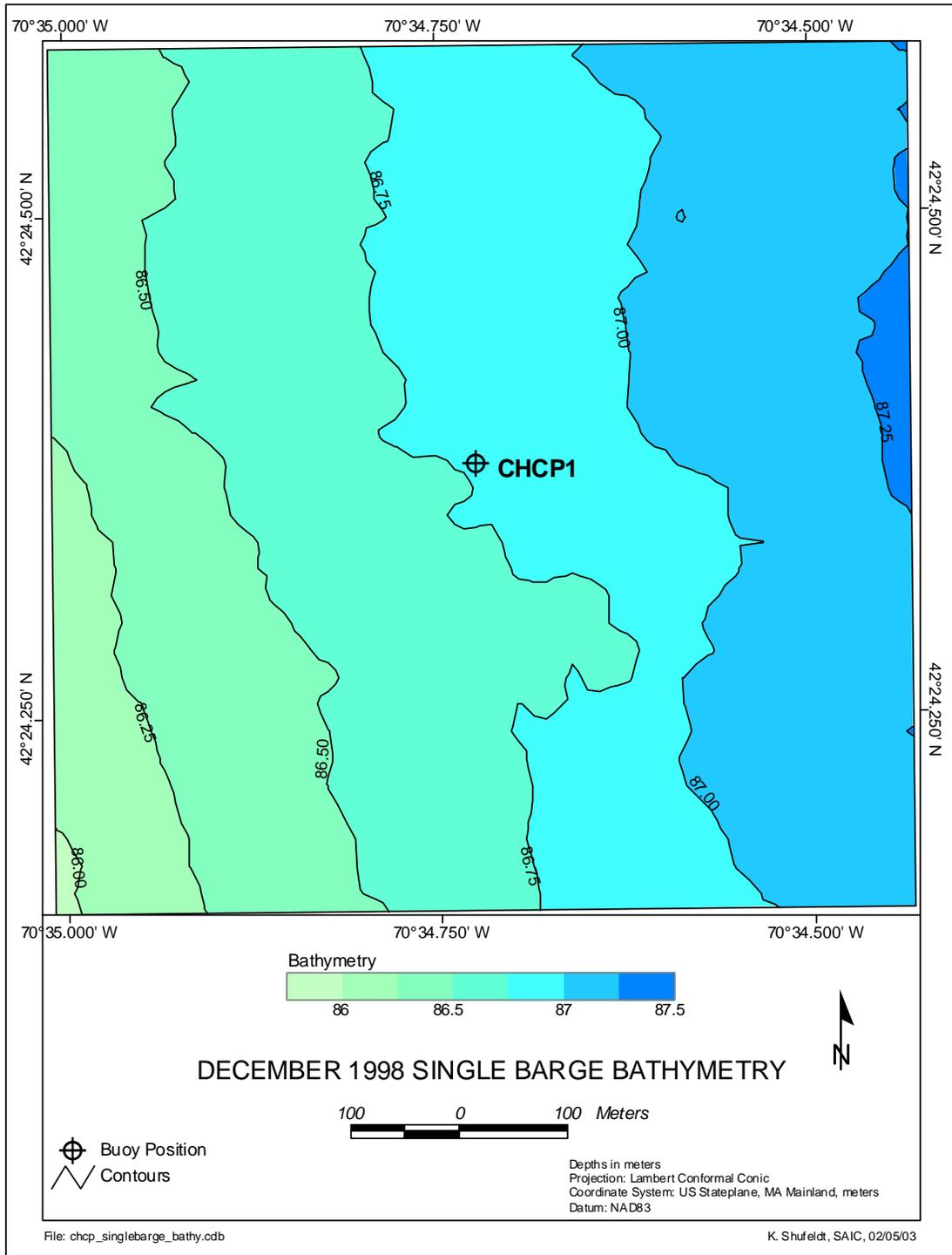
**Figure 3-9.** Bathymetric chart of the 800 × 800 m CHCP study area during the December 1998 Single-Barge survey, 0.25 m contour interval
