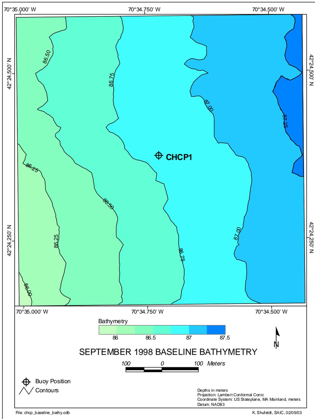
**Figure 3-1.** Bathymetric chart of the 800 × 800 m CHCP study area during the September 1998 Baseline survey, 0.25 m contour interval
