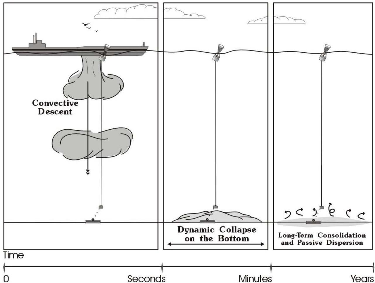
**Figure 4-1.** Schematic diagram of the three phases of descent encountered during a dredged material disposal event
