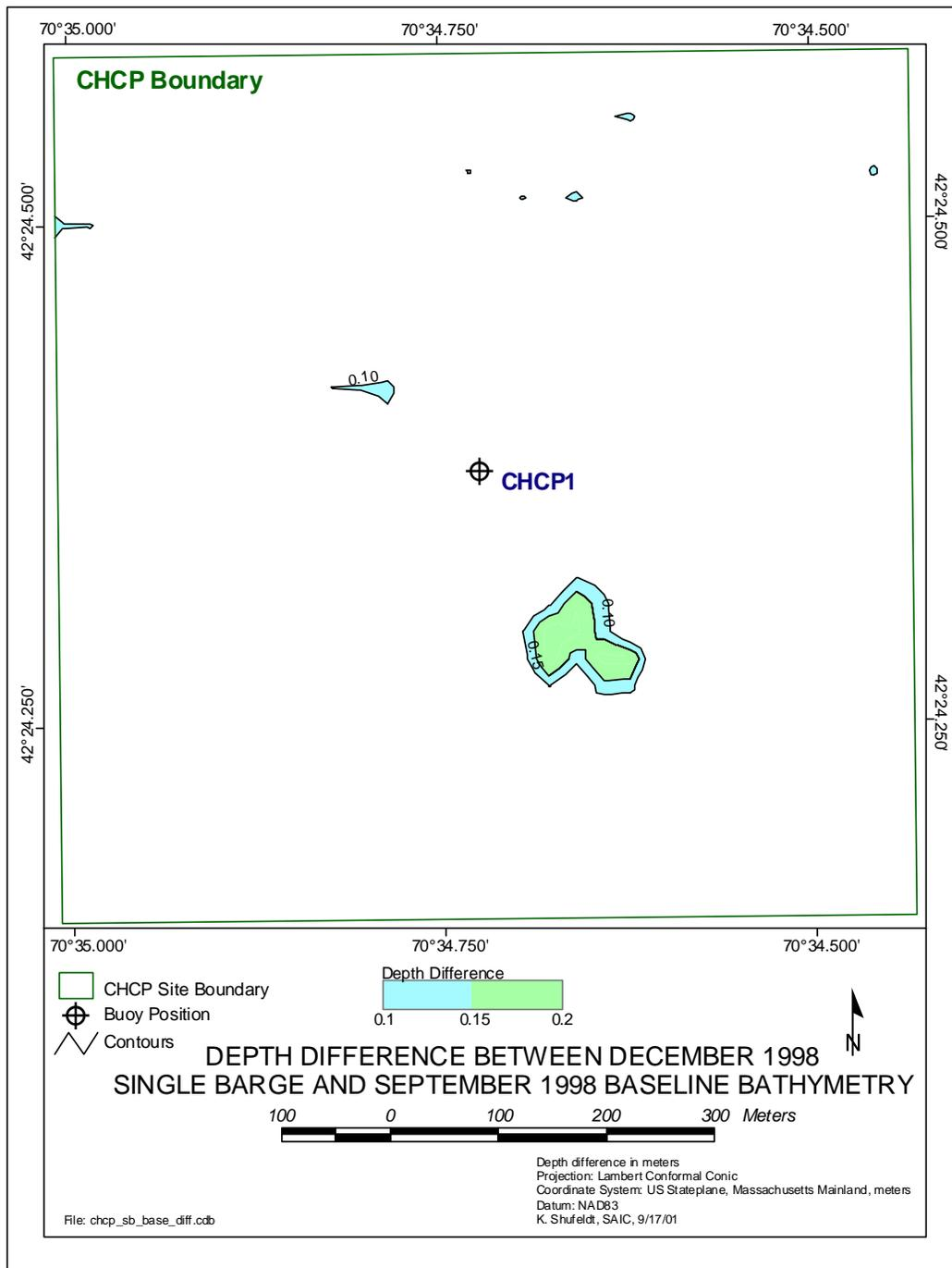
**Figure 3-10.** Depth difference comparisons between the December 1998 Single-Barge and September 1998 Baseline bathymetric surveys showing the accumulation of dredged material within the CHCP study area
