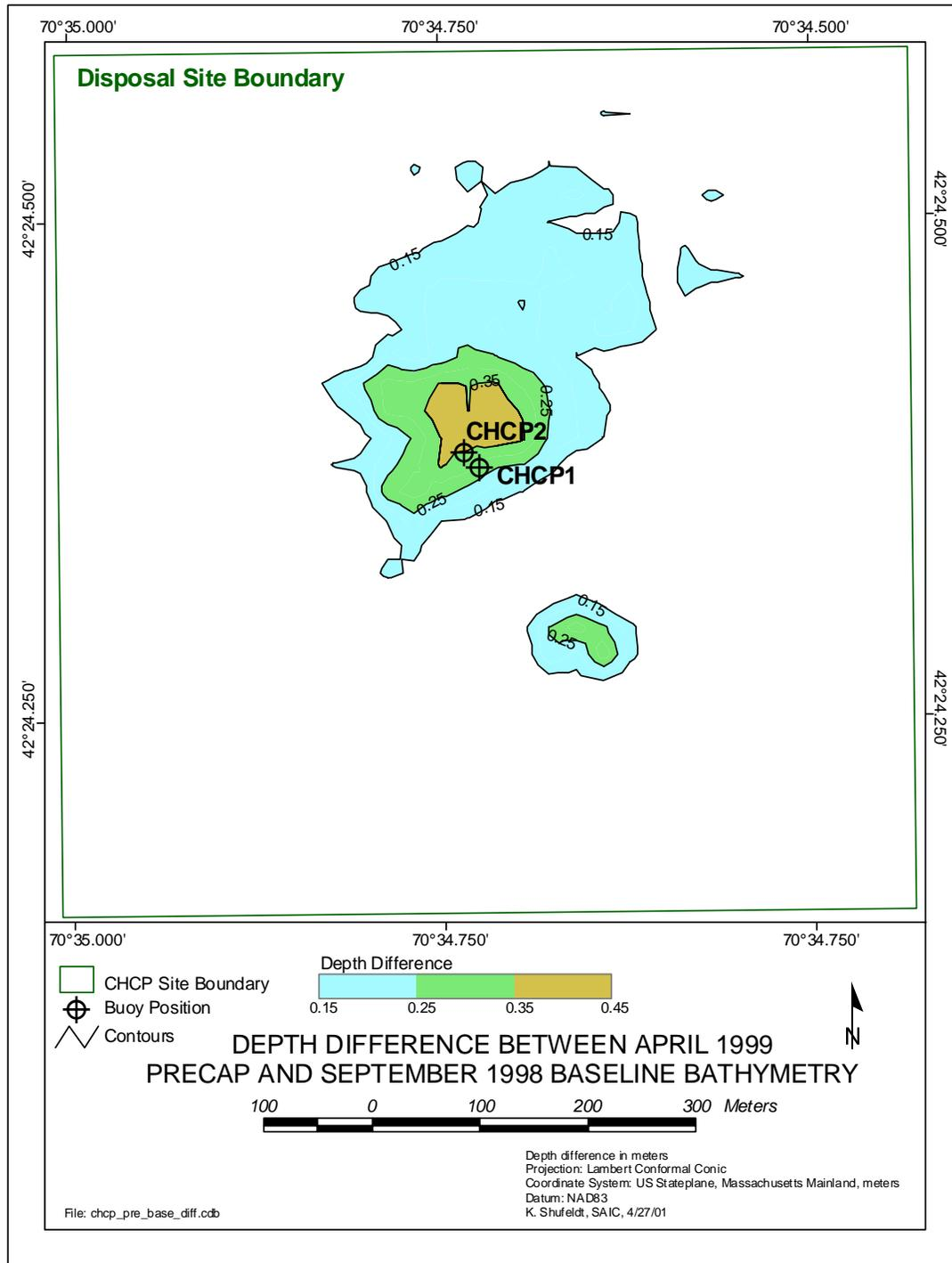
**Figure 3-21.** Depth difference comparison between the April 1999 Precap and September 1998 Baseline bathymetric surveys showing total accumulation of dredged material within the CHCP study area
