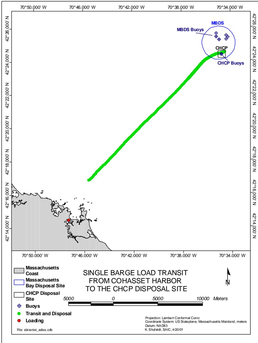
**Figure 2-5.** A graphical example of a typical ADISS data file documenting an entire trip of a disposal barge transiting from Cohasset Harbor to the CHCP study area
