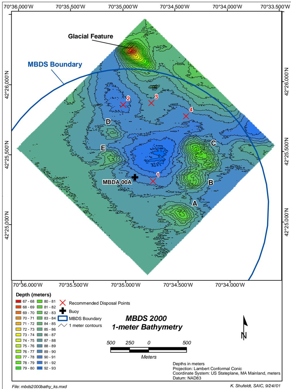
**Figure 4-11.** Bathymetric chart of the northeastern quadrant of MBDS showing disposal mounds A through E, the current MBDA buoy location (MBDA 00A), as well as future recommended disposal points (1-4) to complete the first artificial containment cell on the MBDS seafloor
