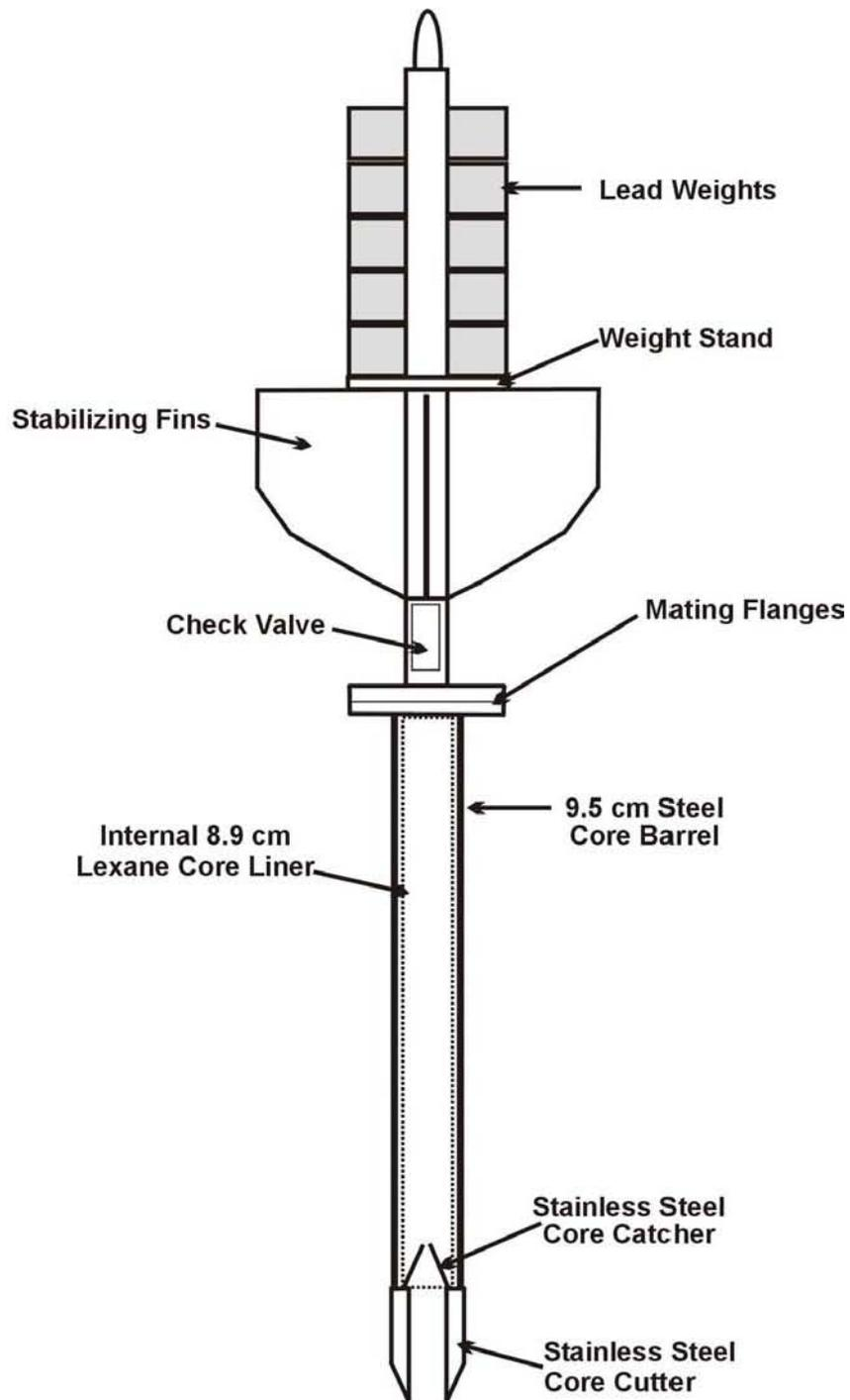
**Figure 2-12.** Schematic drawing of the SAIC gravity coring device employed as part of the Postcap survey efforts over the CHCP study area
