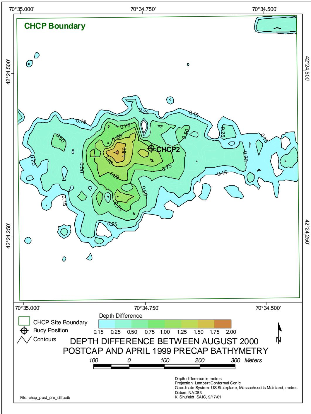
**Figure 3-31.** Depth difference comparison between the August 2000 Postcap and April 1999 Precap bathymetric surveys showing the distribution and thickness of CDM within the CHCP study area, 0.15 m base contour
