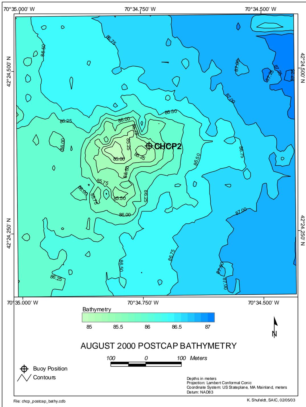
**Figure 3-29.** Bathymetric chart of the 800 × 800 m CHCP study area during the August 2000 Postcap survey, 0.25 m contour interval
