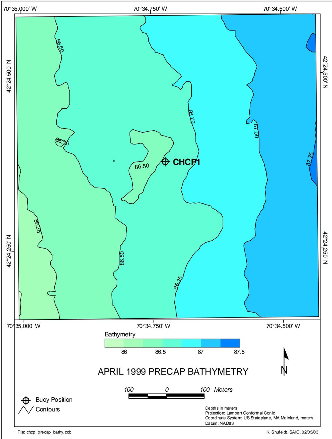
**Figure 3-20.** Bathymetric chart of the 800 × 800 m CHCP study area during the April 1999 Precap survey, 0.25 m contour interval
