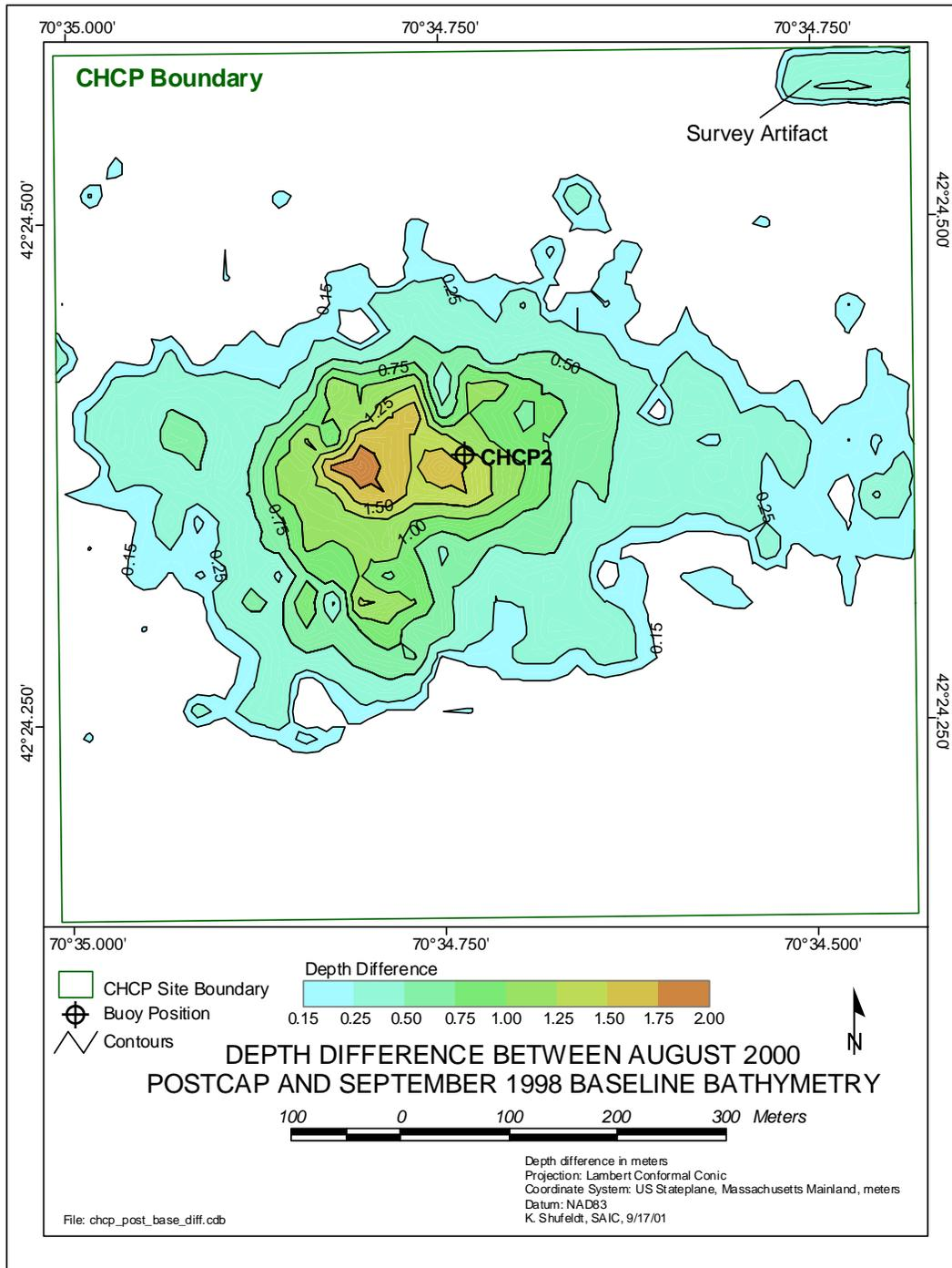
**Figure 3-30.** Depth difference comparison between the August 2000 Postcap and the September 1998 Baseline bathymetric surveys showing the morphology of the CHCP Mound on the MBDS seafloor, 0.15 m base contour
