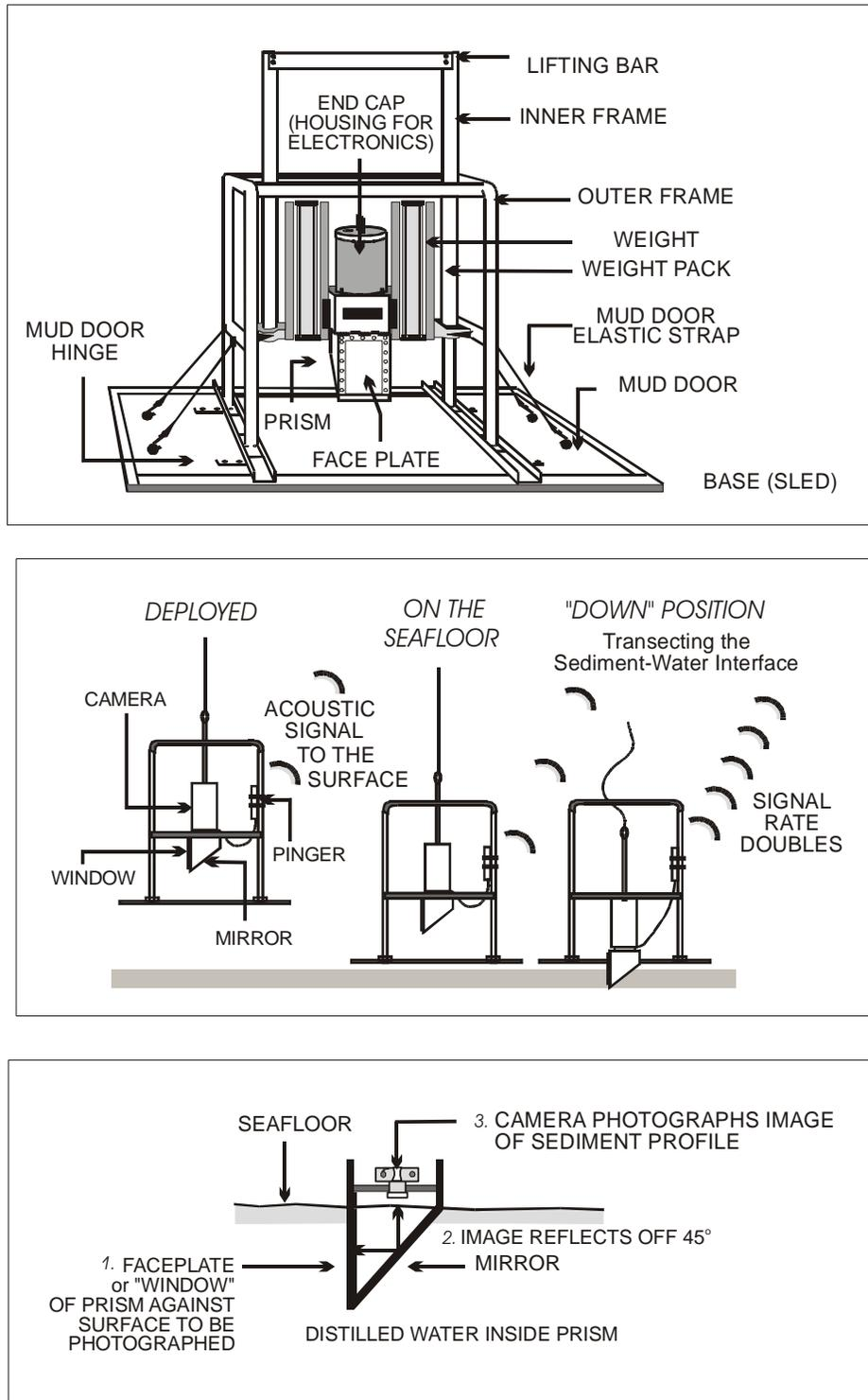
**Figure 2-8.** Schematic diagram of the Benthos, Inc. Model 3731 REMOTS<sup>®</sup> sediment-profile camera and sequence
