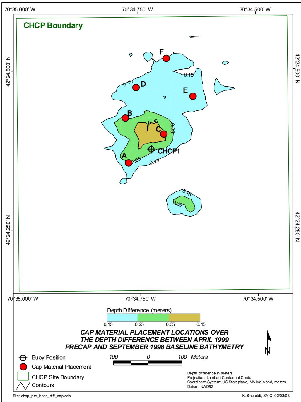
**Figure 4-7.** Graphic illustrating the potential location of capping points over the UDM mound for the placement of CDM to facilitate the development of an even sediment cap to a desired thickness
