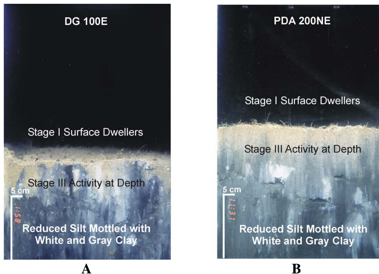
Figure 4-1. REMOTS® images collected from Station 100E over the DG Mound (A) and Station 200NE over the PDA 98 Mound (B) displaying strong similarities in sediment appearance, composition, and benthic recolonization
