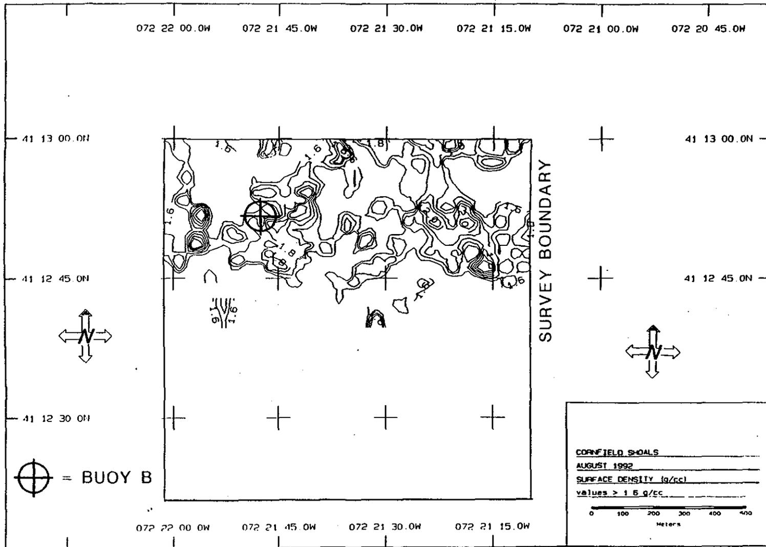
Figure 3-11. Surface sediment density values  $>1.6 \text{ g}\cdot\text{cc}^{-1}$
