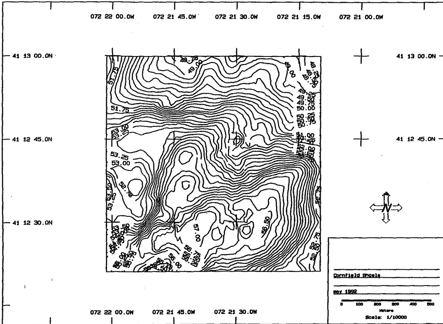
Figure 3-1. Bathymetric contour plot at the Cornfield Shoals Disposal Site, May 1992 (depth in meters)
