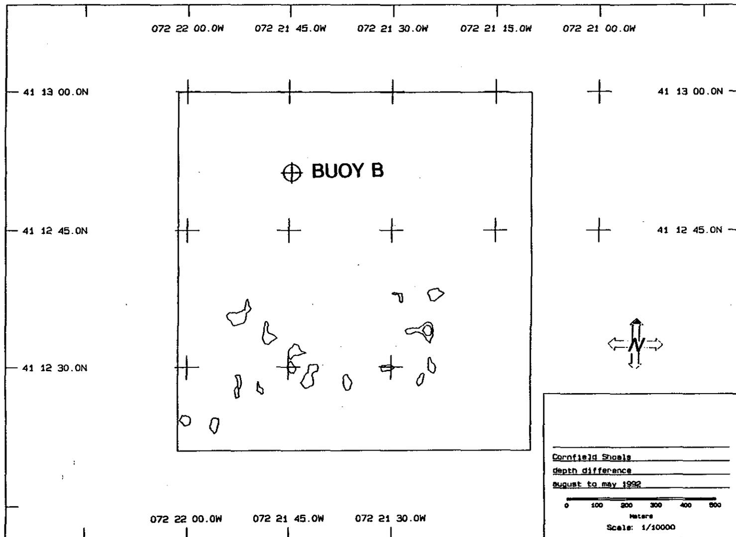
Figure 3-4. Positive depth difference contour plot between May 1992 and August 1992 (contours at 0.2 and 0.4 m)
