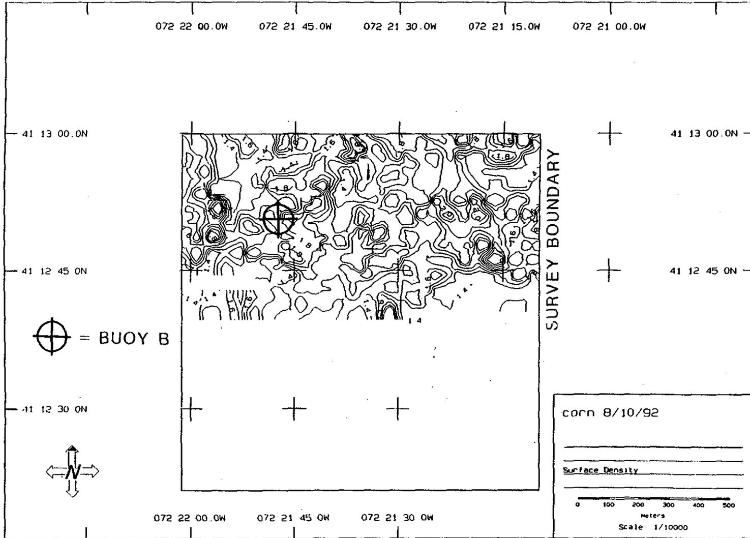
Figure 3-10. Contour plot of surface sediment density ( $\text{g}\cdot\text{cc}^{-1}$ ) at the Cornfield Shoals Disposal Site, August 1992.
