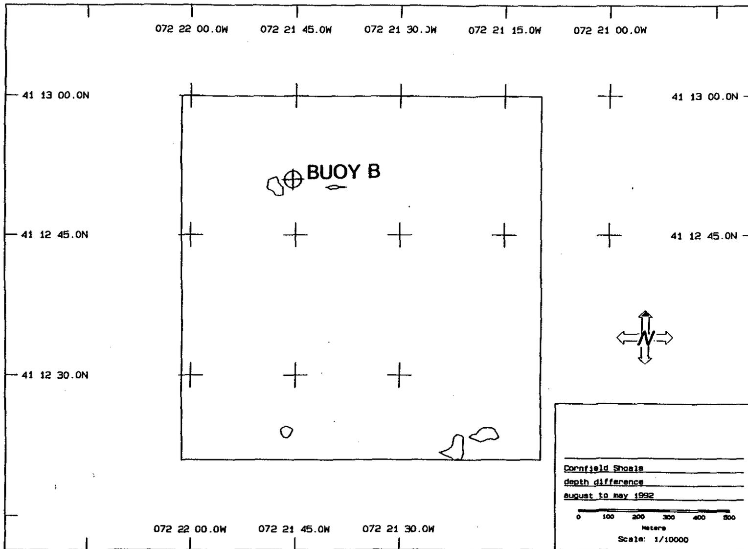
Figure 3-3. Negative depth difference contour plot between May 1992 and August 1992 (contours at 0.2 m)
