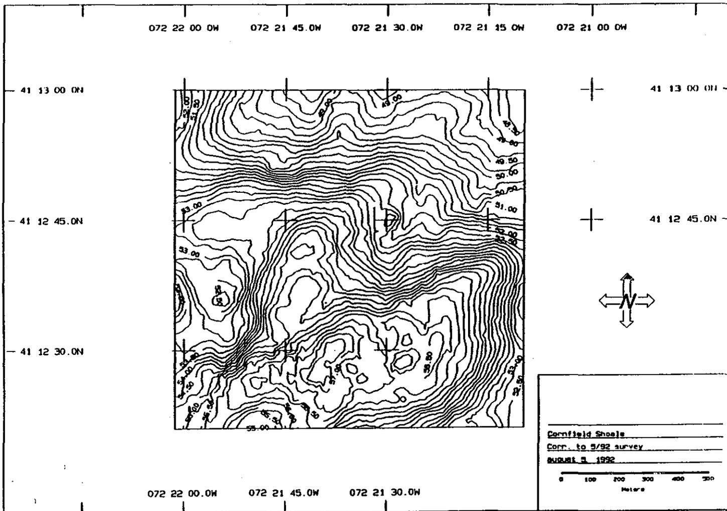
Figure 3-2. Bathymetric contour plot at the Cornfield Shoals Disposal Site, August 1992 (depth in meters)
