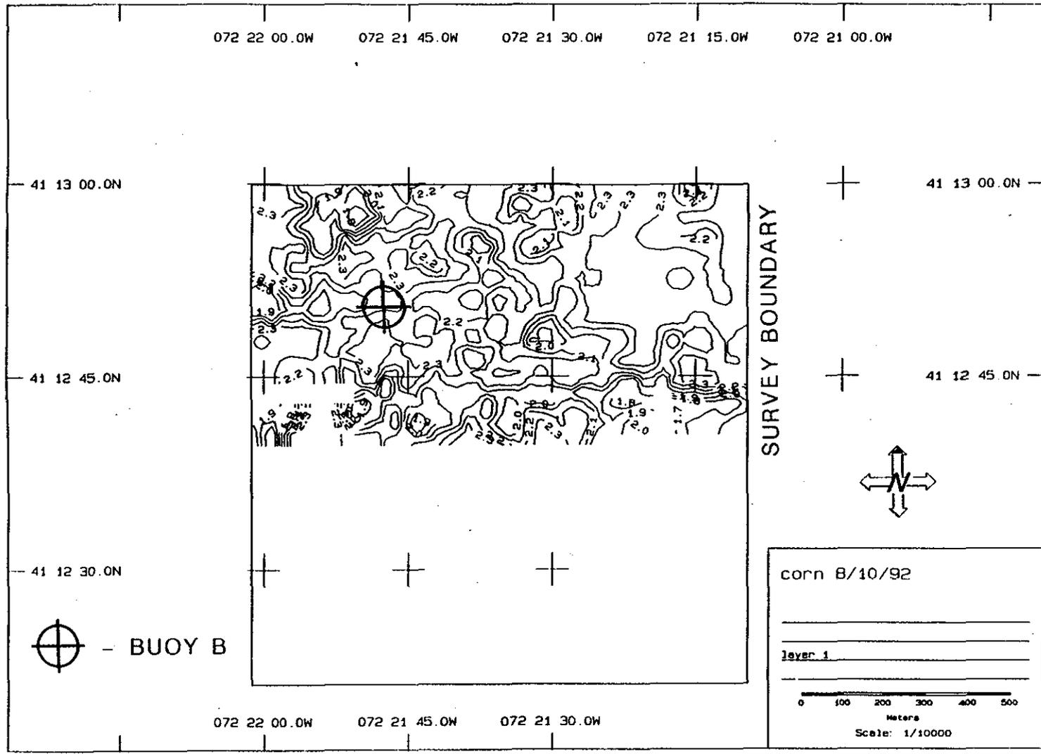
Figure 3-12. Sediment density ( $\text{g}\cdot\text{cc}^{-1}$ ) at the Cornfield Shoals Disposal Site, approximately 15 cm below the sediment surface
