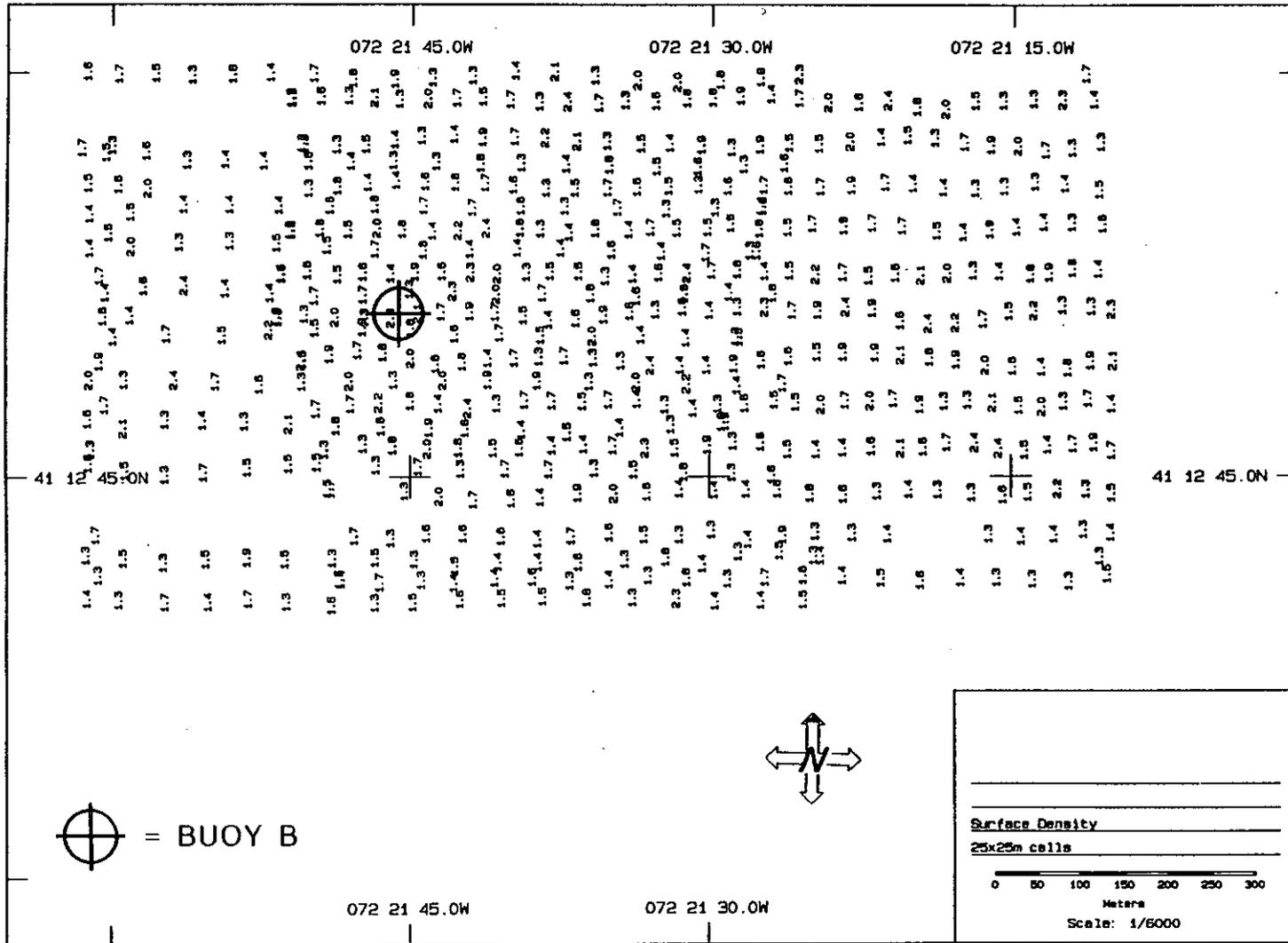
Figure 3-9. Smooth sheet of surface sediment density ( $\text{g}\cdot\text{cc}^{-1}$ ) at the Cornfield Shoals Disposal Site, August 1992
