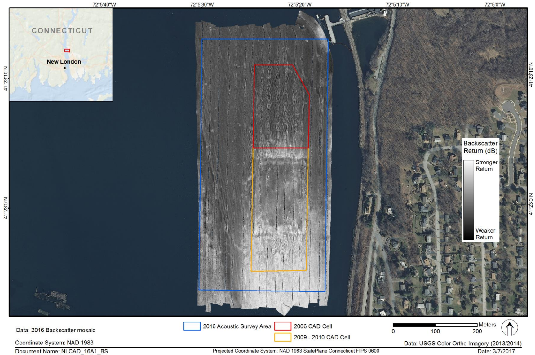
Figure 3-4. Mosaic of unfiltered backscatter data of NLCAD Cell Site – November 2016
