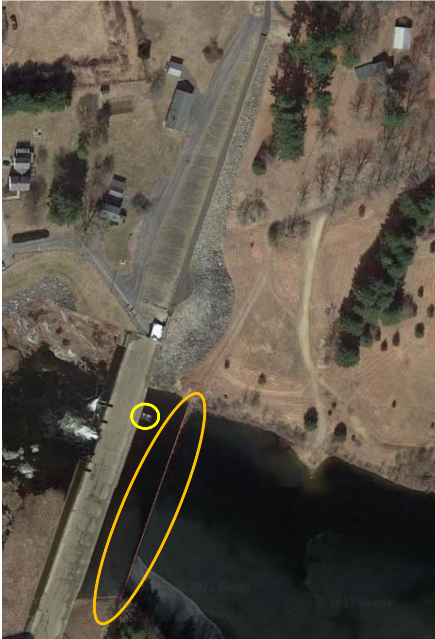
Map 1: Image showing Mansfield Hollow Dam inlet area. Orange log boom (orange circle) and weir box structure (yellow circle) is visible in bottom left of image.
