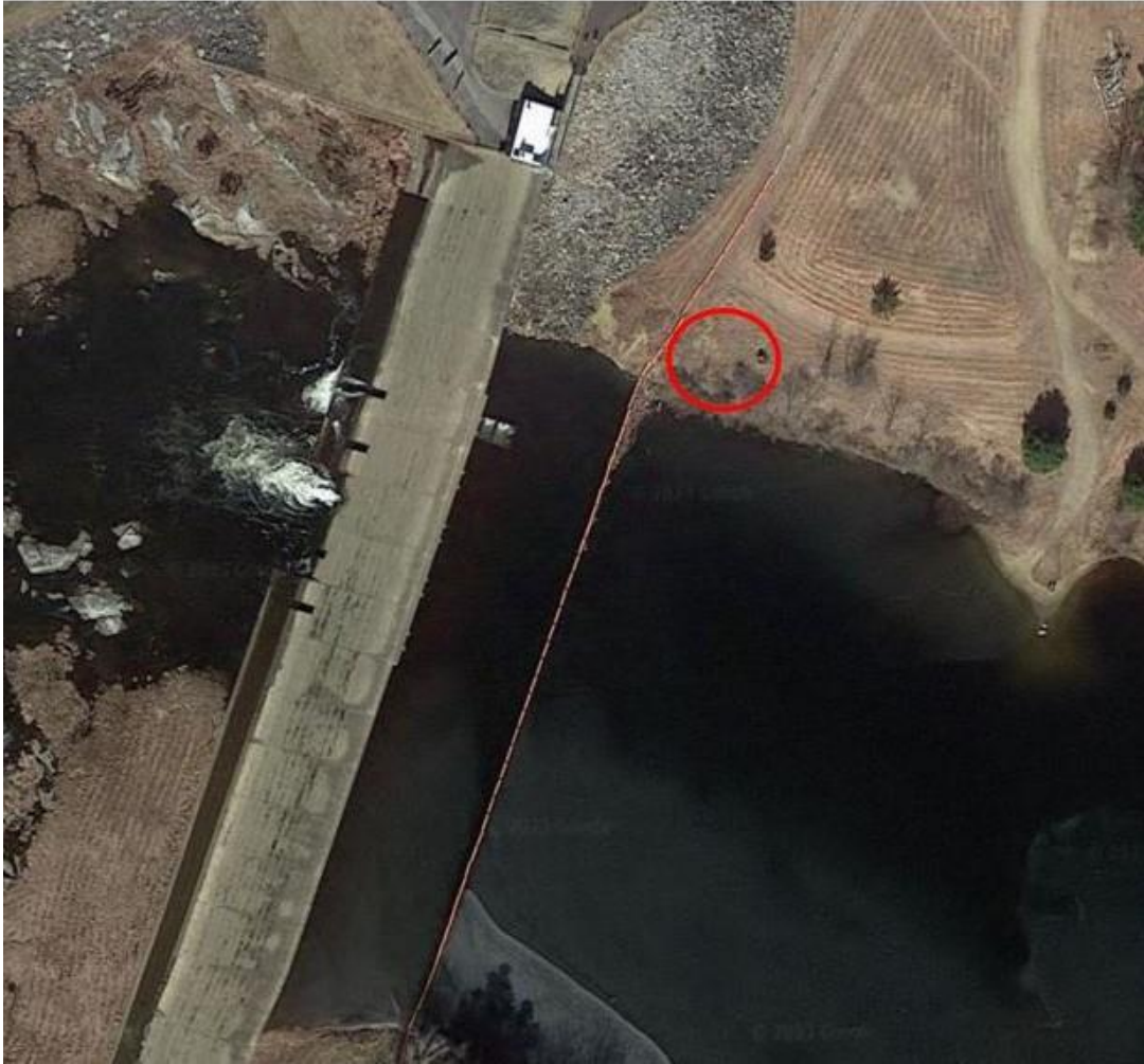
Map 3: Image showing working area where crane is proposed to be staged. 90 ft crane is recommended due to natural working pad location.
