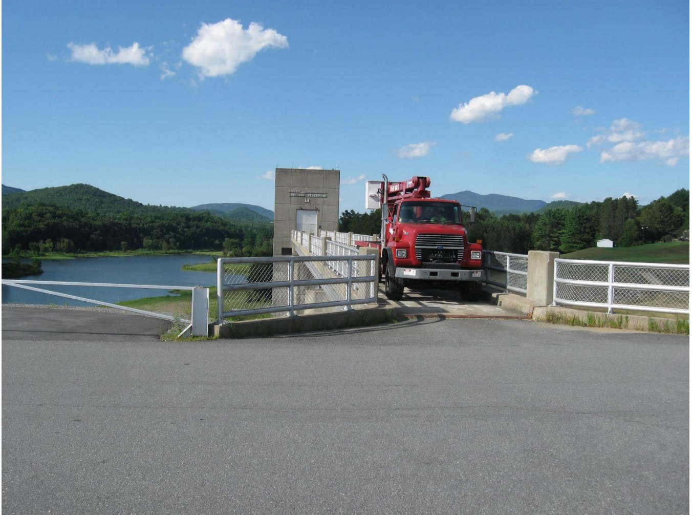
Informational Photo 5: Snooper truck on the North Springfield Lake Service Bridge
