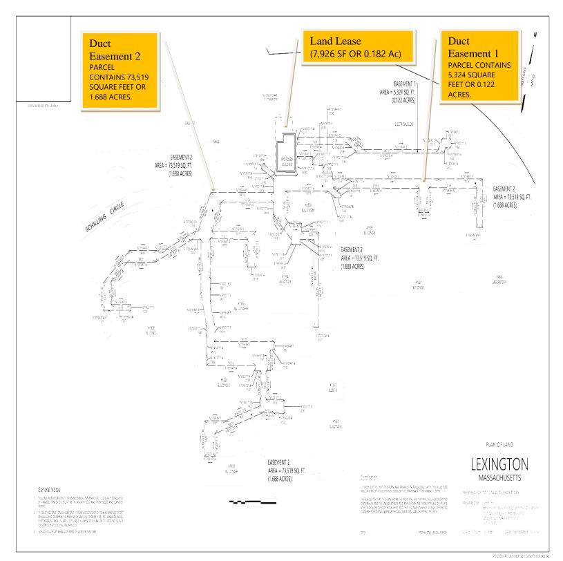
Consisting of a small site to place a single generator cluster building to be constructed on a proposed 7,926 SF (0.182 Acres) Air Force leased land on MIT LL campus. In addition, the project will require easements totaling up to 78,843 SF (1.81 Acres), to run duct banks from the new generator cluster to the existing MIT LL buildings 1302, 1310, 1320, 1321,1322, 1323,
