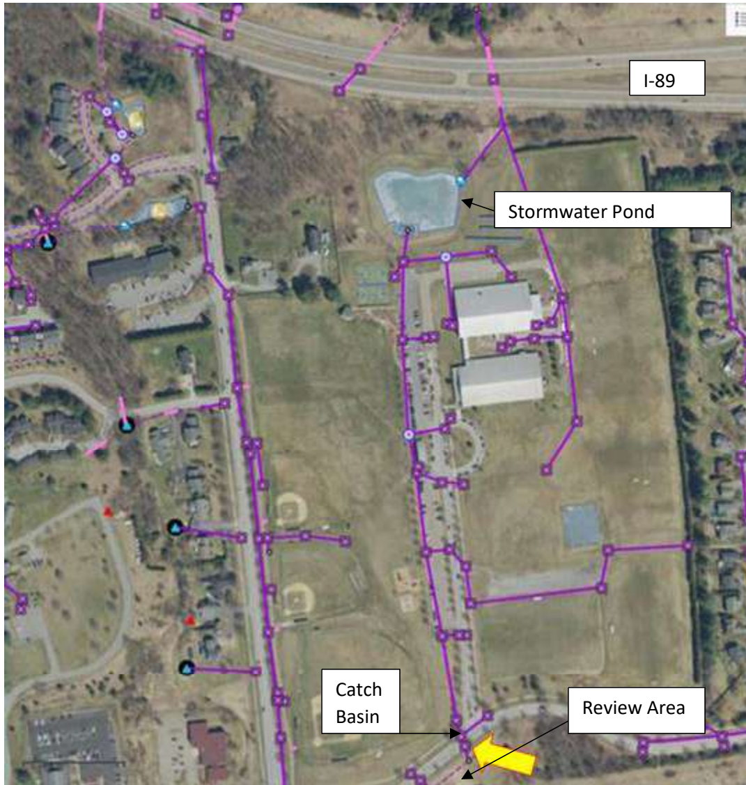
Diagram of catch basins and connecting pipes of existing stormwater treatment systems in the project vicinity provided by the City of South Burlington.
